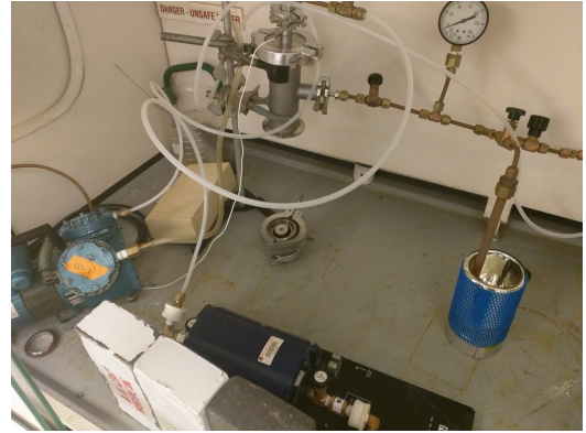
(b) The radon deposition system
