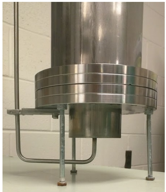
(b) The lower volume with the gas flow tube.
