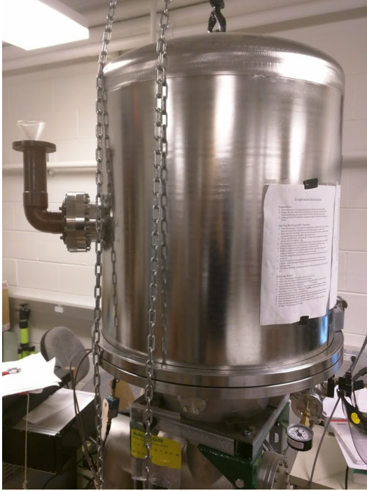
(a) The TPB vacuum deposition system.
