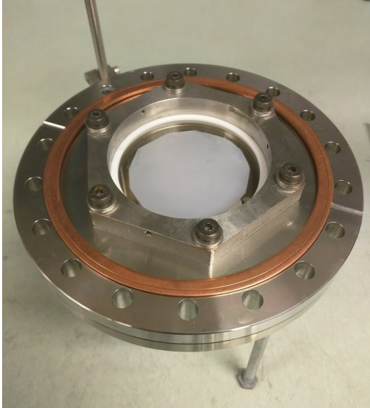
(a) The quartz window seal between the upper and lower volumes, with TPB evaporated on the surface. Some measurements used a clear window without TPB.
