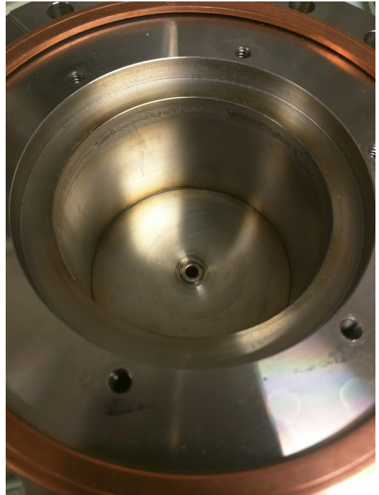
(b) The empty lower volume before the reflector and sample are placed inside.
