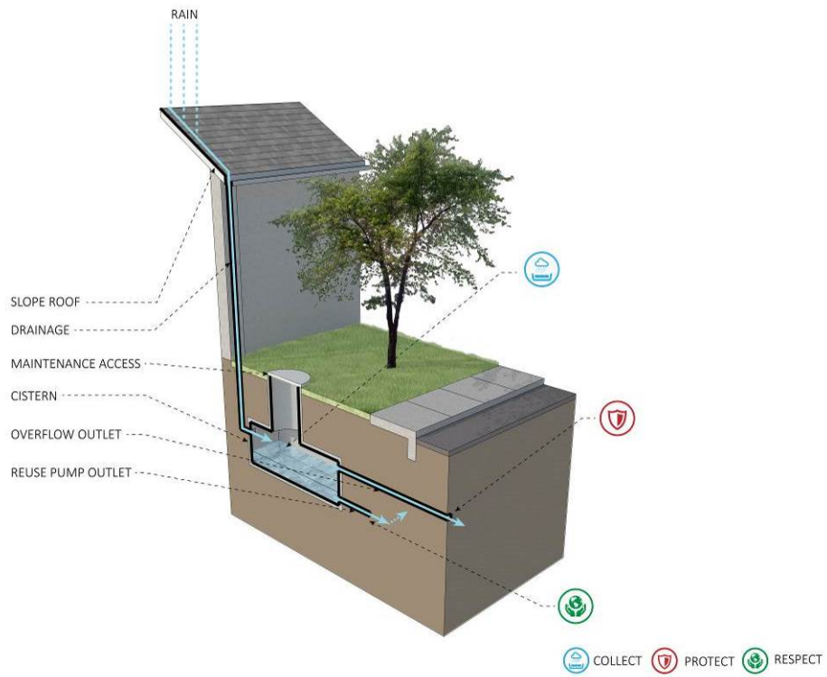
Figure 6-6: Roof Water Collection (Source: Author, Justin Manongdo)
