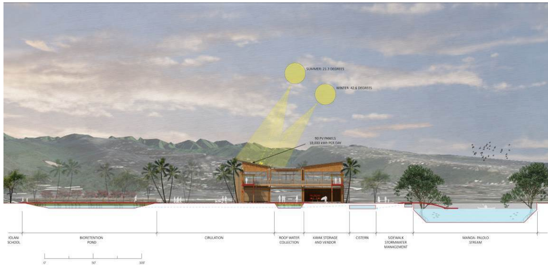
Figure 7-11: Section A-A Water Collection (Source: Author, Justin Manongdo)
