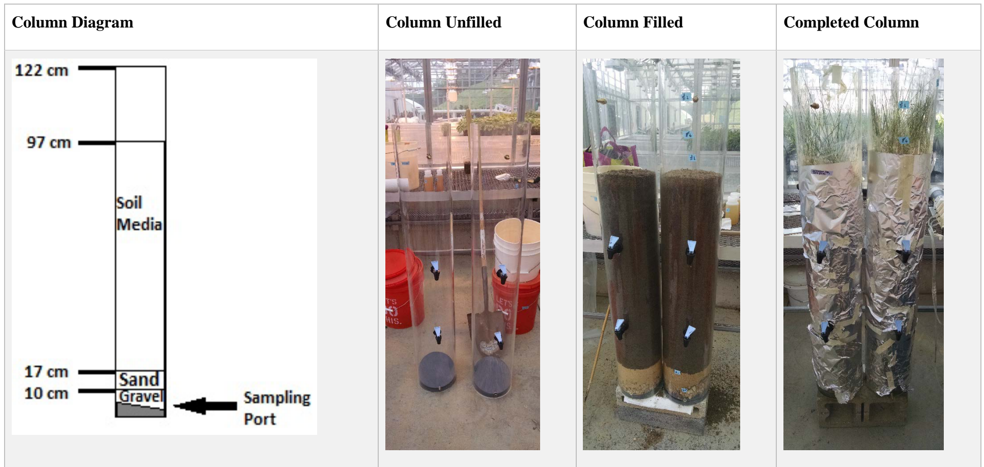
Figure 2.1: Large bioretention column setups for experimental trials.
