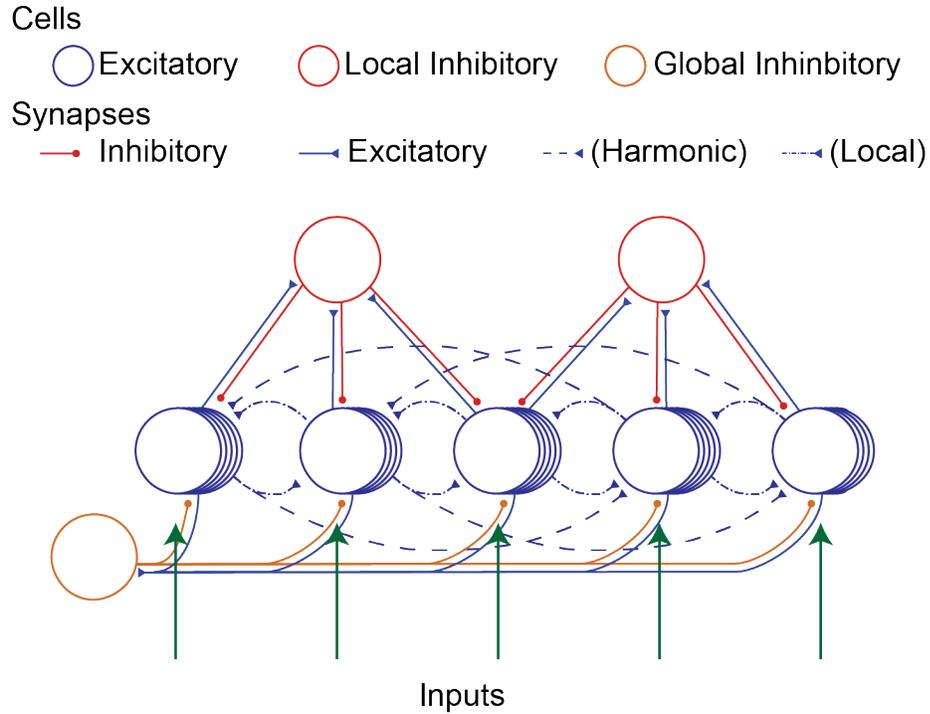
Figure 4.1: **Network structure.** Network composed of excitatory neurons, global inhibitory neurons and local inhibitory neurons. Recurrent excitatory connections change between different networks investigated.
