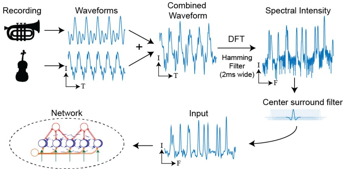
Figure 4.2: **Cochlear pre-processing.** Stages involved in pre-processing stimulus, similar to calculations performed in the cochlea. Sound waves from multiple sources are combined into a single waveform, which is then decomposed into frequency space using a discrete fourier transform (using a hamming filter 2 ms wide, phase information discarded). This is then passed through a 'Difference of Gaussians' filter to create the input current for each excitatory group of neurons.
