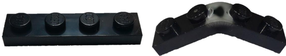
Figure 31: LEGO® brick showing color change when bent
