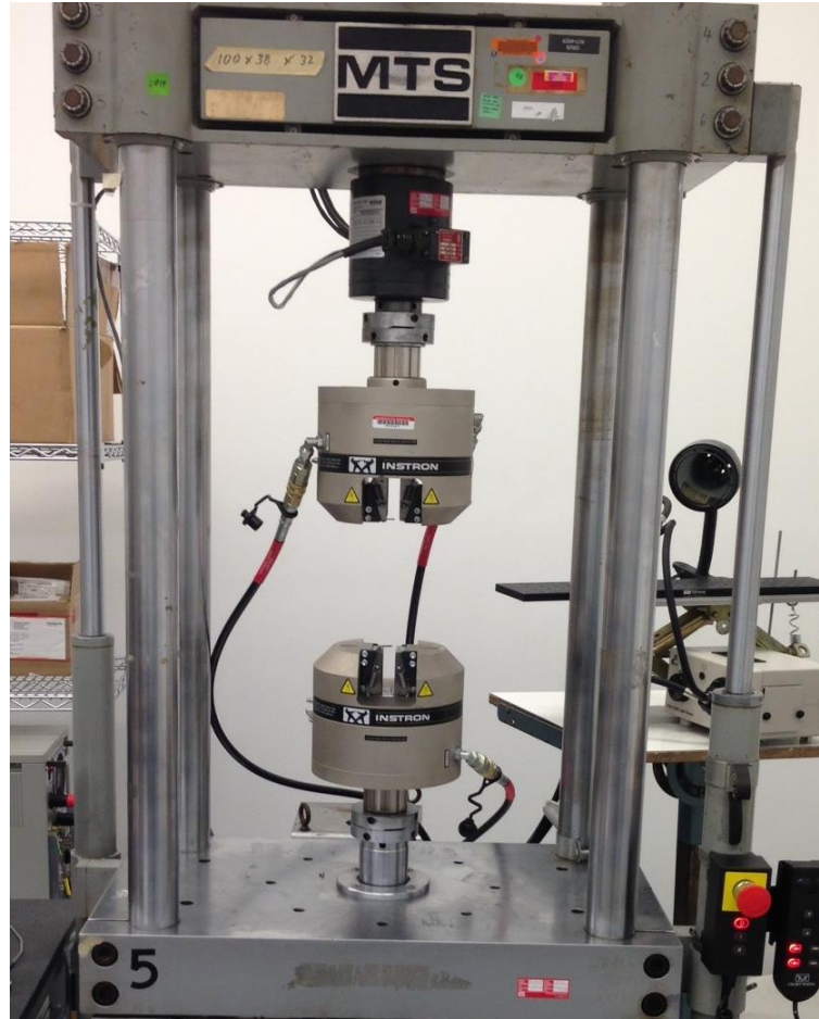
Figure 11: Servo-hydraulic MTS machine
