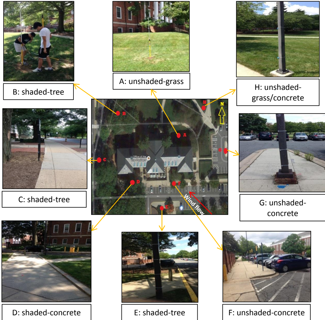
Figure 14: The location of the iButton temperature sensors in the experiment in July 2014 around Mitchell building on the University of Maryland campus
