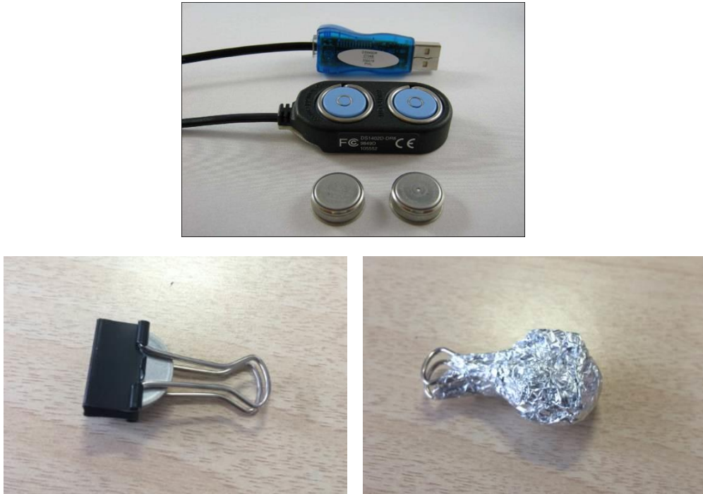
Figure 13: Preparing iButton sensors for the temperature measurements, avoiding direct sunlight and rain using some aluminum foil
