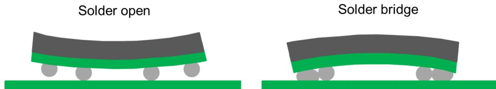
Figure 1.1 Warpage caused failure of the BGA package
