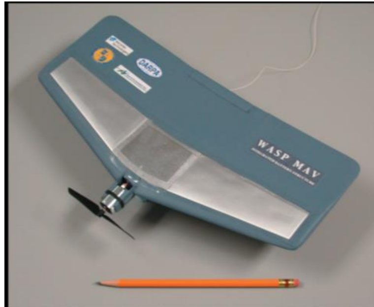
Figure 2.16: UAV with batteries integrated into the wing [19, 20]
