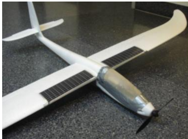
Figure 2.15: Fixed wing vehicle with vibrational harvesting capability as well as solar harvesting capability [13]
