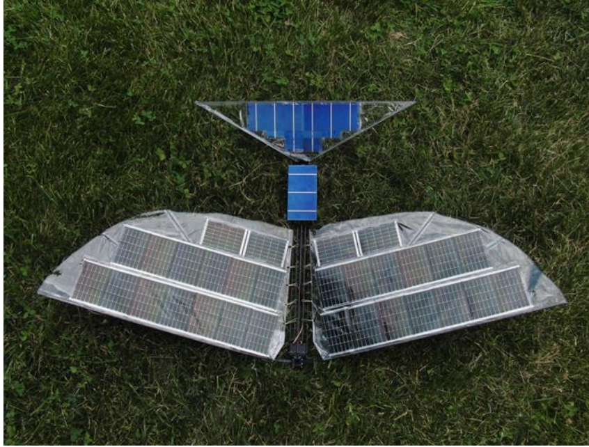
Figure 6.6: Robo Raven with polycrystalline solar cells in the tail and body, and Powerfilm flexible solar cells in the wings.
