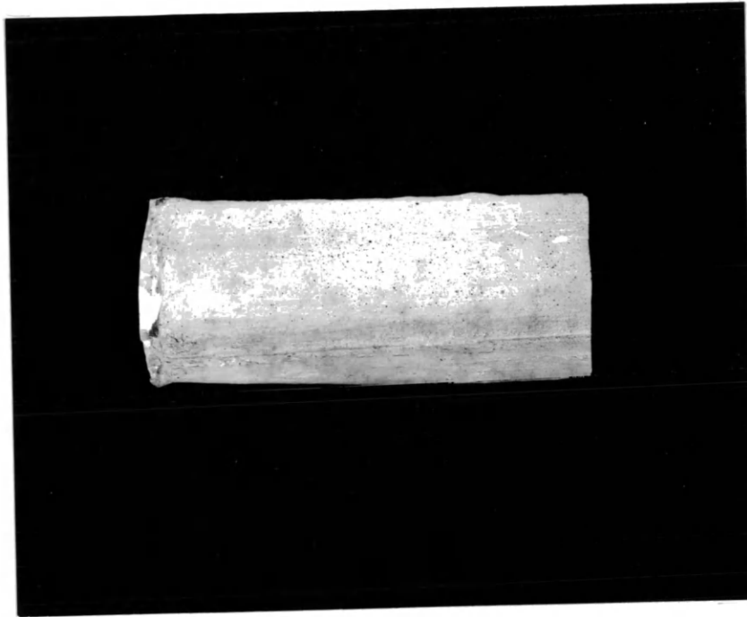
Figure 6. Unfired barium titanate tube. In this condition the tube is powdery, fragile and has a faint pink color.
