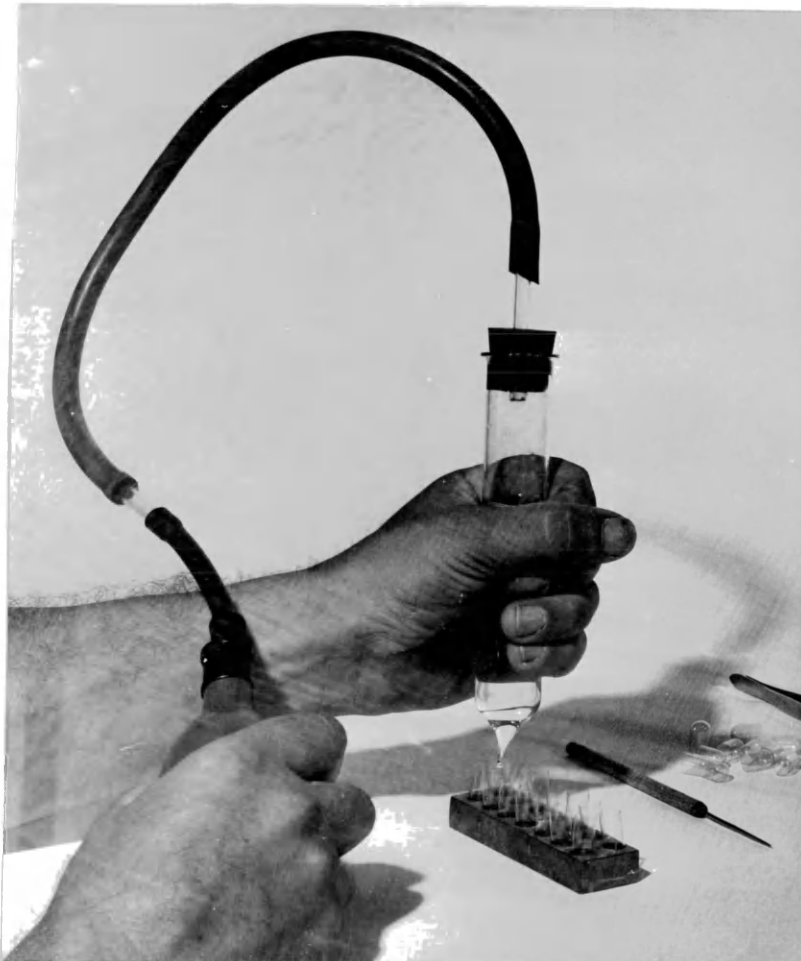
Figure 18. Dispenser for partially polymerized methacrylate. The bulb forces the liquid out through the capillary.
