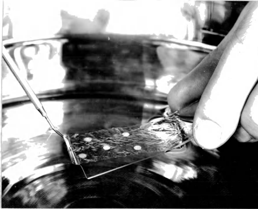
Figure 19. Stripping collodion film from the microscope slide. Note the specimen screens on the film.
