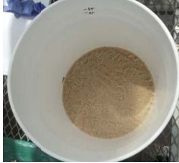
Figure 4.2 Washed pool sand was added to 2.54 cm above the bottom of the bucket
