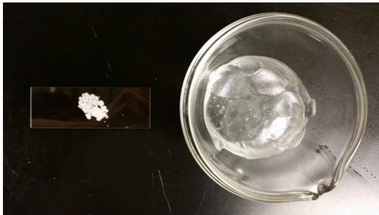
Figure 4-1. Swollen Na-polyacrylate; the right sample has swelling capacity of water 243.1 g/g.
