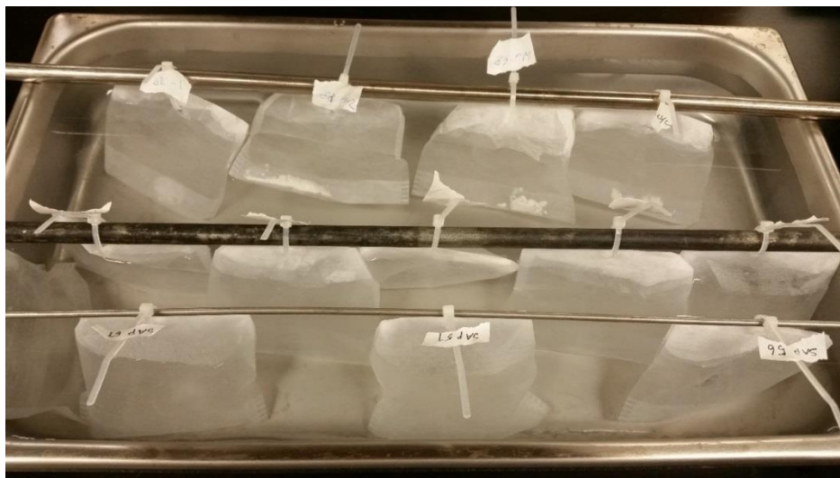
Figure 5-11. Illustration of tea bag method and an image of measuring swelling capacity by the tea bag method.
