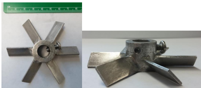
Figure 6-4. The images of the reactor and the agitator used in the experiments; 500 ml-unjacketed reactor with conical flange (I.D.: 108 mm and height: 125 mm), and turbine style agitator (D: 80 mm).
