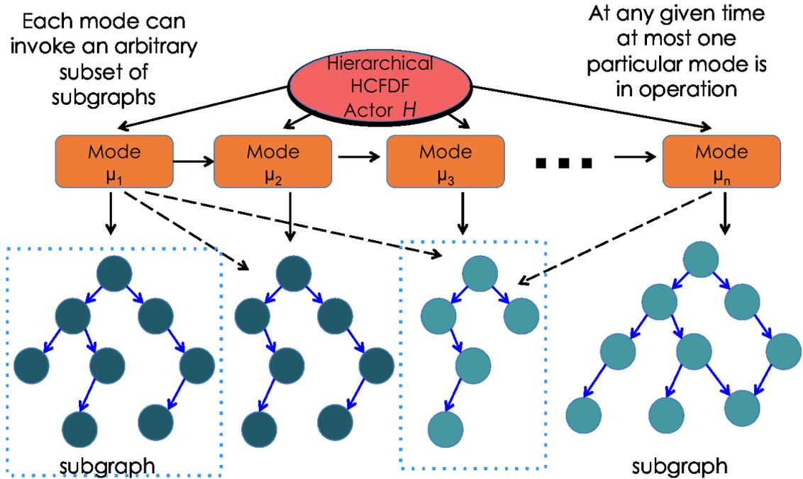
Figure 4.2: Modeling multi-mode DDDAS designs using HCFDF graphs.
