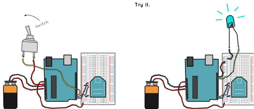
Figure 14: Drawing of the complete remote light switch.
