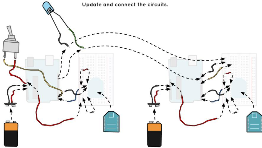
**Figure 12: Drawing of the circuit connections and component placement on the breadboard for the remote light switch.**
