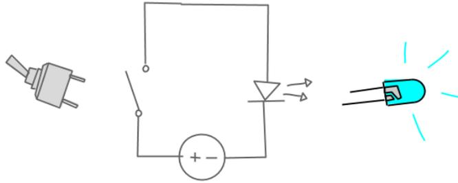
**Figure 44: Conceptual drawing of the default “switch” behavior of a module represented as a switch circuit.**
