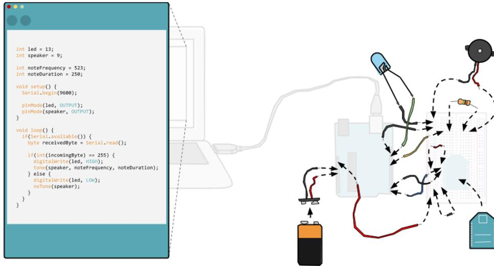
**Figure 21: Drawing of connecting an additional “Output” device. This is done for each of the three additional devices. The complete program is shown in Figure 53 (Appendix A).**
