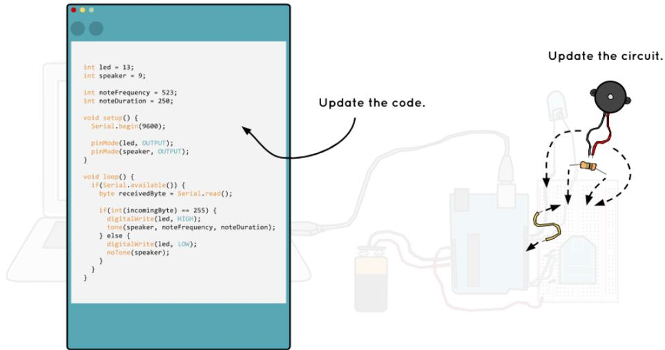
Figure 19: Drawing of connecting the speaker into the circuit and programming the circuit.
