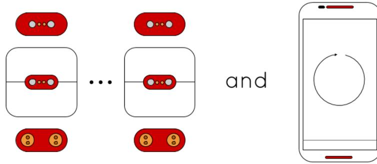
**Figure 1: Conceptual drawing of Pixel, consisting of one or more Pixels (left) and, optionally, a mobile device to program Pixel behavior with the graphical programming environment.**
