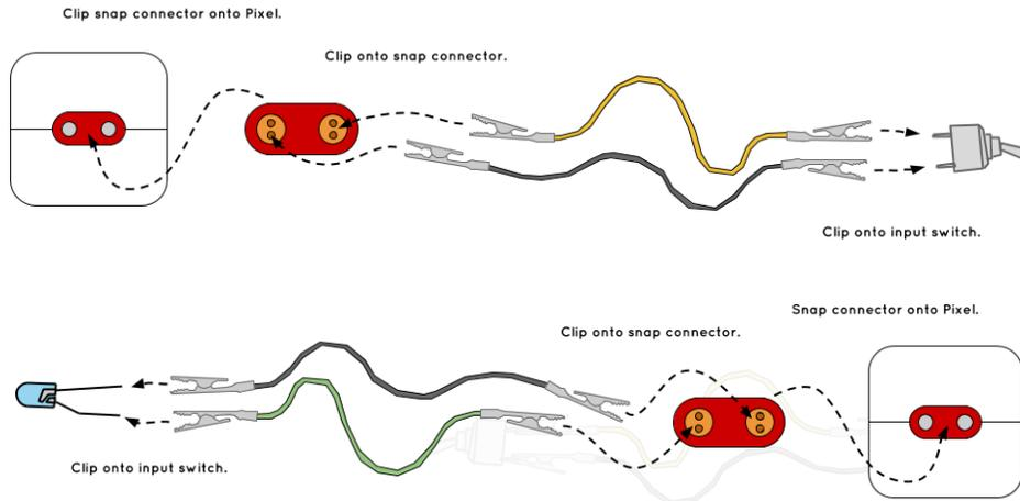
**Figure 9:** Drawing of connecting the input switch (top) and output LED (bottom) for the light switch. The complete system is shown in Figure 10.
