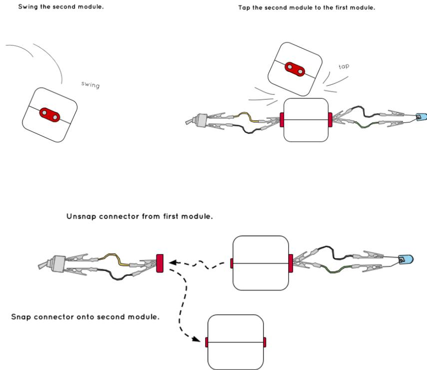
Figure 15: Drawing of the sequence of actions to adapt the light switch to be a remote light switch.
