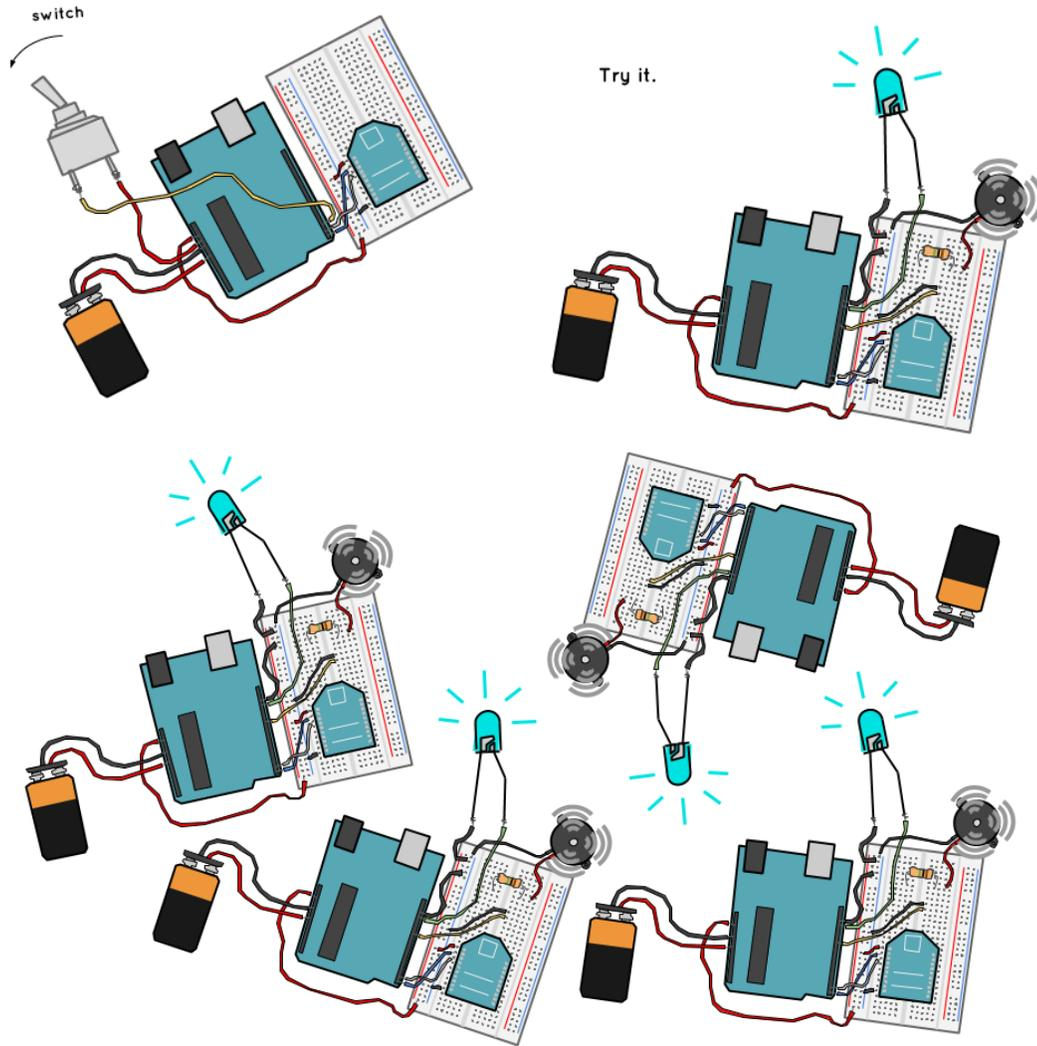
Figure 22: Drawing of connecting an additional “Output” device. This is done for each of the three additional devices.
