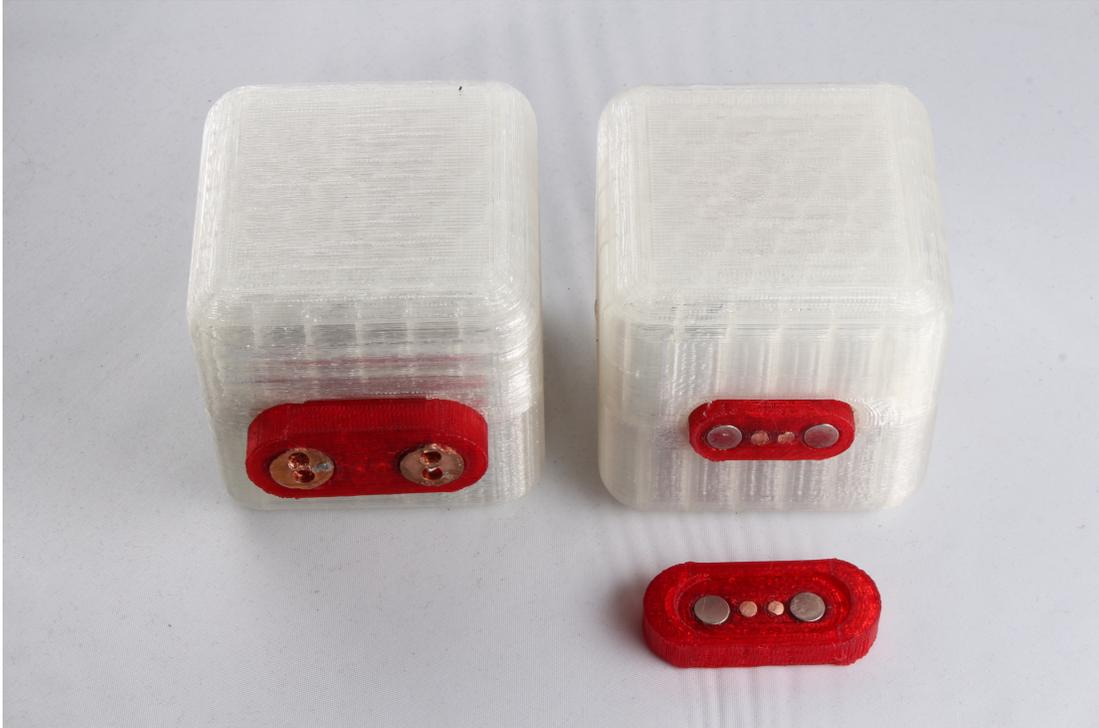
**Figure 34: Photograph of the final prototype, showing the interchangeable port adapters, both attached (left) and detached (right) from modules.**
