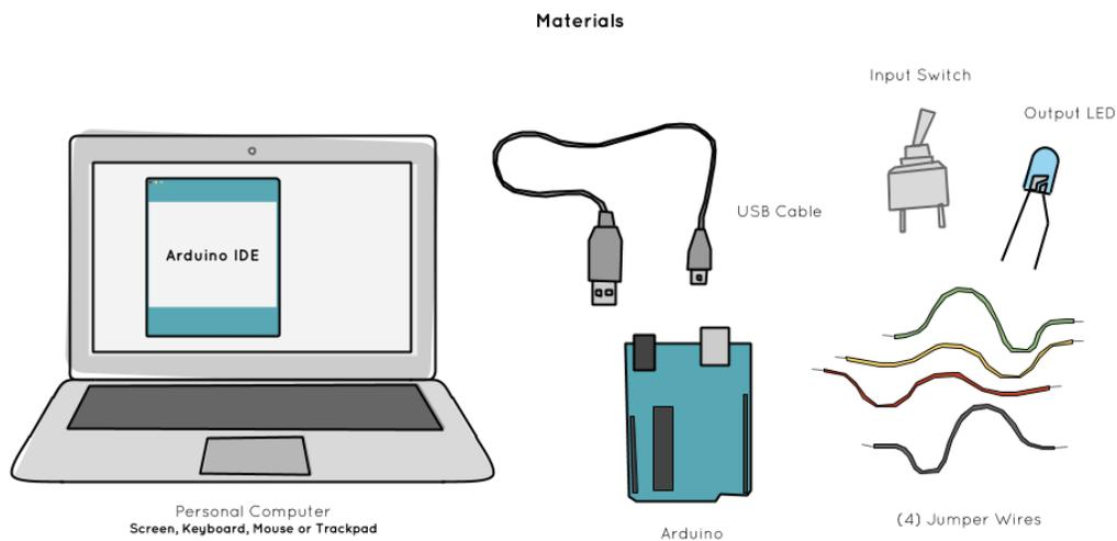
Figure 4: Illustration of the materials needed to make the light switch. Note that no current limiting resistor is used in this scenario, for simplicity.
