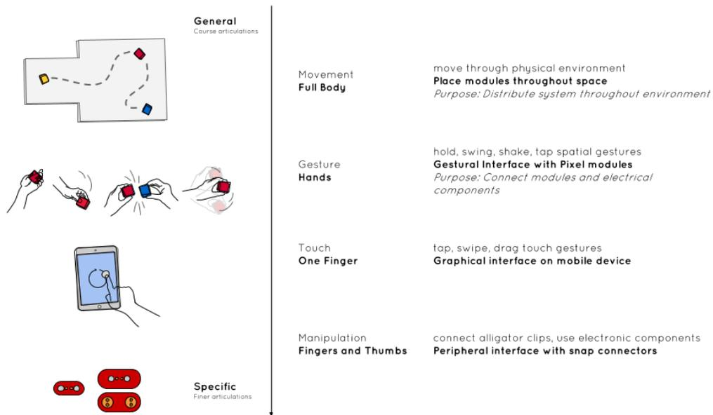
Figure 37: Drawing and description of the general relationships between the movement, gesture, touch, and manipulation engagement styles.
