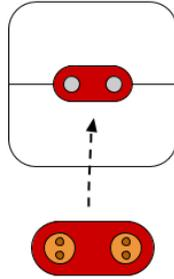
**Figure 3: Drawing of Pixel's "snap connection interface." The component on the Pixel is the "port" to which the removable "snap" couples. The port's two gray circles represent magnets that hold the snap onto the Pixel. The snap has magnets on the opposite side of that shown. The two circular copper features of the snap are designed specifically for connection with alligator clips.**
