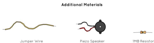
**Figure 18: Drawing of the additional materials needed to adapt the remote light switch to play sound.**
