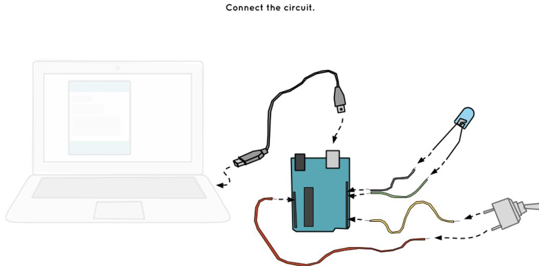
Figure 5: Drawing of connecting the components for the light switch.
