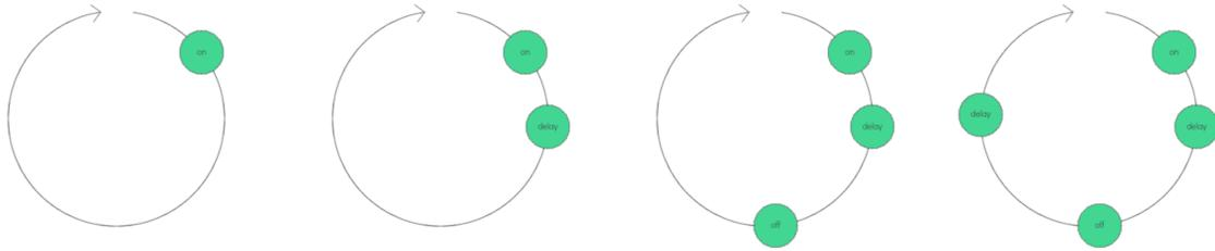
**Figure 43: Four screenshots showing a four-action sequence for turning a connected light emitting diode on for one second then off for one second. This behavior, equivalent to Arduino’s “Blink” example, was created leisurely in under ten seconds on a Motorola Moto X (2<sup>nd</sup> Generation) mobile phone using one hand.**
