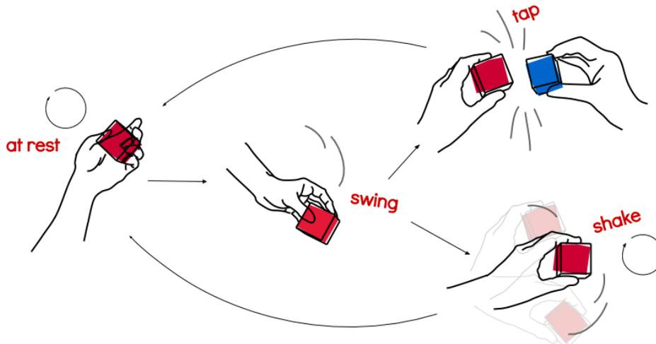
Figure 39: Drawing of the state transition diagram underlying the gestural language.
