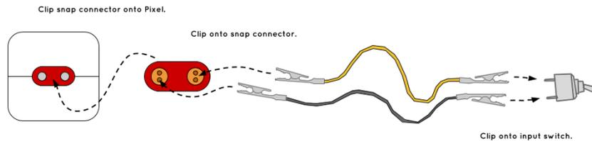
**Figure 27: Drawing of connecting the input switch to the “Switch” Pixel.**
