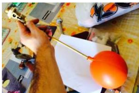
Figure 164: Float Valve (Author)
