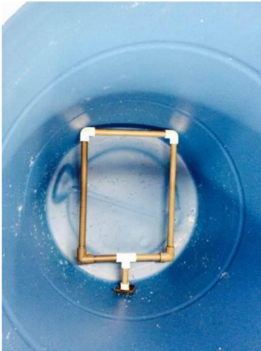
Figure 63: Underdrain Assembly Lab Testing (Author)
