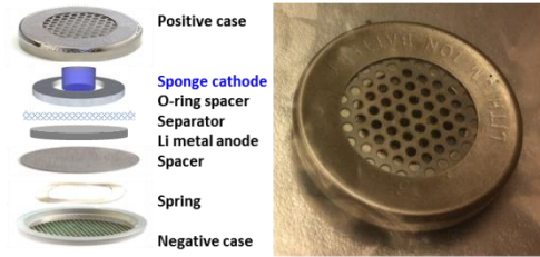
Figure 8: Specialized Li-O 2 coin cell
