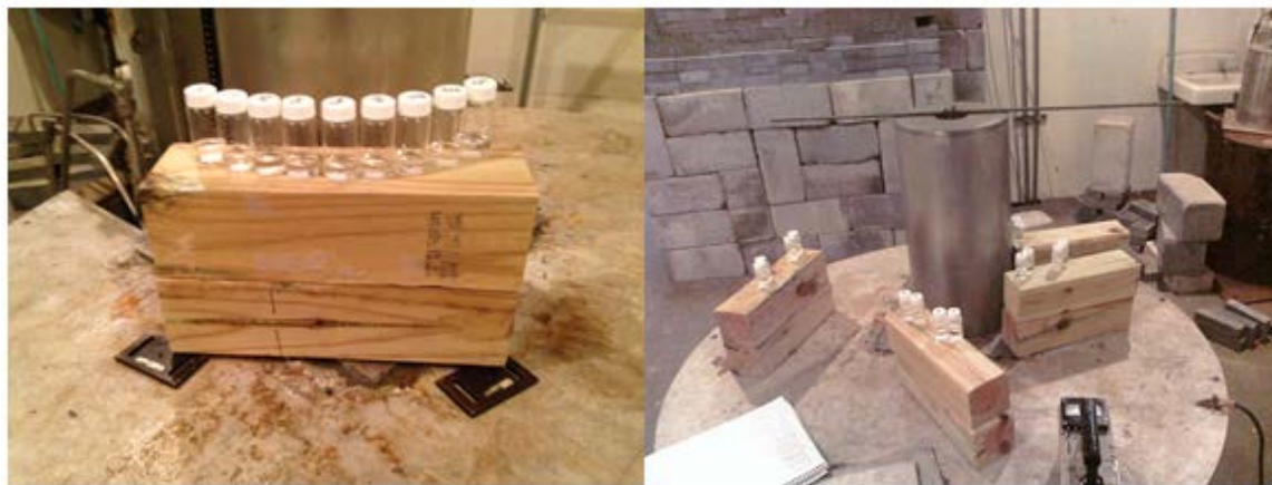
Figure 24. (Left). A set of samples prepared for direct grafting. Each sample was individually measured to be equidistant from the source top hat. (Right). An example of irradiation at 7 different dose rates simultaneously. All samples were placed at 8 inches from the working surface with a direct line-of-sight to the source.
