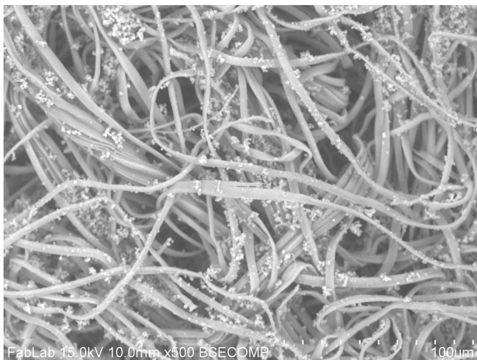
Figure 69. Winged nylon fabric grafted to 53% with B2MP in ethanol. Irradiation with Co-60 at 10 kGy/hr to 40 kGy total dose. 500x magnification; 15 kV.
