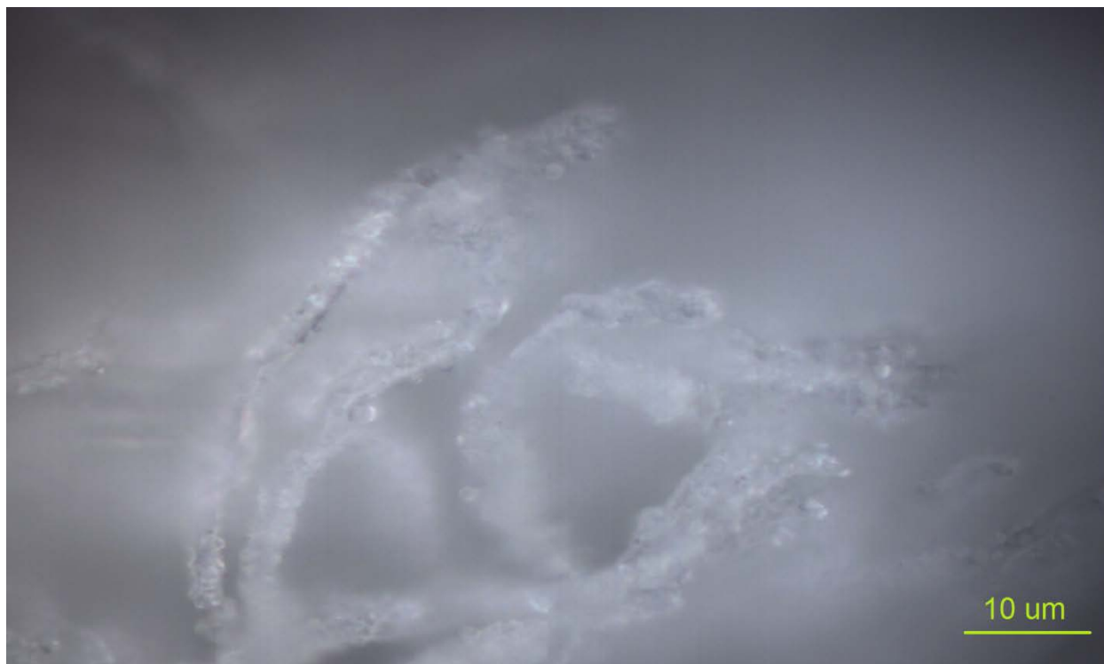
Figure 63. Optical micrographs taken with the confocal Raman microscope of B2MP grafted onto Winged nylon to 50.3% in ethanol. 50x objective, scale approximate
