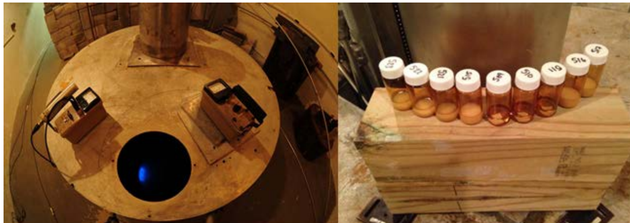
Figure 13. The working surface where small samples are positioned for intermediate-to-high dose rates. Right: An typical high-dose-rate irradiation. The vials are placed at 8 inches vertically from the pool cover and 3 inches radially from the source top hat to receive 10 kGy/hr.
