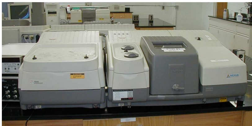
Figure 17. Thermo Nicolet NEXUS 670 FTIR. Chemistry department at the University of Maryland [339]
