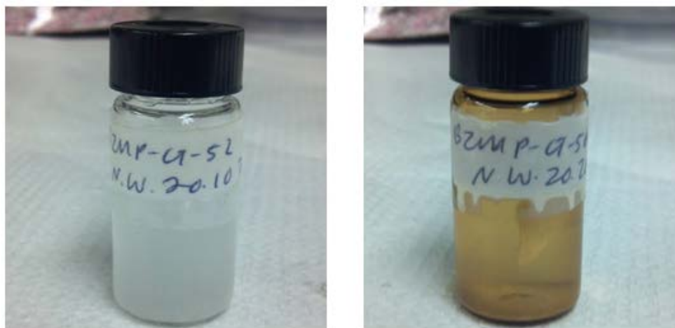
Figure 31. (Left). Un-irradiated vial containing 0.093 M B2MP in water after approximately 115 minutes of sonication. The solution is cloudy and precipitate is already beginning to accumulate on the vial bottom. (Right). Vial containing 0.093 M B2MP in water after irradiation Co-60 at 20 kGy/hr for one hour. Note that the solution is clearer and several mm of precipitate has accumulated at the bottom. The grafted polymer sample is floating near the surface. The darkening of the vial is due to discoloration of the glass upon irradiation.
