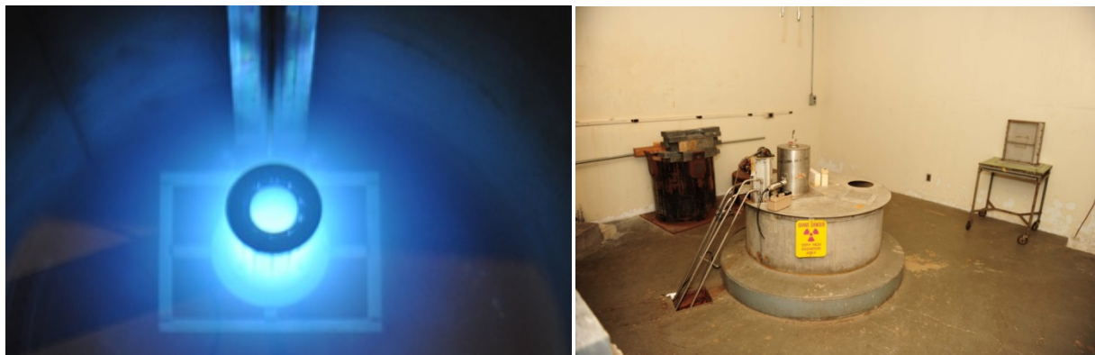
Figure 12. (Left): The Co-60 source array of highest activity in the shielded position. The array consists of ten doubly-encapsulated stainless steel pencils mounted on a movable source rack. (Right): The irradiator vault. In the center is the top of the water-filled storage pool. The elevator mechanism and source top hat are also shown in the center of the photo
