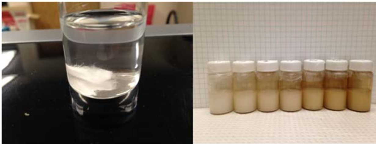
Figure 32. (Left) Typical sample for direct grafting composed of B2MP, ethanol and un-grafted nylon awaiting irradiation with Co-60. Notice the position of the fabric at the bottom of the vial. (Right) Vials containing a single fabric (~25.4 mg) immersed in B2MP dissolved in 10 mL ethanol. Photo taken after direct grafting with Co-60 at 10 kGy/hr to 1, 2, 6, 12, 20, 30 and 40 kGy (left to right). The increase in viscosity of the solution is visible with increasing dose.
