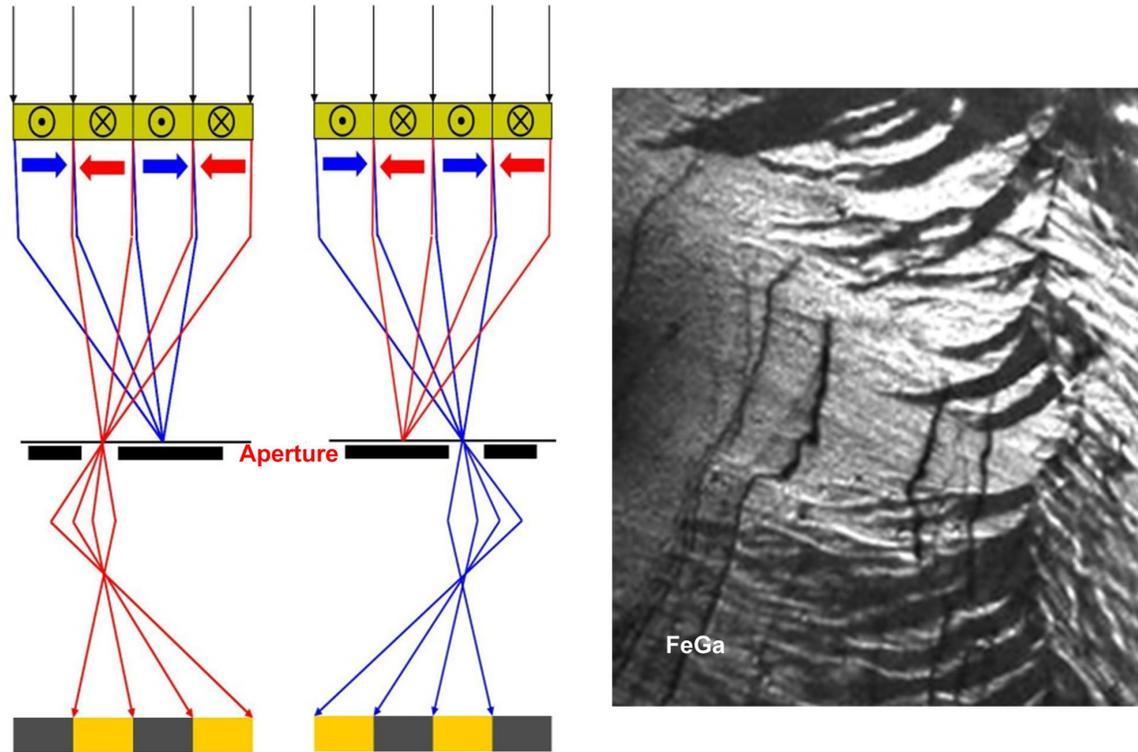
**Figure 3-15.** Schematic of TEM electron-optics for Foucault contrast. An aperture in the back focal plane serves as a knife-edge to select or block specific domain deflections. The result is dark field contrast of a magnetic domain, as seen in the FeGa thin film. Adapted from [75].
