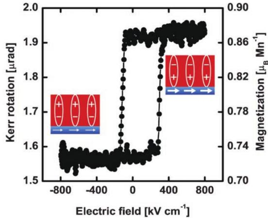
**Figure 2-23. M–E hysteresis curve showing the magnetic response of the PZT/LSMO heterostructure at 100 K as a function of the applied electric field, measured by a MOKE magnetometer. Insets represent the magnetic and electric states in the LSMO layer (blue) and PZT layer (red). Taken from [55].**
