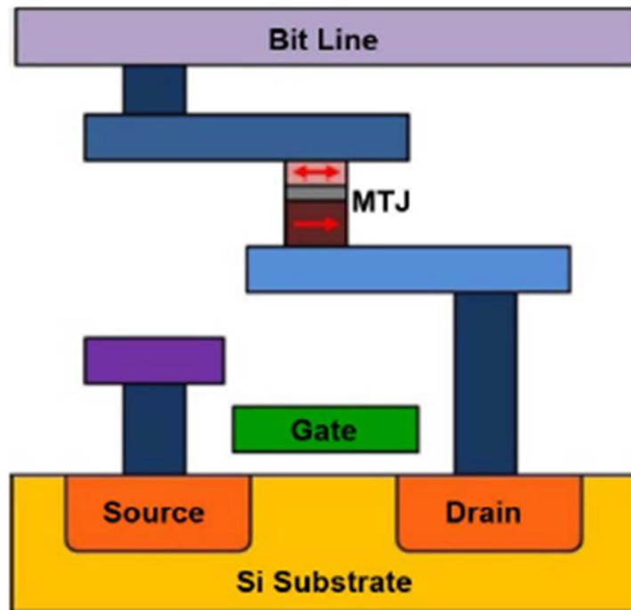
Figure 2-19. Bit cell structure of STT-MRAM. Taken from [37].
