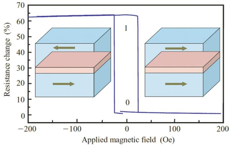
**Figure 2-18. MTJ device switching. Taken from [38].**
