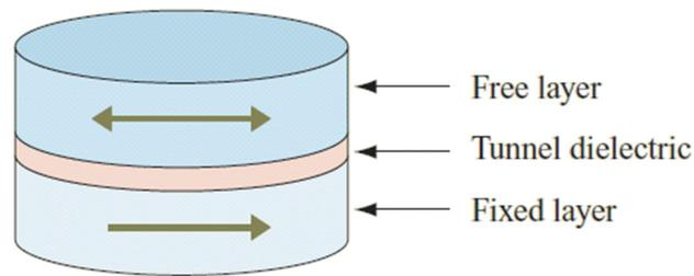
**Figure 2-17. Illustration of fundamental MTJ device structure, with indicated directions of layer magnetization. Taken from [38].**
