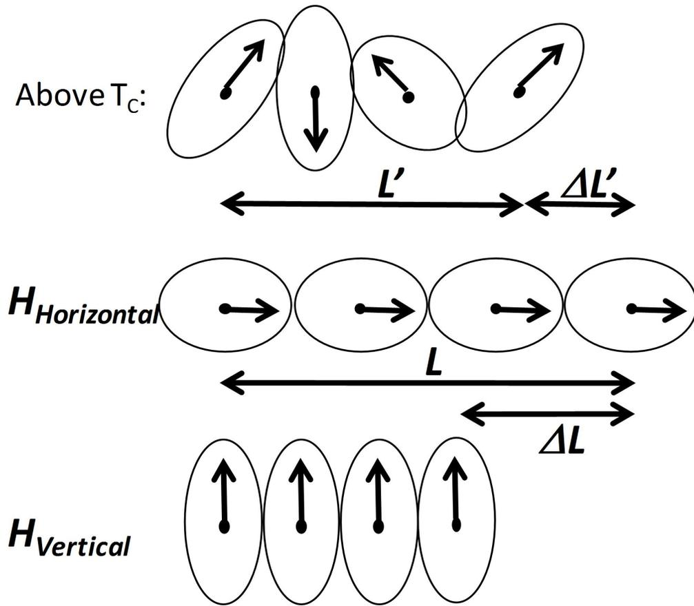
Figure 3-2. Mechanism of magnetostriction. Adapted from [27].
