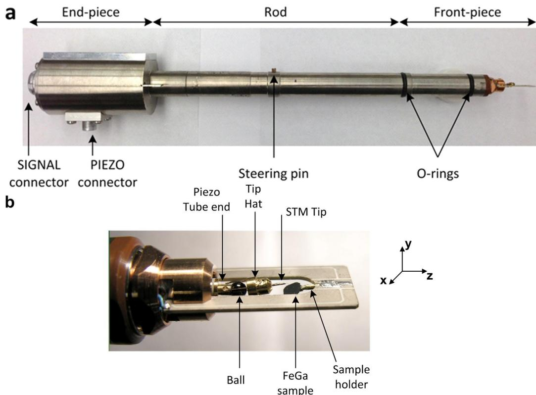
**Figure 3-8. (a) NanoFactory™ TEM-STM holder. (b) Close up front-piece constituents. The only moving part is the tip hat. The STM tip is maneuvered to the film through short pulses of the piezoelectric rod.**
