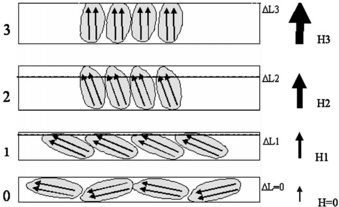
Figure 3-1. Schematic of magnetostriction of a crystal. Taken from [60].
