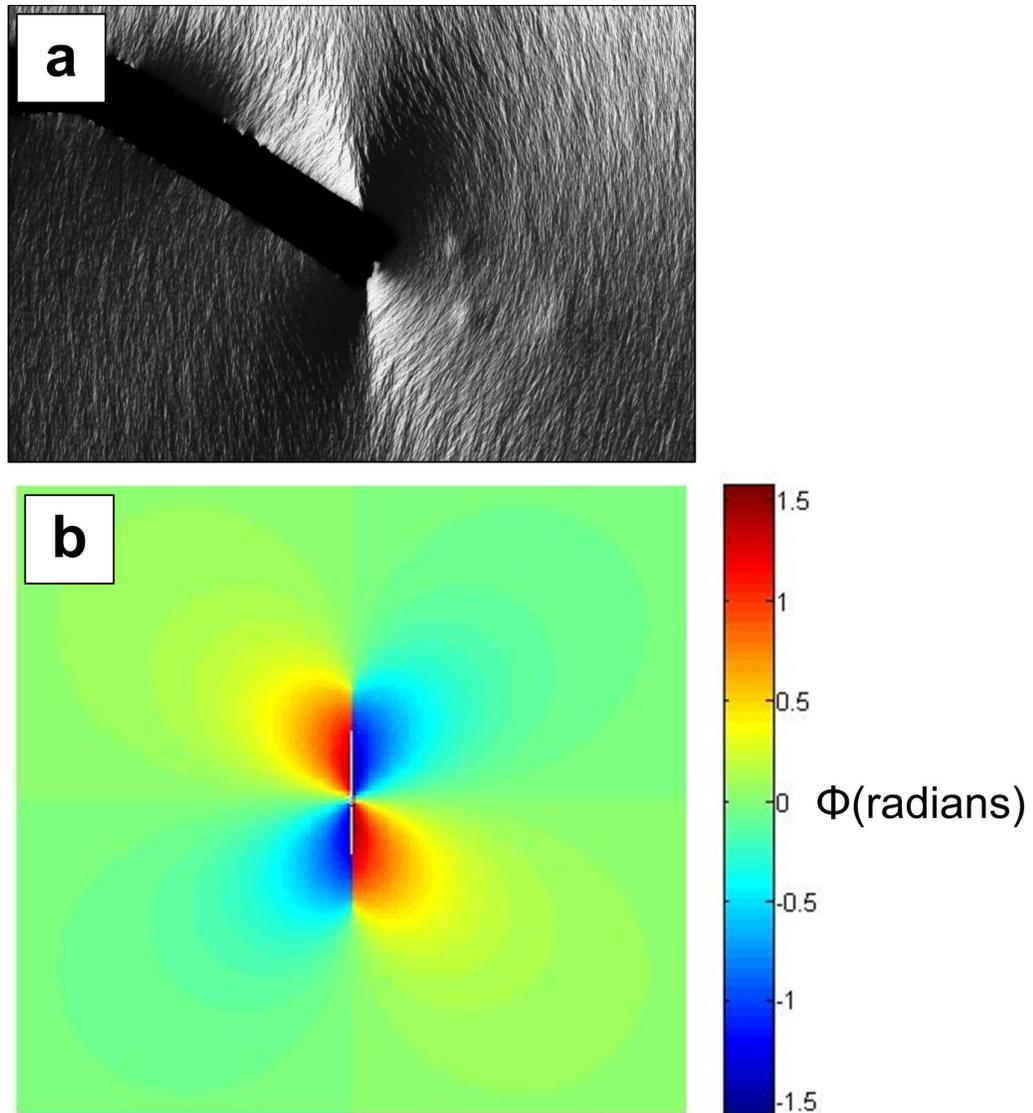
**Figure 4-9. (a) Foucault magnetic contrast of a mechanically loaded field simultaneously experiencing applied field. An aperture in the back-focal plane obscures deflections induced by specific domains. This provides contrast of magnetic domains. (b) A heuristic model of  $\phi(\vec{r})$ , where the applied stress contributing to the magnetoelastic energy is assumed to take the form  $\sigma(\vec{r}) = 1/r$ .**
