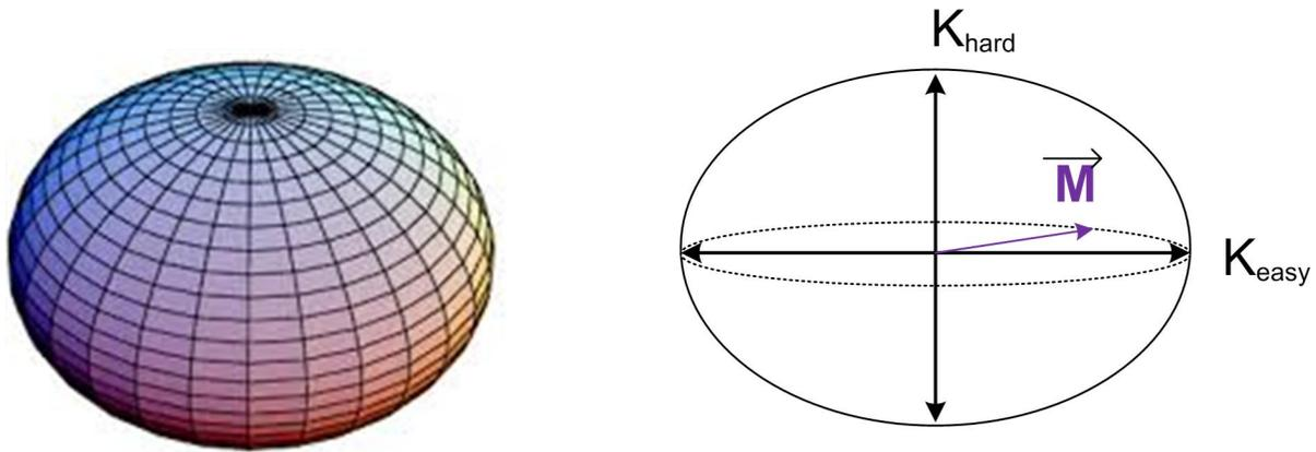
**FIGURE 4-8.** “Energy surface” representing the uniaxial anisotropy for a polycrystalline thin film. The axes of the oblate spheroid describe the hard and easy axes of magnetic anisotropy, where the larger axis represents the preferred alignment for magnetization. Thus the uniaxial anisotropy for a thin film generally lies in-plane, and thus magnetization is restricted to this dimensionality.
