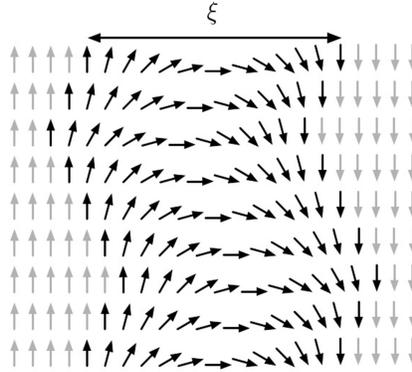
**Figure 2-7 Domains are separated by a transition region with thickness  $\xi$ . The direction of the magnetization changes gradually. Taken from [24].**
