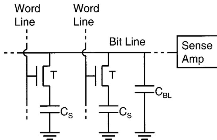
**Figure 2-4 DRAM circuit schematic. Two 1T1C cells are depicted. Taken from [19].**
