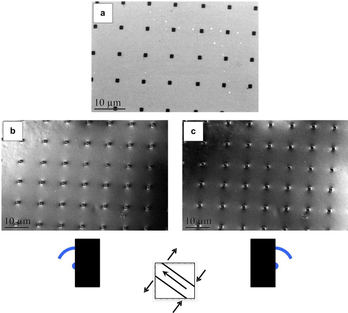
**Figure 3-19.** (a) TEM of patterned FeGa array of  $500\text{ nm} \times 500\text{ nm}$  squares using electron lithography. (b)-(c) Foucault magnetic contrast of the array captures the magnetic order within each element, and is schematically depicted. The contrast along the geometry border is due to the strong edge field. The contrast is simply reversed in these images with repositioning the edge of the back focal plane aperture.
