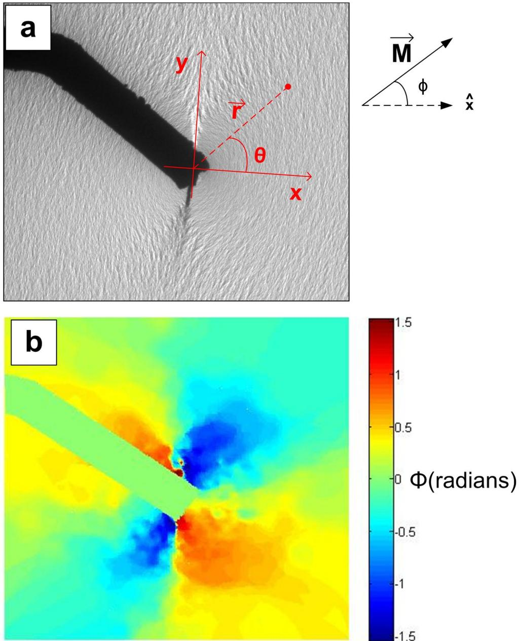
Figure 4-7. (a) Fresnel contrast of FeGa film experiencing both mechanical loading and applied field. The magnetization  $\vec{M}(\vec{r})$  is characterized by the rotation  $\phi$  away from the direction of the field generated uniaxial anisotropy. (b)  $\phi(\vec{r})$  is manually measured from the ripple texture, which lies orthogonally to  $\vec{M}(\vec{r})$ . The magnetic domains are thus characterized by  $\phi(\vec{r})$ .
