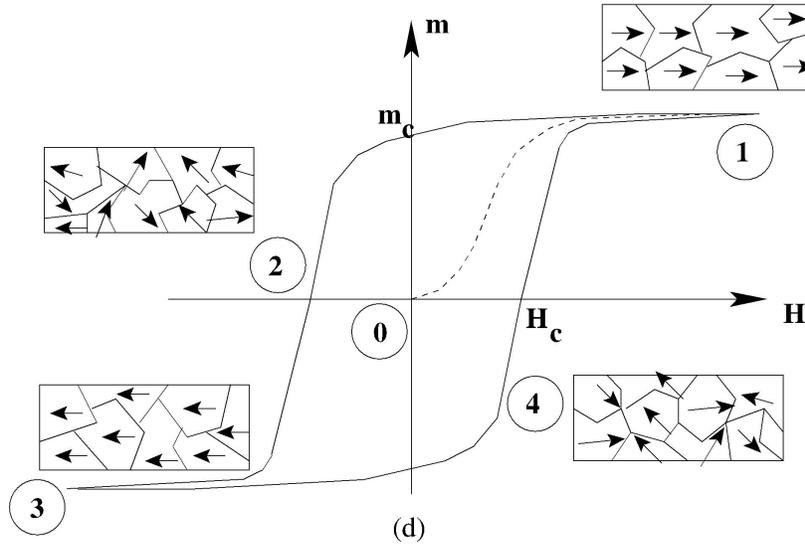
Figure 2-9. Magnetization reversal and hysteresis for a polycrystalline magnet. Taken from [25].
