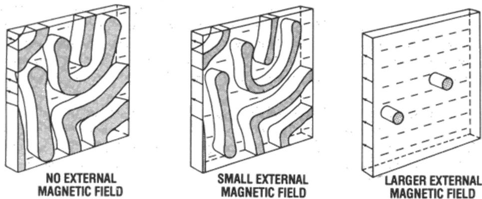
**Figure 2-10 Bubble formation within a MBM chip. Taken from [28].**
