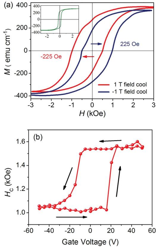
**Figure 2-24. (a) Magnetic hysteresis curves of the BFO/LSMO heterostructure measured by SQUID at 7 K after being field cooled from 350 K in 1 T (red) and in -1 T (blue). The inset shows magnetic hysteresis curve for a BFO/STO/LSMO structure with no exchange bias after field cooling. (b) Change of magnetic coercivity  $H_c$  of the LSMO with respect to the applied gate voltage at 5.5 K. Taken from [56].**
