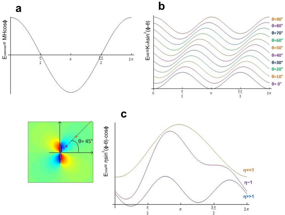
**Figure 4-10.** The “energy landscapes” of both competing energy terms (a) applied (Zeeman) field, (b) magnetoelastic energy, and (c) the combined effects. In (b) the phase of the magnetoelastic energy shifts with increasing  $\theta$ , thus magnetization rotation angle  $\phi$  shifts from  $n\pi$  to  $(2n-1)\pi/2$ . In (c) the energy landscapes represent fixed  $\theta=45^\circ$ , and the ratio of the anisotropies  $\eta$  is varied.
