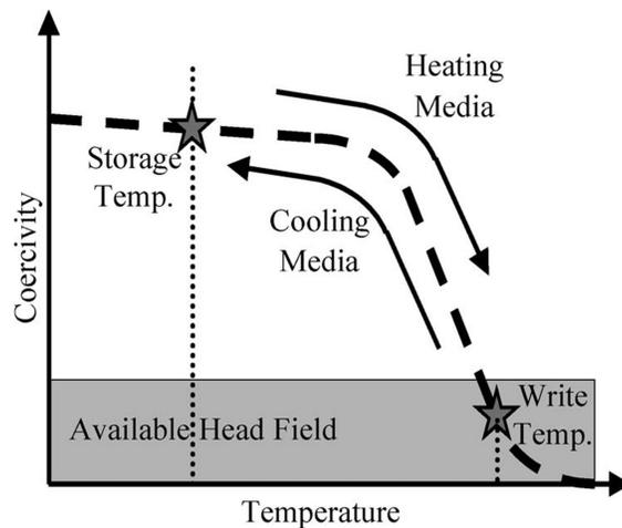
**Figure 2-15** Diagram of the HAMR write process. Taken from [35].
