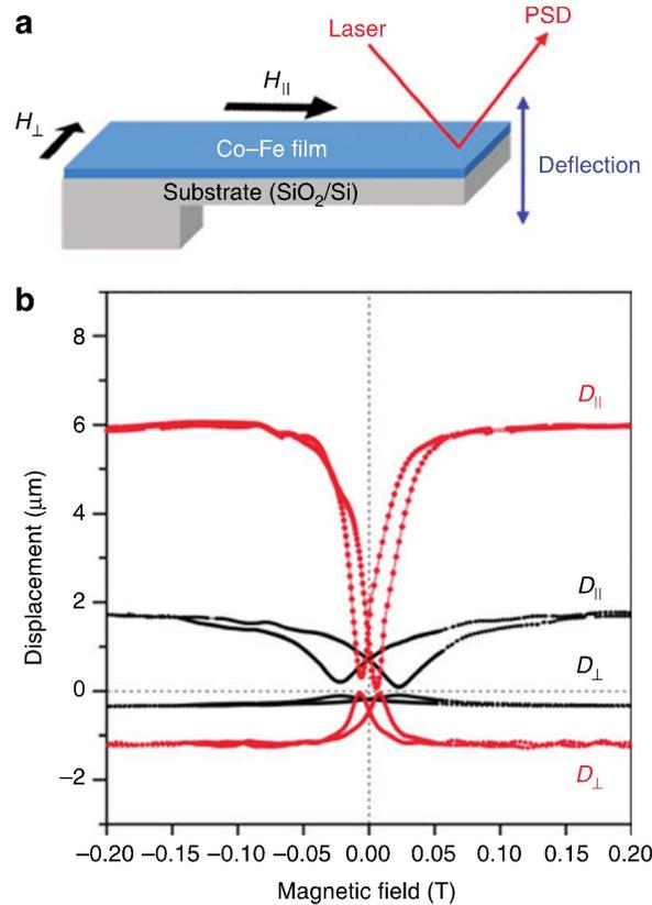
**Figure 3-6. (a) Schematic showing cantilever deflection method for measuring  $\lambda$ . (b) Plot of displacement versus magnetic field for as deposited (black curve) and annealed (red curve) CoFe. This represents an example of how the figure of merit is determined for the  $\text{Fe}_{0.7}\text{Ga}_{0.30}$  film. Taken from [72].**
