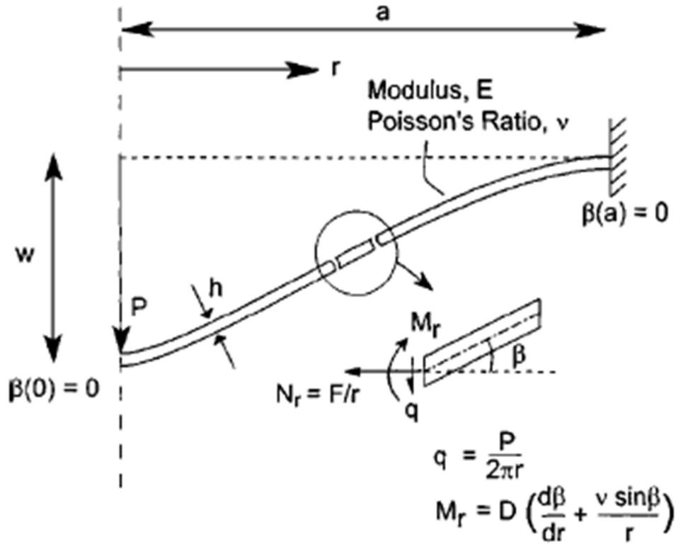
Figure 4-11. Schematic illustration of the dimensions and variables used in the analysis of a thin circular film subjected to a point load. Taken from [85].
