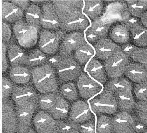
**Figure 2-13. Illustration of grains in polycrystalline magnetic recording media. Both the randomness of the easy-axis orientations, and the bit boundary are depicted. Taken from [32].**
