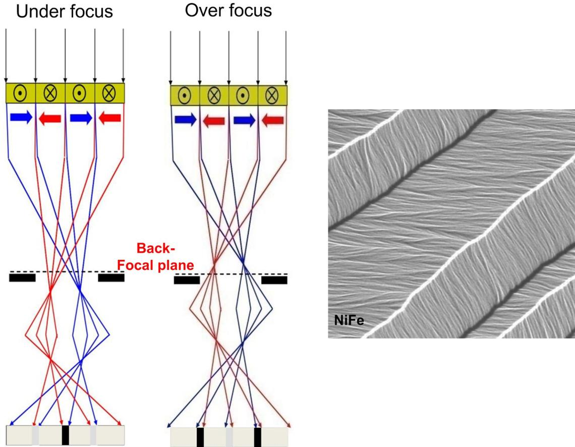
**Figure 3-13. Schematic of TEM electron-optics for Fresnel contrast. The bright/dark lines correspond to domain walls in the permalloy sample. Adapted from [75].**
