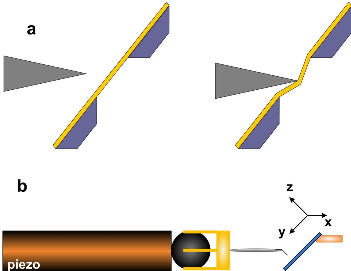
**Figure 3-7. (a) Schematic of mechanism for direct mechanical interaction with FeGa thin film. (b) Schematic of NanoFactory™ TEM-STM holder for in situ manipulation and observation.**
