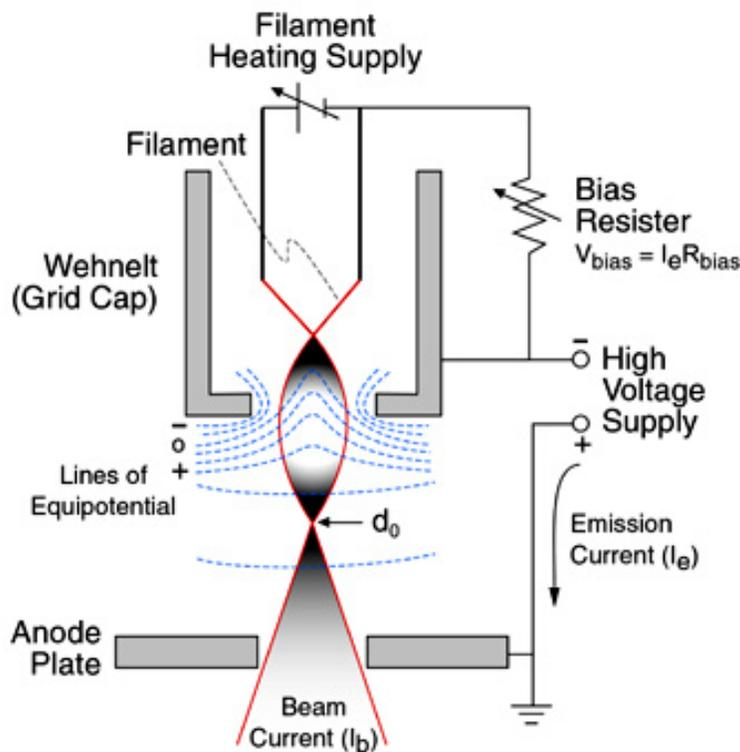
**Figure 3-10.** Schematic of a thermionic electron gun. Taken from [74].
