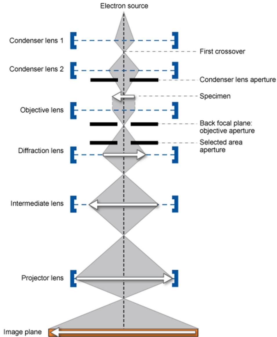
**Figure 3-9. Schematic of electron-optical system for TEM. Adapted from [74].**
