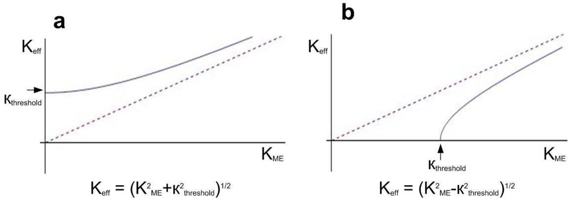
**Figure 4-14. Functional forms representing a threshold for anisotropy onset. (a) the practice of adding unassociated terms in quadrature is common, however it does not describe the sudden onset of magnetoelastic effects in the system. (b) Rather subtracting in quadrature creates a threshold barrier where magnetoelastic effects are realized. The dashed line represents a linear relationship between the effective and magnetoelastic anisotropies.**
