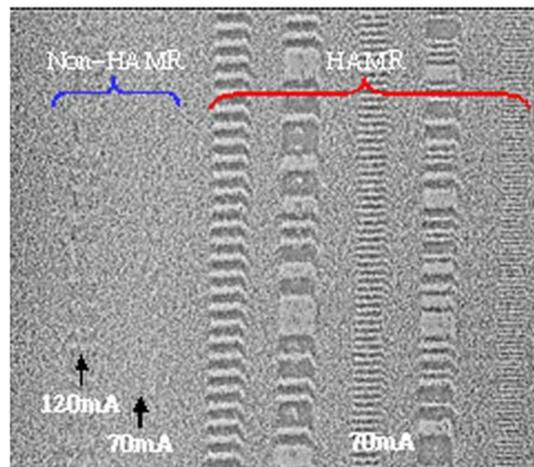
**Figure 2-16. Magnetic force microscopy image of high coercivity media being written without and with heat assist. Taken from [35].**
