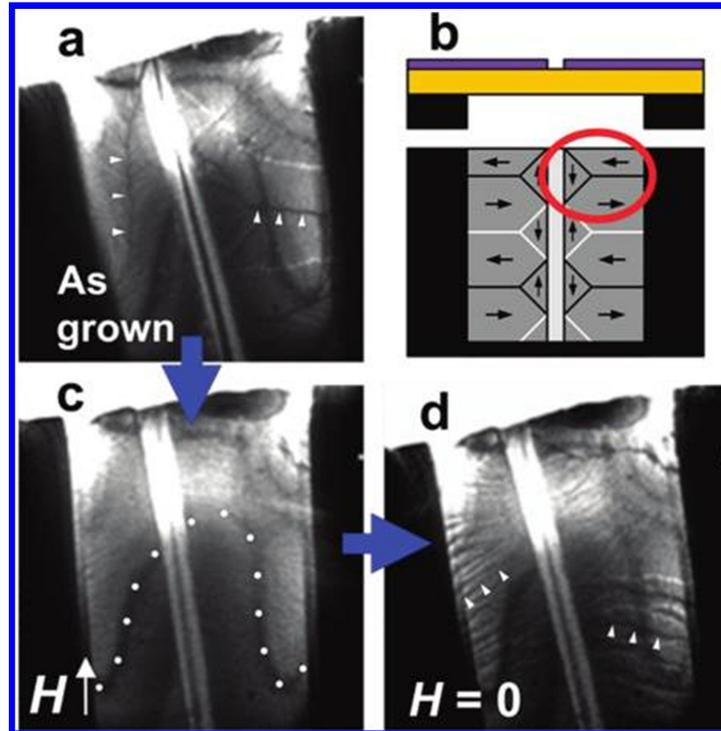
**Figure 2-27.** Magnetic response of thin film bilayer device. (a),(c) and (d) represent Lorentz micrographs of the device with magnetic fields applied. Blue arrows indicate the order of operations. (b) A schematic of the device in side-view (top) and plane-view (bottom). A schematic of the resulting magnetic order is depicted in the plane-view as light and dark lines representing domain walls, and arrows representing magnetization. Taken from [59].
