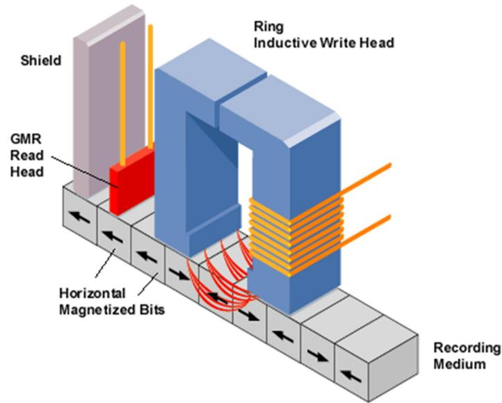
Figure 2-12 Writing process in longitudinal recording [31].
