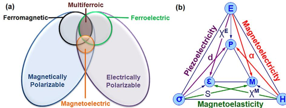
**Figure 2-21. (a) The relationship between multiferroic and magnetoelectric materials. (b) Schematic illustrating different types of coupling mechanisms present in materials. Much attention has been given to materials where electric and magnetic order parameters are coupled. These materials are known as magnetoelectric materials. Taken from [42].**
