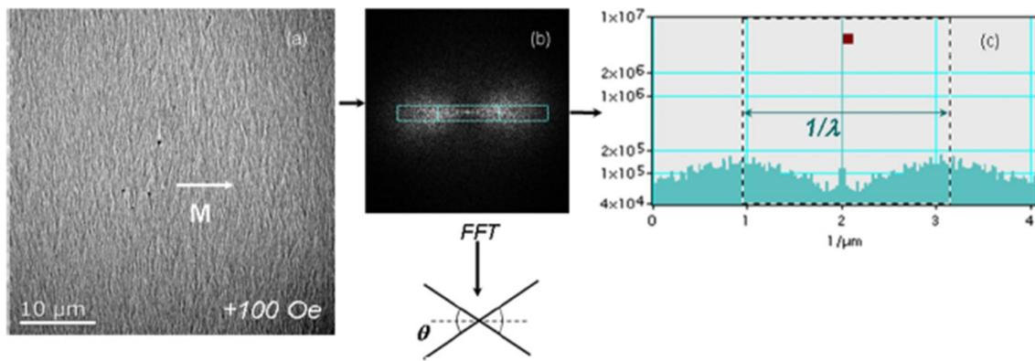
**Figure 4-4** Diagram of the calculation of ripple wavelength from Fourier transform of a Fresnel image. Taken from [83].
