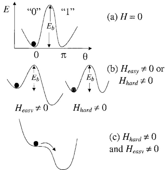
**Figure 2-20. Schematic of energy barrier  $E_b$  that separates logic 0 from logic 1 in STT-MRAM cell. (a) In zero magnetic field,  $E_b$  is maximum. (b) With applied field  $H_{hard}$  or  $H_{easy}$ ,  $E_b$  is reduced. (c) With applied field  $H_{hard}$  and  $H_{easy}$ ,  $E_b$  is reduced to 0 and the cell is programmed [12].**
