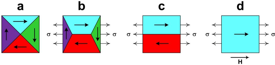
**Figure 3-3.** Schematic of magnetization of a material with positive magnetostriction under tensile stress. Adapted from [27].
