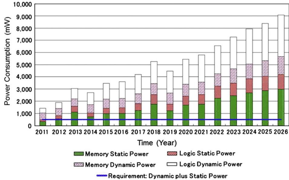
Figure 2-2 Mobile SOC power consumption trends. Taken from [14].
