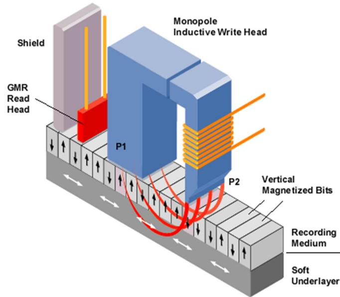
**Figure 2-14. Writing process in perpendicular recording. Taken from [31].**
