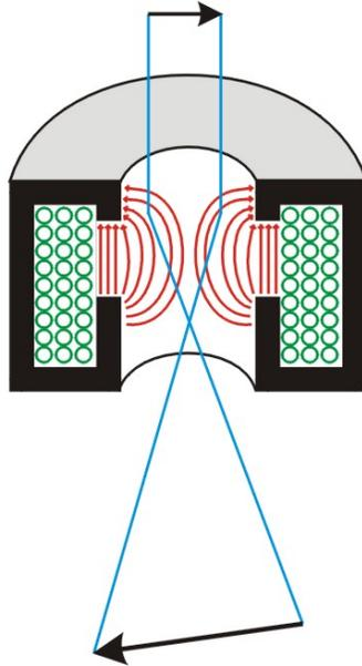
**Figure 3-11. Electromagnetic lens consisting of polepiece and copper wire coils. Adapted from [74].**
