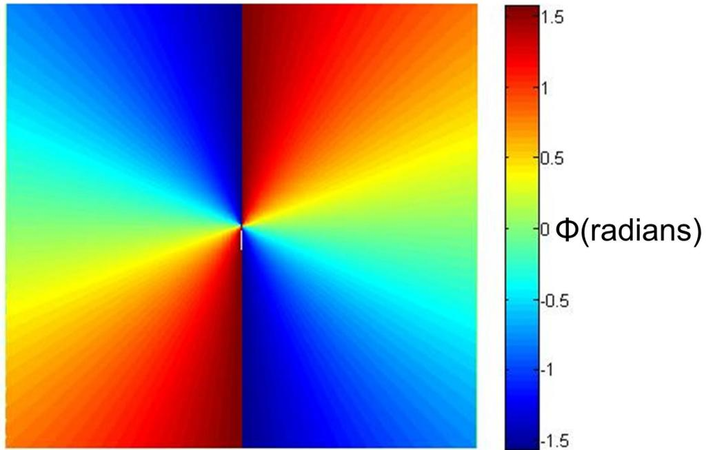
**Figure 4-12. Map of  $\phi(\vec{r})$  determined from energy minimization. The stress  $\sigma(\vec{r})$  is determined according to theoretical behavior of a plate experiencing central point-loading.**
