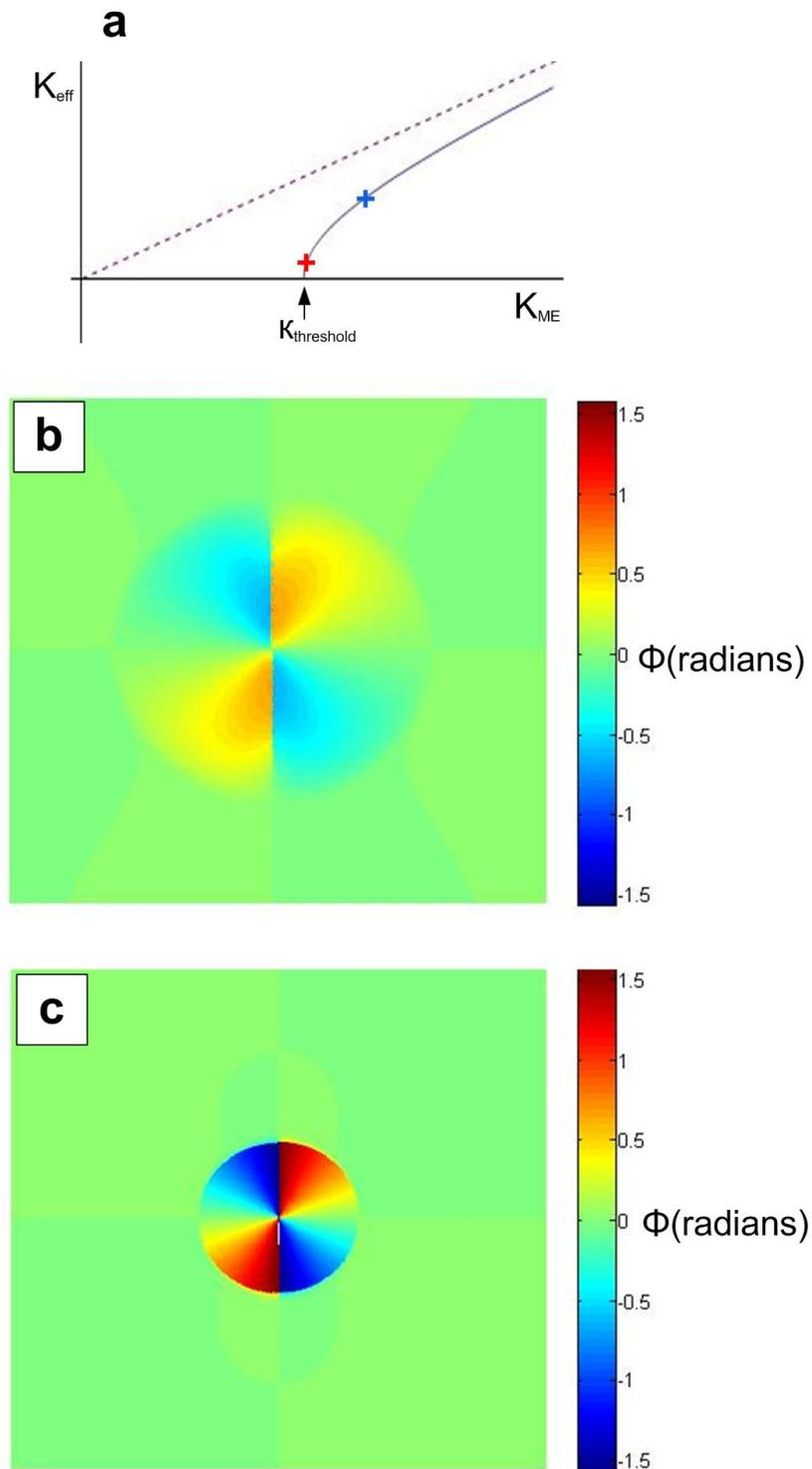
Figure 4-15. Map of  $\phi(\vec{r})$  determined from energy minimization using the OOMMF solver. The stress  $\sigma(\vec{r})$  is determined according to theoretical behavior of a plate experiencing central point-loading with an imposed threshold condition for the onset of magnetoelastic effects. The strength of the magnetoelastic effect is scaled for (a) weak and (b) strong post-onset effect.
