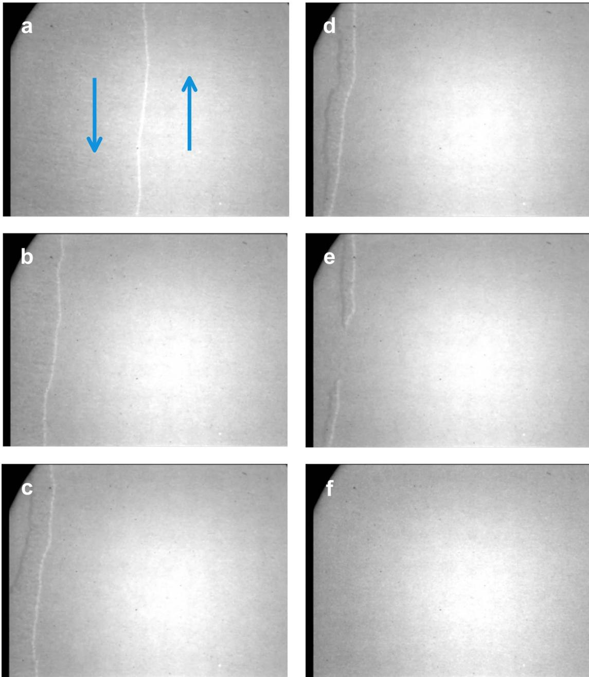
**Figure 3-17. Sequential image “stills” from a video clip demonstrating magnetization reversal in the FeGa/SiN sample with Fresnel contrast LTEM. The reversal is the result of increasing external magnetic field from -160 – +160 G. Blue arrows indicate the polarization for the two domains separated by a 180° domain wall (bright line).**
