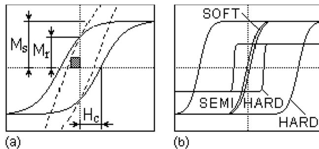
**Figure 2-8 Hysteresis loops. (a) Basic extrinsic properties derived from M-H loops. (b) Hysteresis loops of hard, semihard, and soft magnets. Taken from [23].**
