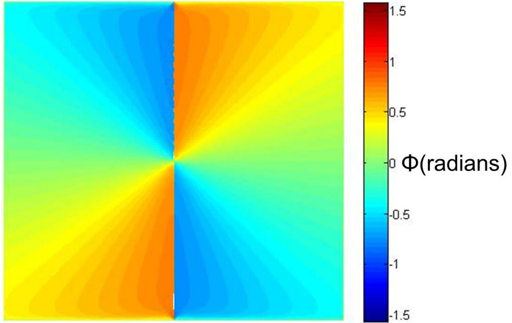
**Figure 4-13. Map of  $\phi(\vec{r})$  determined from energy minimization using the OOMMF solver. The stress  $\sigma(\vec{r})$  is determined according to theoretical behavior of a plate experiencing central point-loading.**
