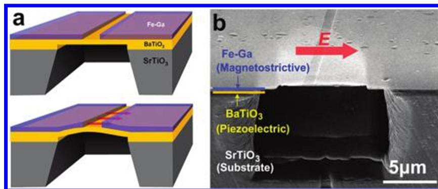
**Figure 2-26. (a) Schematic of FeGa/BaTiO<sub>3</sub> thin film bilayer structure. The bottom image represents the electric field (red arrows) that leads to mechanical response in piezoelectric BTO. (b) Scanning electron micrograph (SEM) of device. Taken from [59].**
