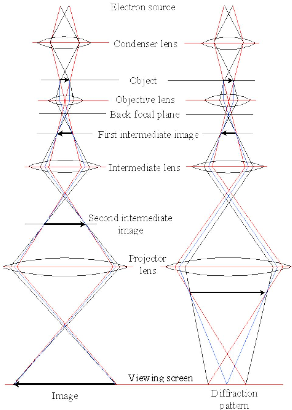
**Figure 3-12. The two basic operations of the TEM imaging system: projecting an image, and projecting a diffraction pattern. Adapted from [74].**
