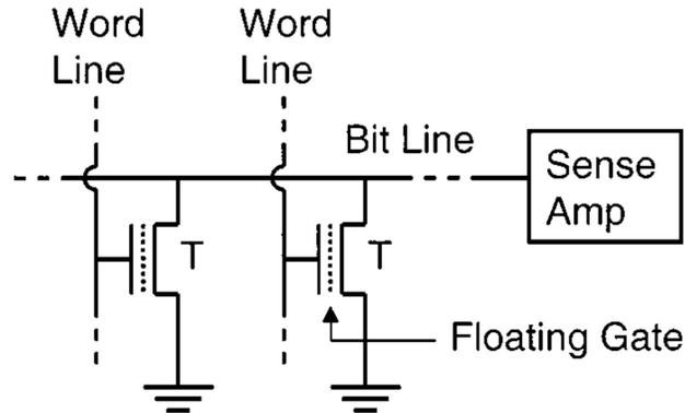
Figure 2-5 Flash memory circuit schematic. Two memory cells are depicted. Taken from [19].
