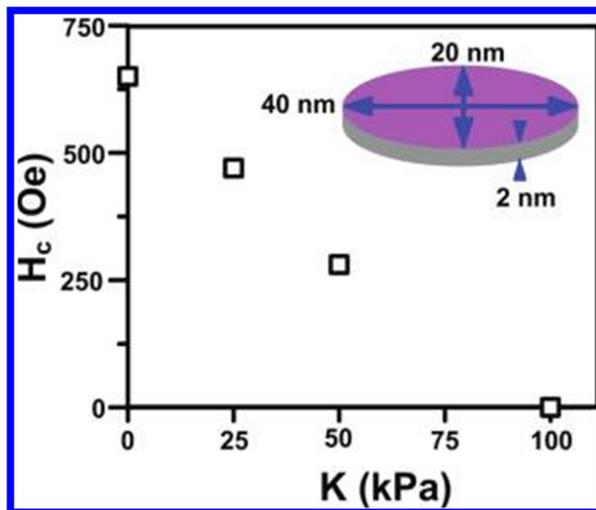
**Figure 2-29.** Demonstration of magnetoelectric memory mechanism derived using OOMMF. Inset depicts an individual ellipsoid of magnetostrictive material [59].
