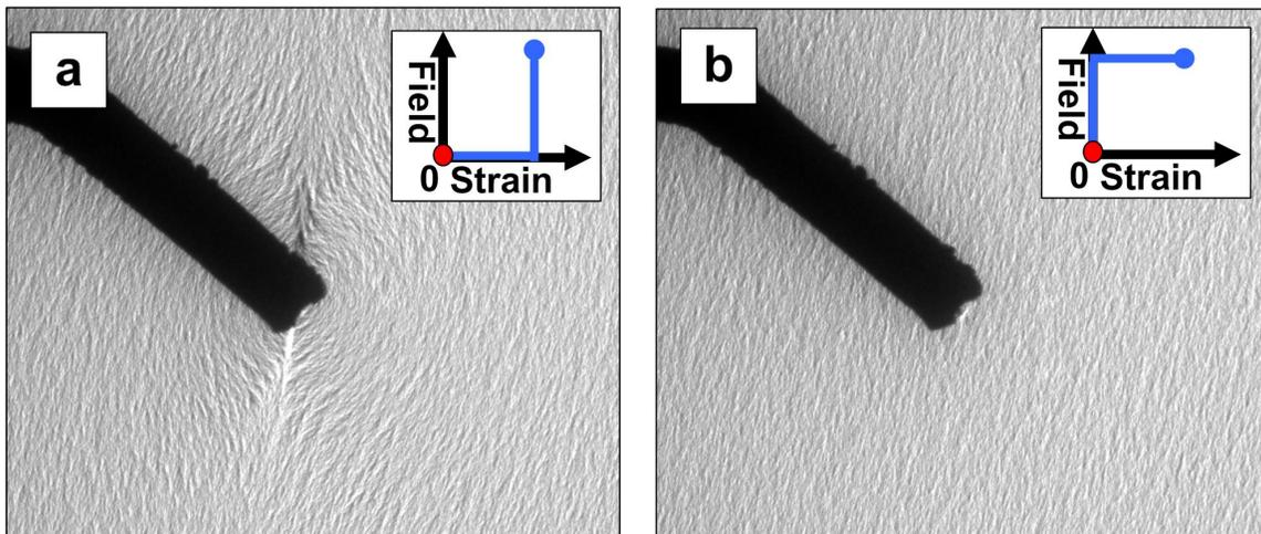
**Figure 4-3. Remanent states as a result of hysteresis in both applied field and strain. The hysteresis is depicted in the inset of the respective figure, detailing the initial state (blue dot), hysteresis path (blue line), and final state (red dot).**
