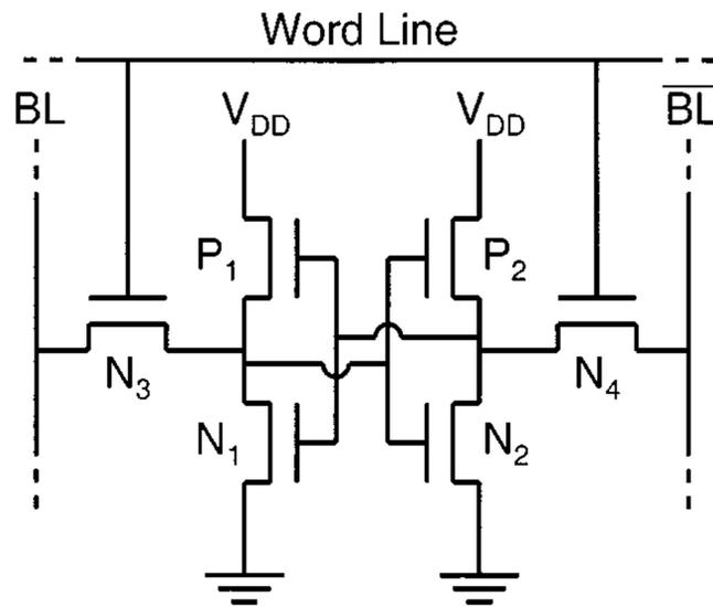
**Figure 2-3 6T SRAM cell circuit schematic. This represents one memory cell. Taken from [19].**
