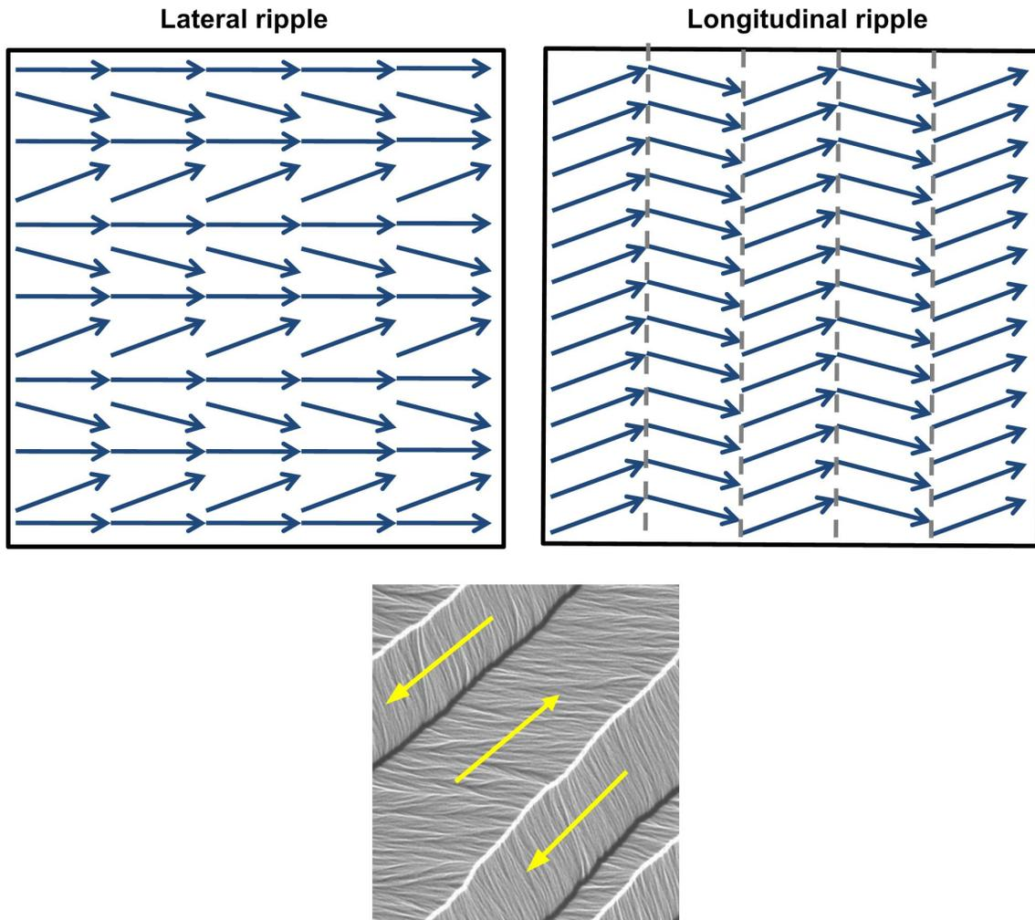
**Figure 3-14.** Schematic of lateral and longitudinal variations in local magnetic structure. The more energetically favored longitudinal arrangement results in magnetization texture that runs perpendicularly with the overall magnetization of the domain. Adapted from [75].
