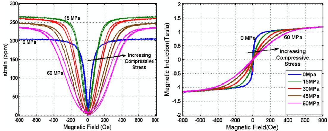
**Figure 3-5.  $\lambda$ -H (left) and B-H (right) of furnace cooled 29 at %  $\langle 100 \rangle$ -single crystal FeGa with compressive pre-stress: 0, 15, 30, 45, 60, and 80 MPa. Taken from [61].**
