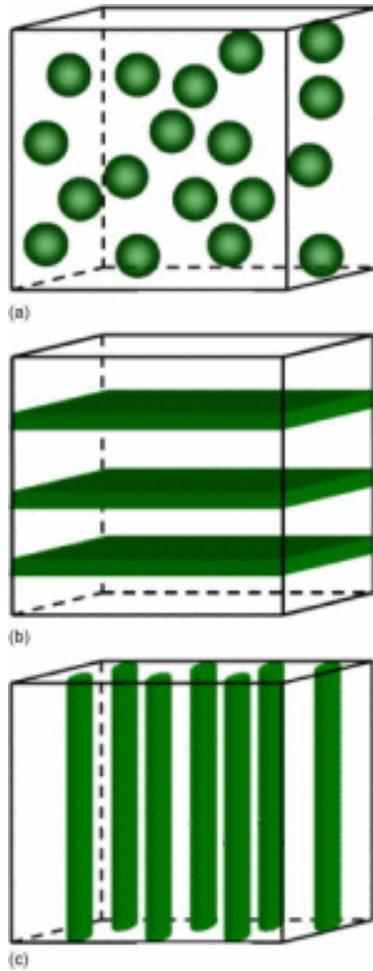
**Figure 2-22. Three common connectivity schemes in two-phase magnetoelectric composites: (a) 0-3 particulate composite, (b) 2-2 laminate composite, and (c) 1-3 fiber/rod composite. Taken from [44].**
