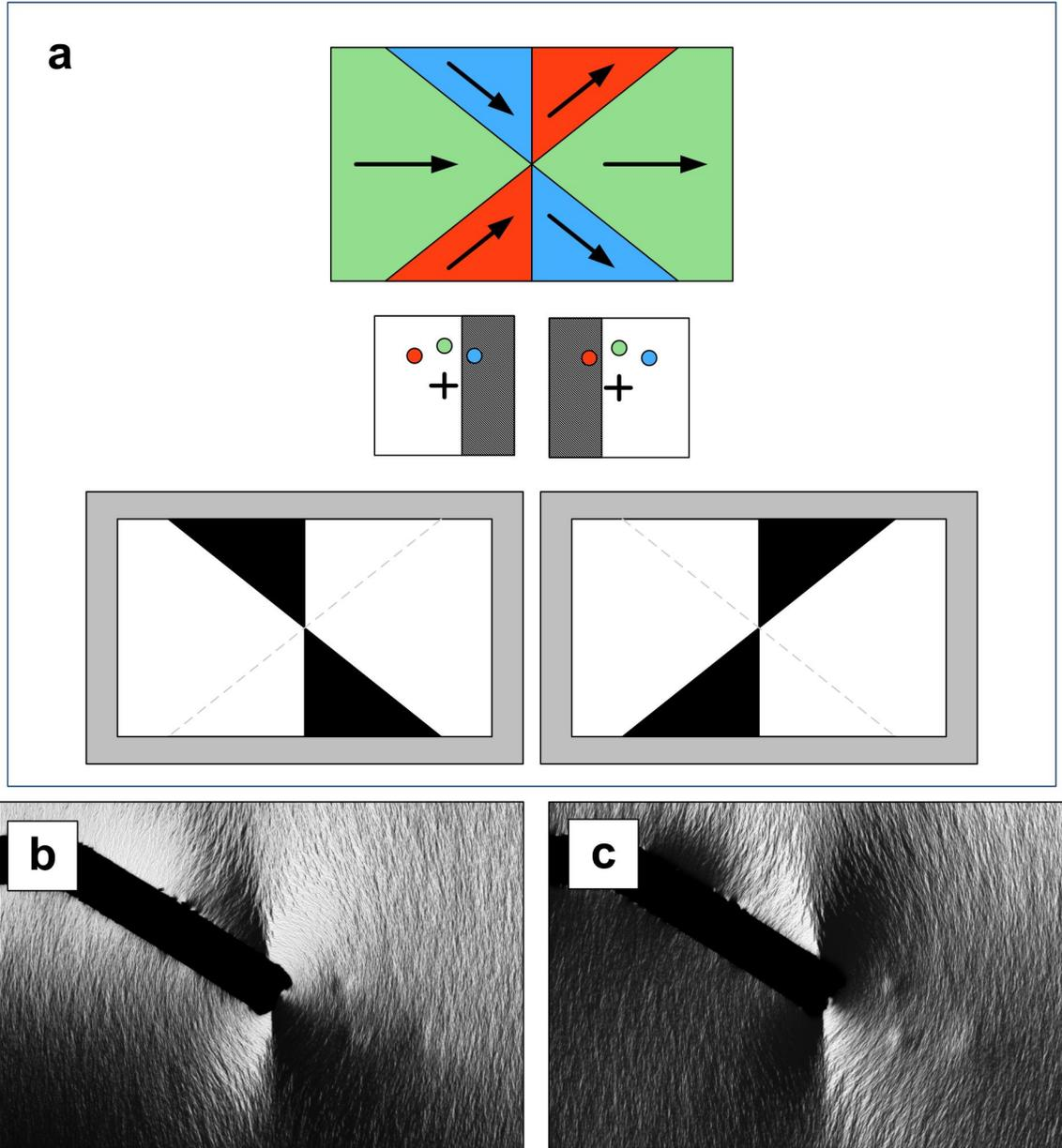
**Figure 4-2. (a) Schematic of LTEM operating mechanism for Foucault contrast. (b-c) Foucault contrast of the magnetic domain structure as a result of magnetic and mechanical stimuli. The contrast can be reversed with either a field reversal (resulting in domain reversal) or repositioning the aperture in the back-focal plane.**
