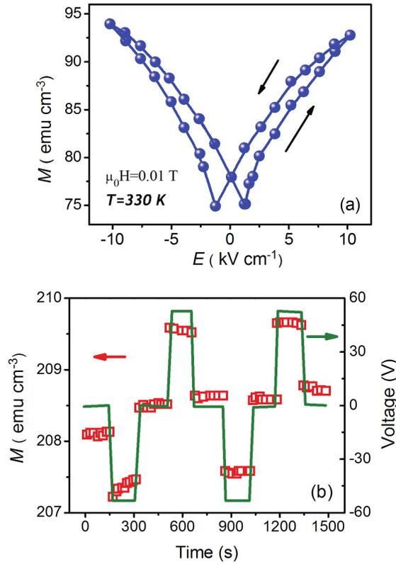
**Figure 2-25. (a)** In-plane magnetization of LSMO film grown on single-crystal PMN-PT measured using VSM with external electric field  $E$  applied across the PMN-PT substrate [57]. **(b)** The in-plane magnetization  $M$  of CFO switches as a function of time with the electric voltage pulse applied on the single-crystal PMN-PT substrate. Taken from [58].
