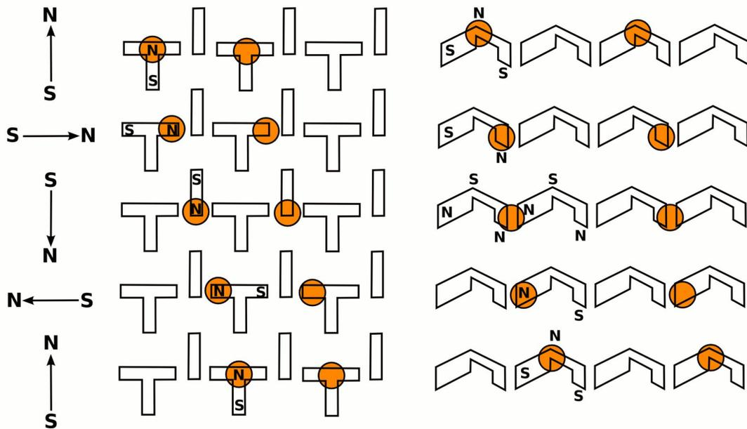
**Figure 2-11 T-bar (left) and chevron (right) propagation circuits. Adapted from [28].**
