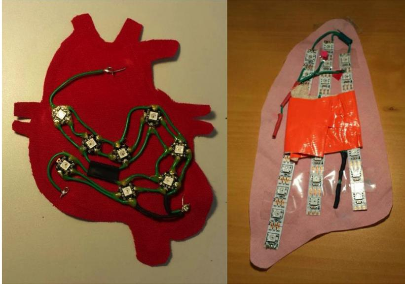
**Figure 29: Prototype 2.1 now uses insulated stranded wire as opposed to conductive thread in the heart and lungs.**
