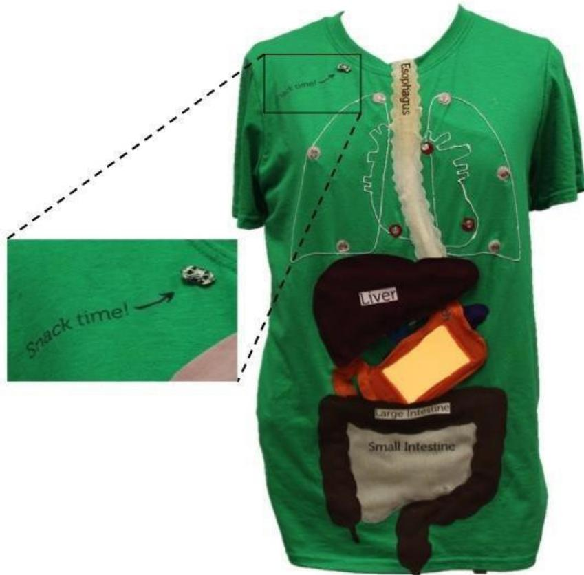
**Figure 33: The “snack time” button triggers the digestive system shown here.** stomach and embedded LEDs in the remaining digestive system organs. The visualization begins with a push of the “Snack time!” button (Figure 33). The esophagus, which consists of a Neopixel LED strip covered with fabric, lights up to illustrate the movement of food traveling down (Figure 34).
