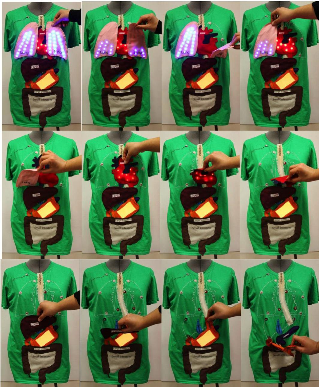
**Figure 28: Magnets are used to connect the removable organs to the shirt.**
