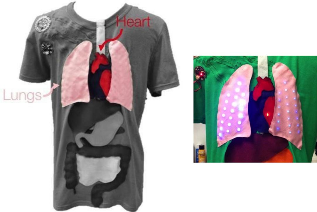
Figure 16: A snapshot of the heart and lungs in Prototype 2.0 (left) and a close up of the heart and lungs visualization (right). Here, the lungs are fully “inflated” as indicated by all the lit LEDs.
