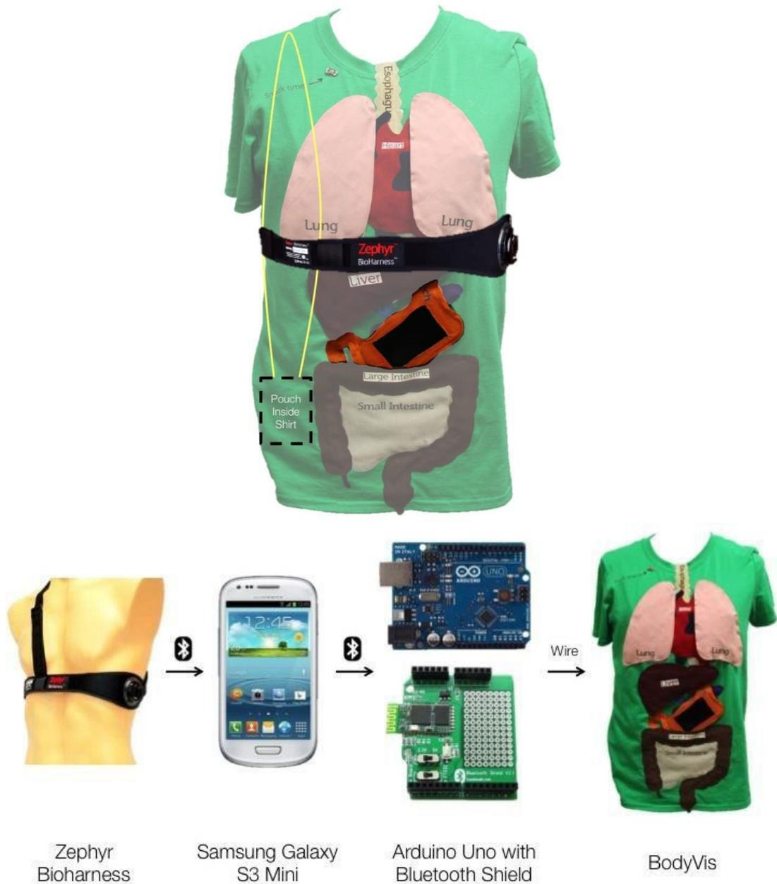
**Figure 32: The Bioharness (shown on top of shirt for clarity), Android phone (Galaxy S3 Mini), and Arduino (in pouch) are embedded into the shirt (on top). The Bioharness sends bio-data to the Android phone via Bluetooth; the phone translates this data and sends it to the Arduino via Bluetooth; the Arduino is wired to and controls the LEDs in the organs (on bottom).**
