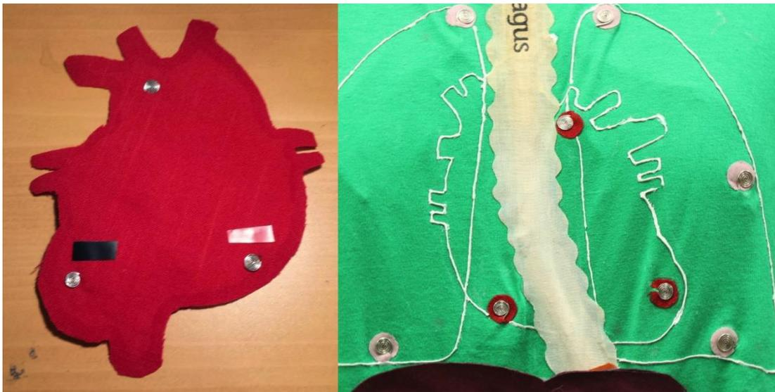
**Figure 27: The back of the heart (left) contains three spiraled wires that, when attached to the shirt, turn on its visualization. The heart's points of contact on the shirt (right) can be located using the red "highlighters" and white outline.**
