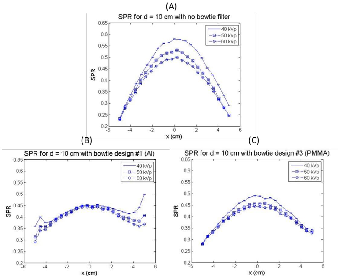
Figure 5.5: Experimental SPR values for various tube voltages using (A) no-bowtie filter, (B) bowtie design #1 and (C) bowtie design #3.
