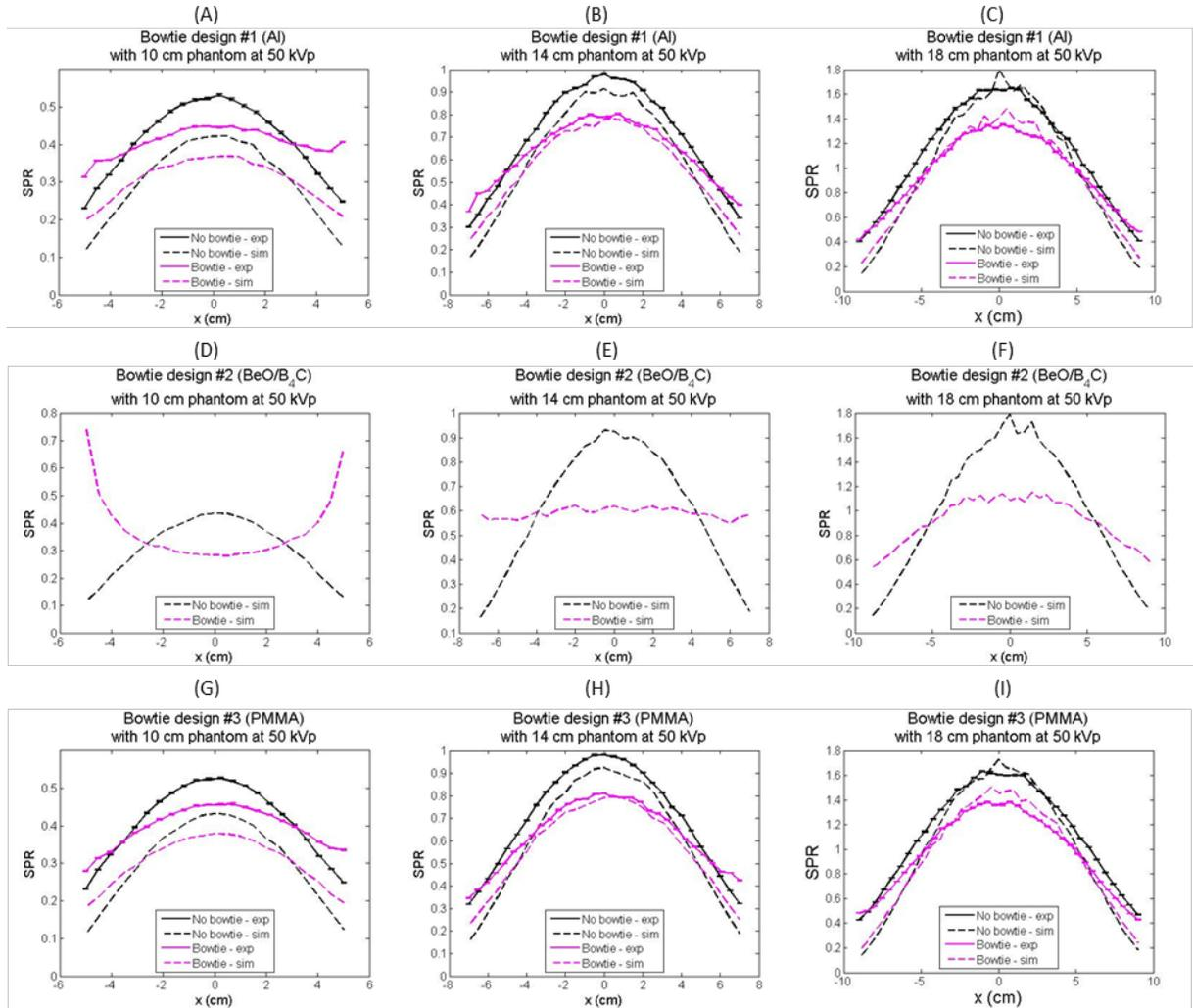
Figure 5.8: SPR value for various diameter phantoms using (A-C) bowtie design #1 (Al), (D-F) bowtie design # 2 ( $\text{BeO/B}_4\text{C}$ ) and (G-I) bowtie design #3 (PMMA). Both experimental and simulation values of SPR are shown at a tube voltage of 50 kVp.
