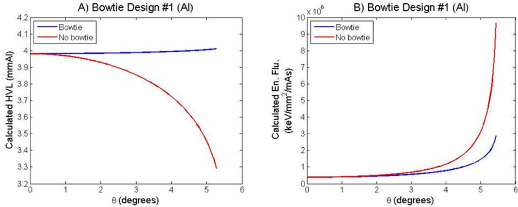
Figure 3.2: Calculated HVL (A) and energy fluence (B) as a function of fan angle with and without bowtie filter design #1.
