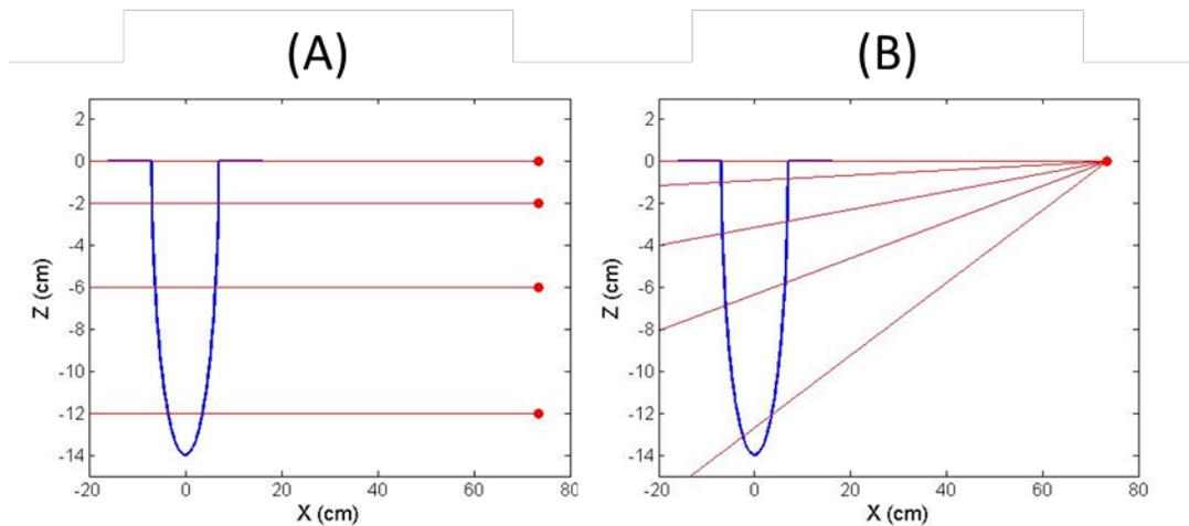
Figure 8.1: Ray traces through the half-ellipsoidal shape representing the pendant breast for the (A) fan-beam case and the (B) cone-beam case from a point source 73.5 cm away from the center of the breast. Each plot shows the half-ellipsoidal shape in the  $xz$ -plane.
