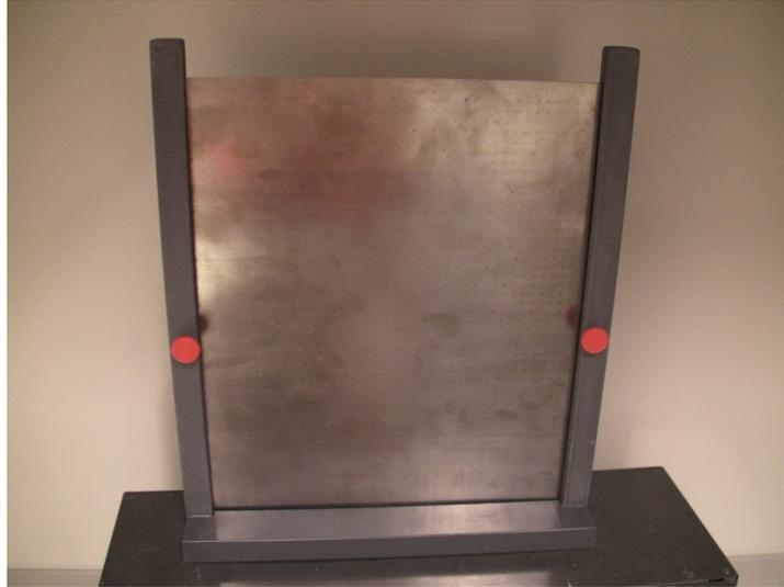
Figure 6.4 Tungsten plate used for scatter correction in experimental study
