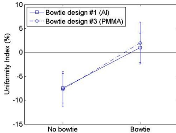
Figure 6.11: Noise uniformity index calculated using the 14-cm diameter phantom with and without bowtie design #1 (Al) and bowtie design #3 (PMMA).
