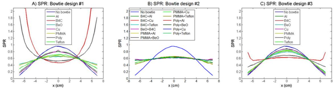
Figure 4.9: SPR calculated from simulated projection data for (A) bowtie design #1, (B) bowtie design #2, and (C) bowtie design #3 for various materials.
