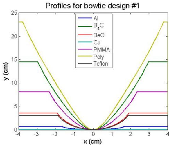
Figure 4.2: Cross-section profile of bowtie design #1 materials using seven different investigated materials.
