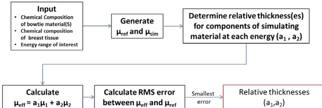
Figure 2.3: Flowchart detailing the steps in generating the thickness values ( $a_1, a_2$ ) for bowtie design #2 that transmits the same spectral shape and intensity as breast tissue.
