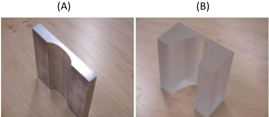
Figure 6.1: Images of the two bowtie filters validated computationally and manufactured for experimental validation and evaluation. The image is (A) shows bowtie design #1 made of aluminum and (B) shows bowtie design #3 made of PMMA.
