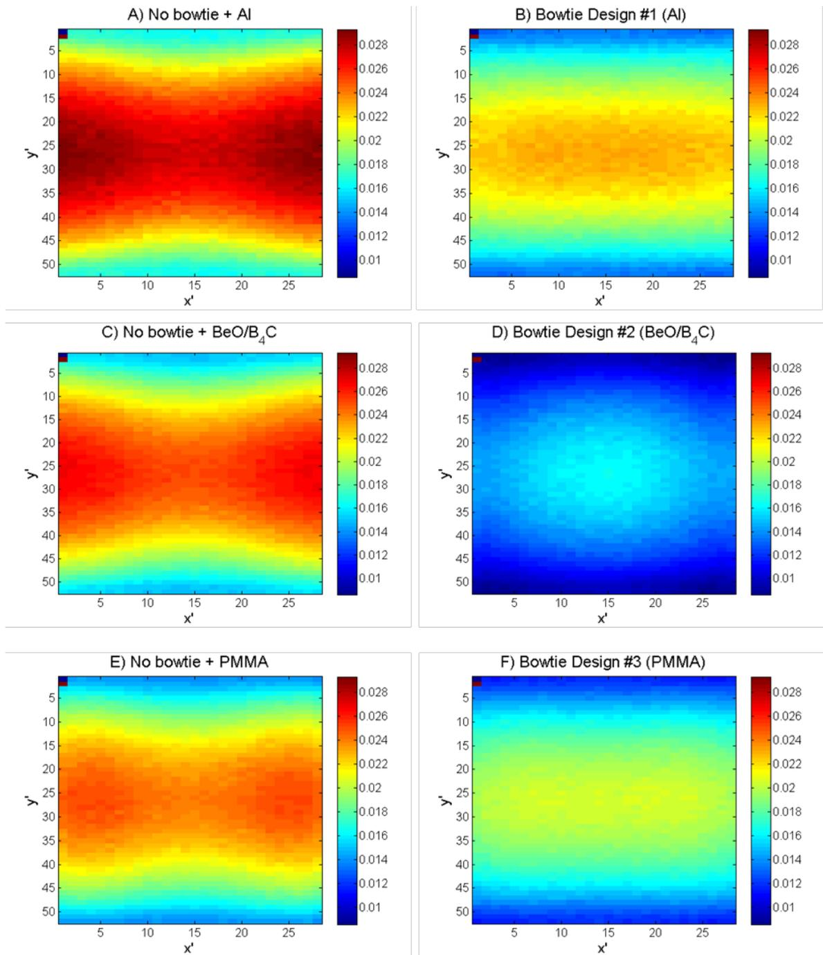
Figure 5.11: Scatter distribution using the SOCR metric for the three bowtie filter types using a 14 cm diameter breast phantom and a tube voltage of 50 kVp. A, C, E show the scatter distributions with no-bowtie filter, but include the constant thickness base from the bowtie filter so that a valid comparison between the two cases can be made. The variables  $x'$  and  $y'$  represent the bin number of the re-binned scatter image used to compute the SOCR.
