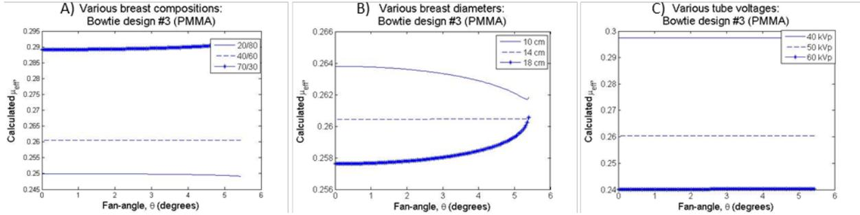
Figure 3.8: Calculated effective attenuation coefficient across object FOV for (A) various breast compositions, (B) various breast diameters, and (C) various tube voltages using bowtie design #3 (PMMA).
