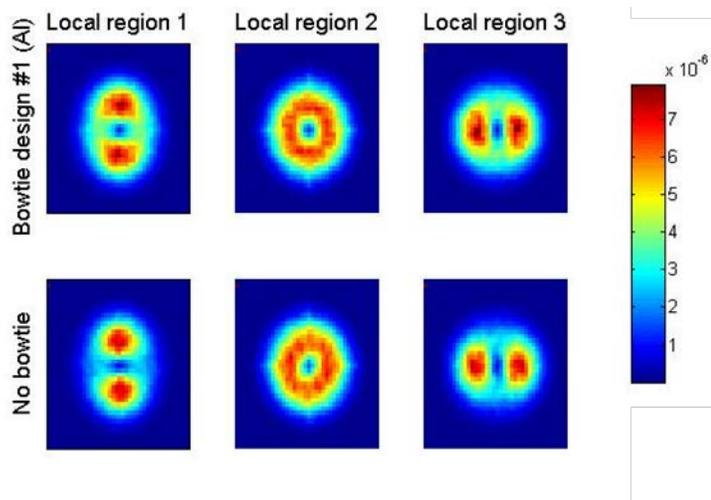
Figure 8.4: Location-dependent 2D NPS with and without bowtie design #1 (Al). The bowtie/no-bowtie filter cases are each plotted on the same scale.
