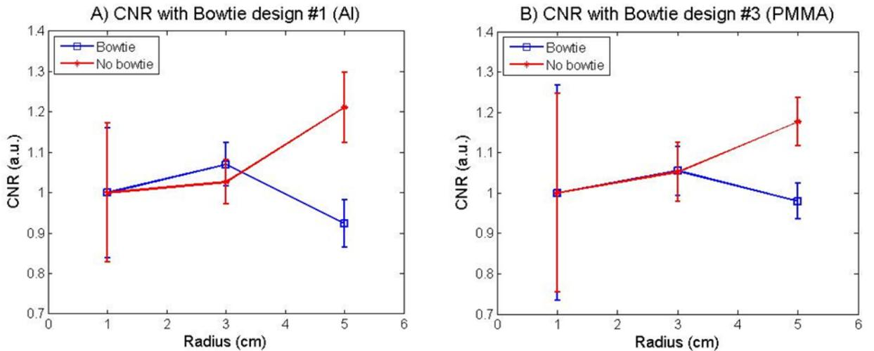
Figure 6.12: CNR calculations as a function of radial distance using (A) bowtie design #1 (Al) and (B) bowtie design #3 (PMMA). The results are normalized to the central CNR value.
