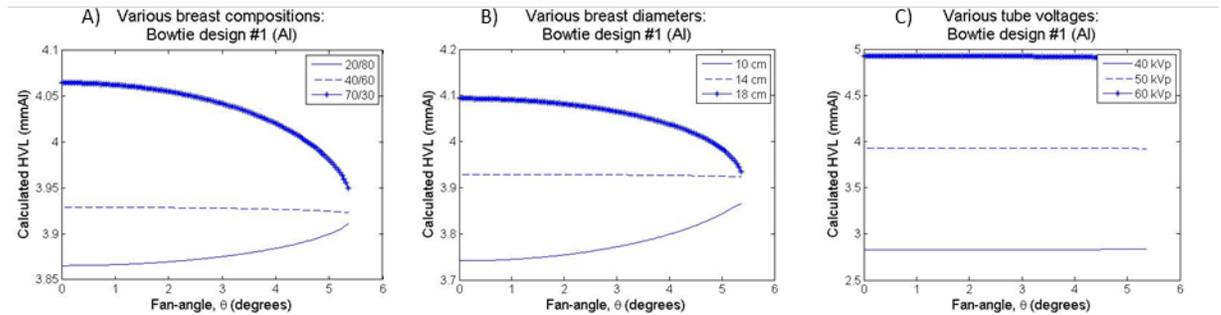
Figure 3.6: Calculated HVL for (A) various breast compositions, (B) various breast diameters, and (C) various tube voltages.
