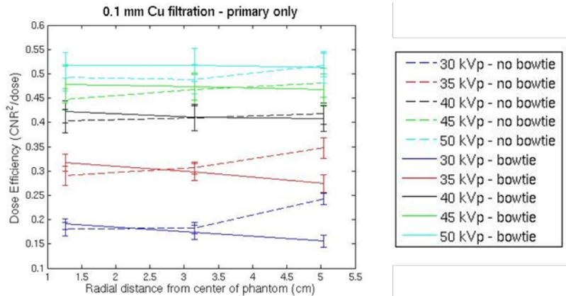
Figure 7.6: DE metric calculated from simulation data both with and without bowtie design #2 for various tube voltages. The DE was calculated using the reconstructed volume from the primary only projection images. The flat filter used in these data was 0.1 mm Cu.
