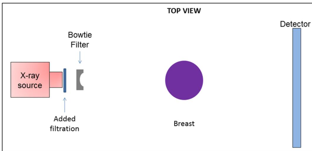
Figure 1.3: Top-side view of a dedicated breast CT system set-up with the inclusion of a bowtie filter between the x-ray source and the breast.
