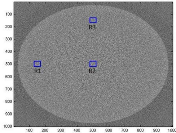
Figure 8.3: A single slice from the reconstructed volume used to compute the location-dependent NPS. The blue squares labeled R1, R2, and R3 show the regions extracted from each slice for the NPS analysis.
