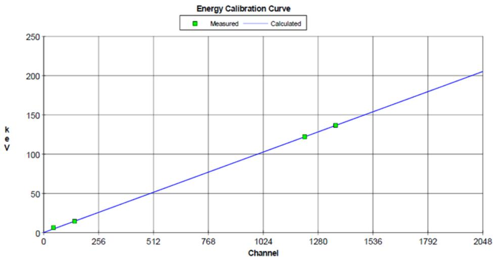
Figure 2.5: Calibration curve using the energy peaks from a Co-57 source. The known energy of the  $\gamma$ -ray emission is given on the y-axis, and the corresponding channel of the measured peak is shown on the x-axis. The calculated linear fit (blue line) allows for the conversion between channel and energy.
