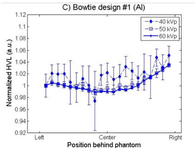
Figure 6.9: Normalized HVL measurements behind the phantom FOV for various parameters using bowtie design #1 (Al). The HVL was measured with various (A) breast compositions, (B) breast phantom diameters, and (C) tube voltages.
