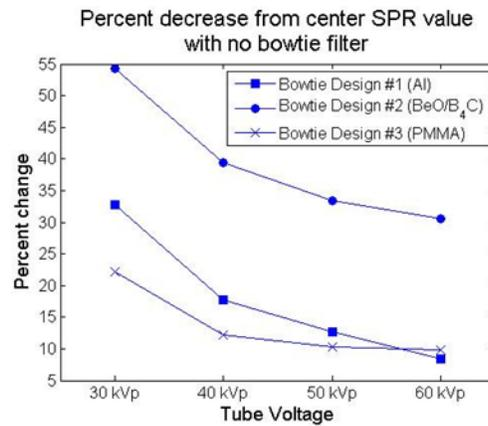
Figure 5.7: Calculated percent change from center SPR value (at  $x = 0$ ) with no-bowtie filter and center SPR value with bowtie filter for various tube voltages.
