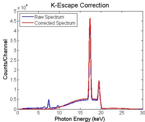
Figure 2.6: Raw spectrum and corrected spectrum for K-edge escape in the Ge detector.
