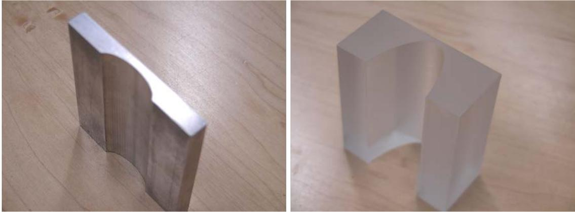
Figure 5.1: Images of the two bowtie filters used for experimental analysis of scatter in dedicated breast CT. (Left) Bowtie design #1 made of aluminum that transmits the same quality of radiation as breast tissue. (Right) Bowtie design #3 made of PMMA that yields the same effective attenuation coefficient at the detector.
