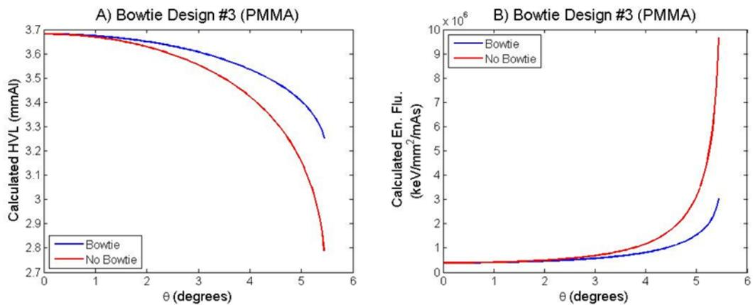
Figure 3.4: Calculated HVL (A) and energy fluence (B) as a function of fan-angle with and without bowtie design #3 (PMMA).
