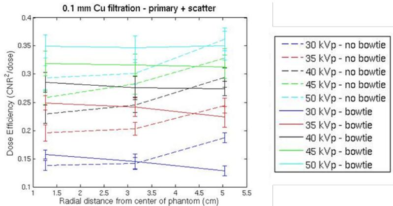
Figure 7.7: DE metric calculated from simulation data both with and without bowtie design #2 for various tube voltages. The DE was calculated using the reconstructed volume from the primary + scatter projection images. The flat filter used in these data was 0.1 mm Cu.
