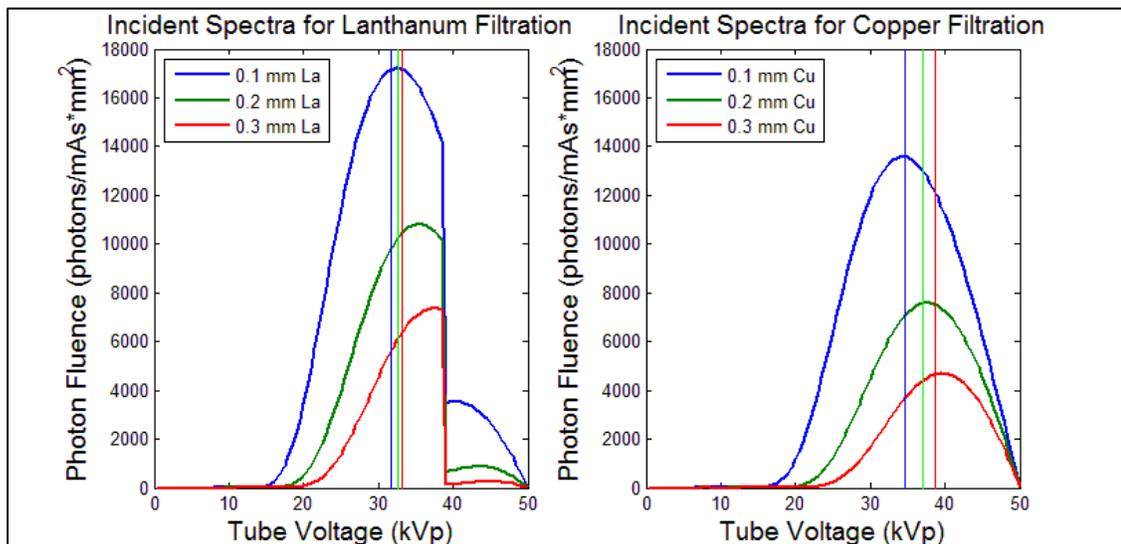
Figure 7.1: Simulated spectra using different thicknesses of lanthanum and copper filtration. With lanthanide filtration, we get a greater degree of monochromaticity with average energies in the ideal energy range. Initial spectrum is from IPEM Report 78.
