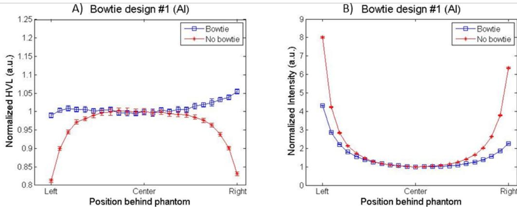
Figure 6.7: Measured values behind phantom FOV with and without bowtie design #1 (Al) normalized to the center value. (A) The measured HVL is plotted as a function of position behind the phantom with and without the bowtie filter. (B) The measured intensity as a function of position behind the phantom is plotted with and without the bowtie filter.
