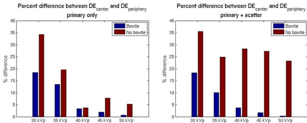
Figure 7.8: Percent difference between the center DE value and peripheral DE value with and without bowtie design #2 for various tube voltages using 0.1 mm Cu filtration. (Left) The primary only reconstructed volume was used to compute the DE. (Right) The primary + scatter reconstructed volume was used to compute the DE.
