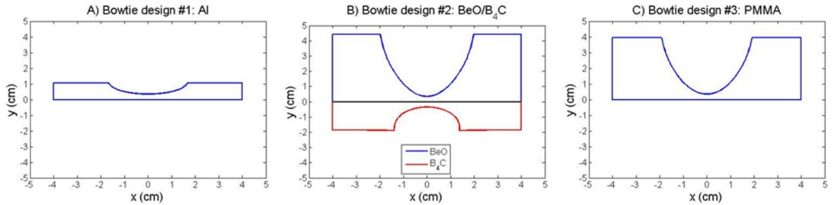
Figure 5.2: Cross-section views of the bowtie filter designs using (A) aluminum for bowtie design #1, (B) BeO/B<sub>4</sub>C for bowtie design #2, and (C) PMMA for bowtie design #3.
