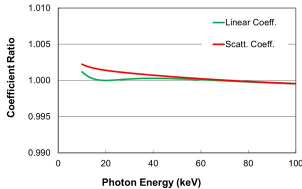
Figure 2.8: Ratio of the linear attenuation coefficient and scatter coefficient for the liquid mixture and the reference material, 25% fibroglandular/75% adipose breast tissue.
