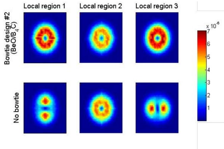
Figure 8.5: Location-dependent 2D NPS with and without bowtie design #2 (BeO/B<sub>4</sub>C). The bowtie/no-bowtie filter cases are each plotted on the same scale.
