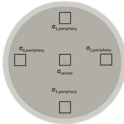
Figure 3.14: Placement of the VOI in the uniform composition breast phantom to calculate the noise uniformity index.
