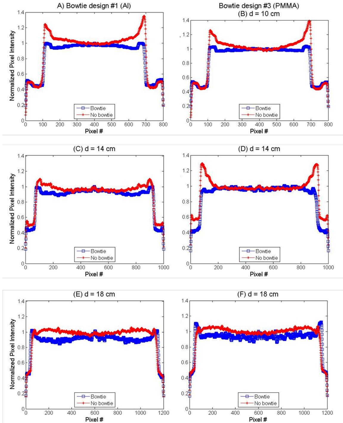
Figure 6.10: Line profiles of central slice of reconstructed images with and without bowtie design #1 (Al) and bowtie design #3 (PMMA). Plots A, C, E show the line profiles with and without bowtie design #1 (Al) for various phantom diameters. Plots B, D, F show the line profiles with and without bowtie design #3 (PMMA) for various phantom diameters.
