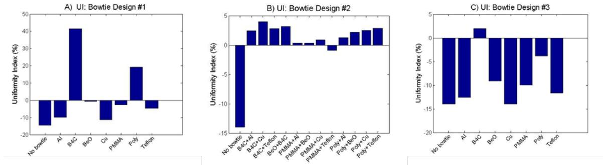
Figure 4.8: Noise uniformity index for (A) bowtie design #1, (B) bowtie design #2, and (C) bowtie design #3 with various materials.
