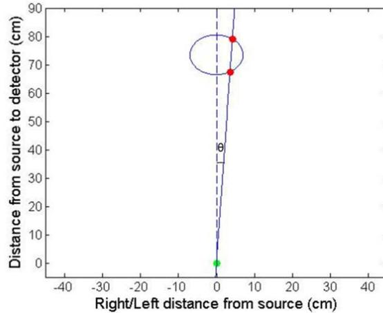
Figure 2.7: Path of photons from the x-ray source through the breast phantom at an angle,  $\theta$ . The green dot represents the source and the red dots represent the intersection of the ray and the phantom.
