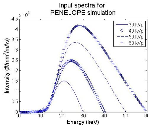
Figure 5.3: Number of simulated photons per energy bin for each simulated tube voltage.
