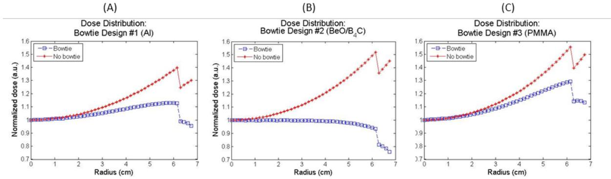
Figure 3.10: Dose profile from center to periphery of cylindrical phantom for all bowtie filter and no bowtie filter cases. Normalized dose for the 14-cm phantom at 50 kVp using bowtie design #1 (A), bowtie design #2 (B), and bowtie design #3 (C).
