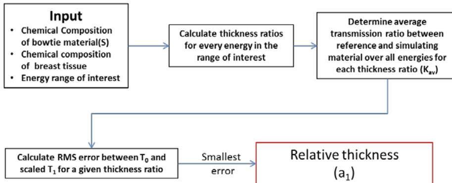
Figure 2.2: Flow chart detailing the steps in generating the relative thickness value used in the computational methods for designing the single material bowtie filter that transmits the same spectral shape as breast tissue.
