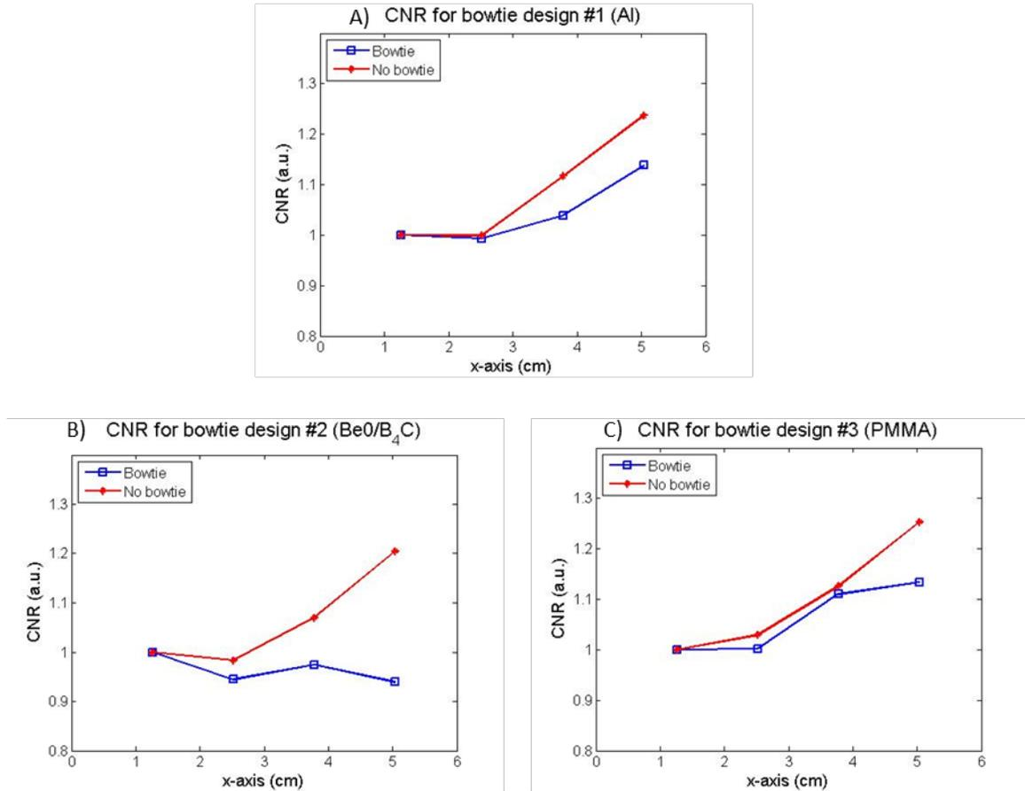
Figure 3.16: CNR values normalized to the innermost contrast insert value for three different bowtie filters. These data points were calculated for the 14-cm diameter phantom at 50 kVp. The results are shown for (A) bowtie design #1 (Al), (B) bowtie design #2 (BeO/B<sub>4</sub>C), and (C) bowtie design #3 (PMMA) with the respective no-bowtie filter cases.
