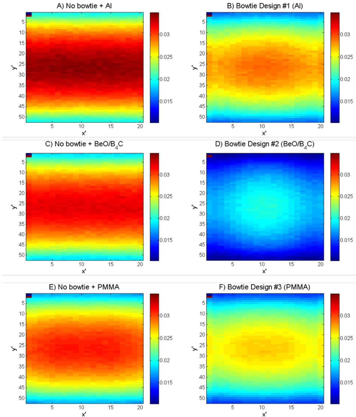
Figure 5.10: Scatter distribution using the SOCR metric for the three bowtie filter types using a 10 cm diameter breast phantom and a tube voltage of 50 kVp. A, C, E show the scatter distributions with no-bowtie filter, but include the constant thickness base from the bowtie filter so that a valid comparison between the two cases can be made. The variables  $x'$  and  $y'$  represent the bin number of the re-binned scatter image used to compute the SOCR.
