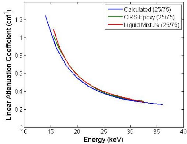
Figure 2.9: Calculated (blue) and spectrally measured and fit (green and red) linear attenuation coefficients for 25% fibroglandular/75% adipose breast tissue, CIRS epoxy phantom simulating 25% fibroglandular/75% adipose breast tissue, and a liquid mixture simulating 25% fibroglandular/75% adipose breast tissue. These data are from a 35 kVp spectrum.
