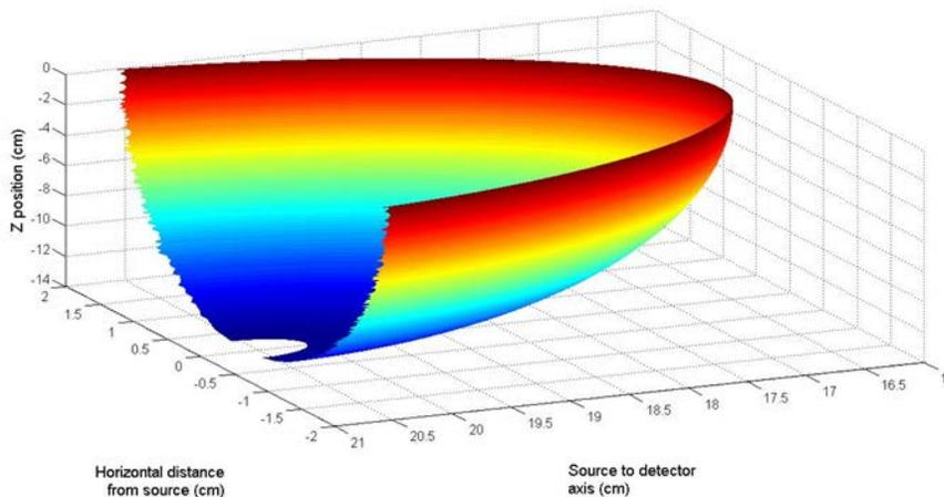
Figure 8.2: 3D plot of an anthropomorphic bowtie filter of design #3 assuming a fan-beam geometry. The different colors represent the filter shape for a given  $z$  position.
