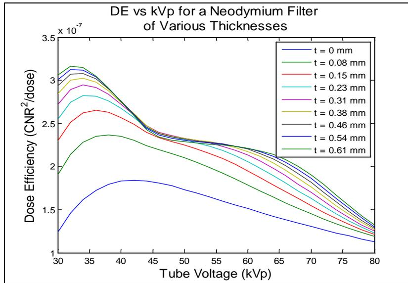
Figure 7.4: Dose efficiency vs. tube voltage for a neodymium filter of various thicknesses.
