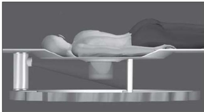
Figure 1.1: Schematic of clinical prototype dedicated breast CT scanner.<sup>10</sup> The x-ray source is shown on the left with the flat panel detector shown on the far right.
