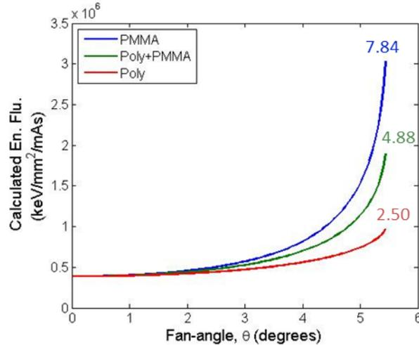
Figure 4.6: Demonstration of the flexibility of bowtie design #3 in specifying the dynamic range. The calculated energy fluence for bowtie design #3 made of PMMA and polyethylene as a function of fan-angle are shown, as well as the achieved dynamic range with the combination of PMMA and polyethylene. The numbers next to each line show the dynamic range.
