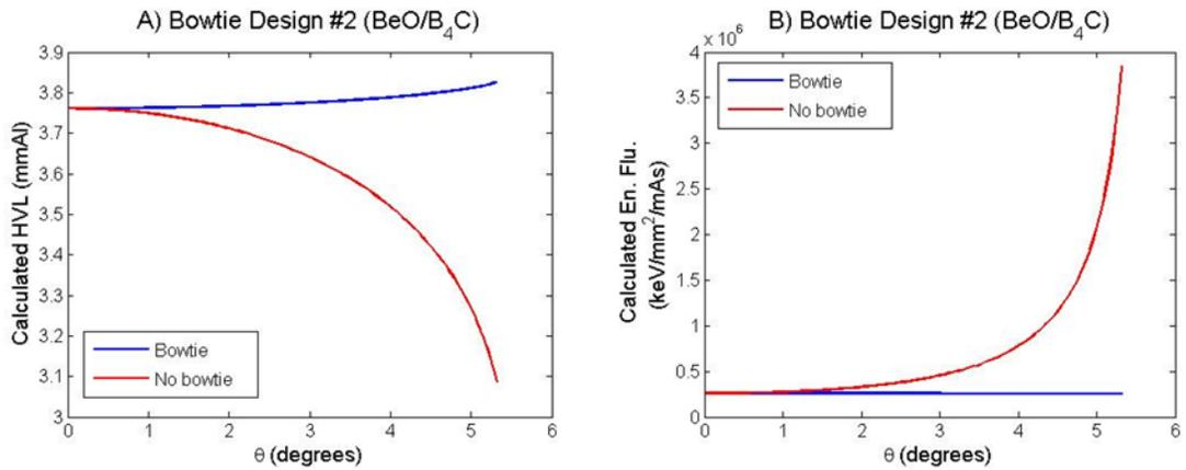
Figure 3.3: Calculated HVL (A) and energy fluence (B) as a function of fan angle with and without bowtie filter design #2.
