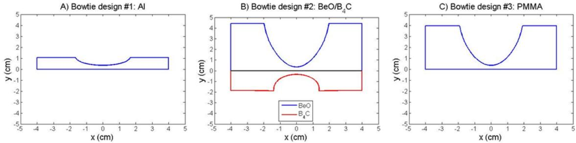
Figure 3.1: Cross-section views of the bowtie filter designs using (A) aluminum for bowtie design #1, (B) BeO/B<sub>4</sub>C for bowtie design #2, and (C) PMMA for bowtie design #3.
