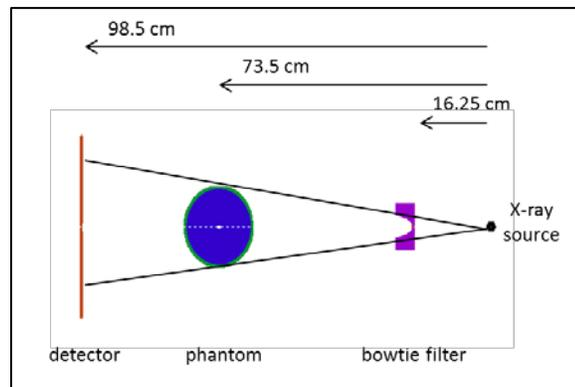
Figure 3.9: Breast CT simulation set-up.
