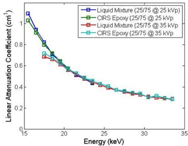
Figure 2.10: Spectrally measured linear attenuation coefficient at 25 kVp and 35 kVp for the CIRS epoxy phantom and liquid mixture simulating 25% fibroglandular/75% adipose breast tissue.
