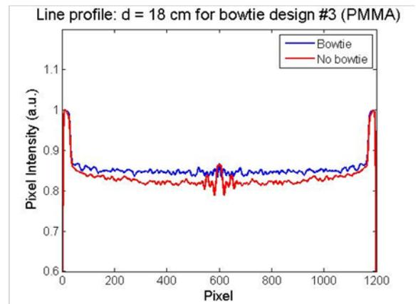
Figure 3.12: Line profiles through 14-cm breast phantom with and without bowtie design #1 (Al) (top), bowtie design #2 (BeO/B<sub>4</sub>C) (center), and bowtie design #3 (PMMA) (bottom).
