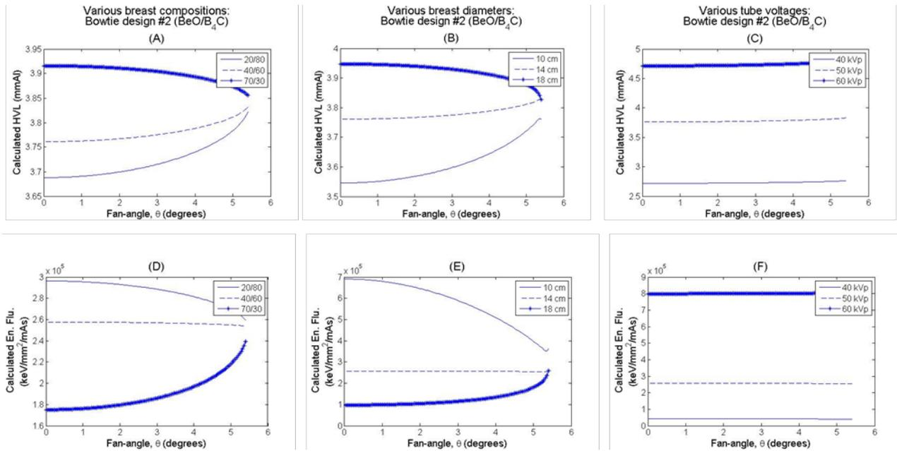
Figure 3.7: Calculated HVL and energy fluence for various breast compositions, breast diameters, and tube voltages for bowtie design #2 (BeO/B<sub>4</sub>C). Plots (A) – (C) show the calculated HVL and (D) – (F) show the calculated energy fluence.
