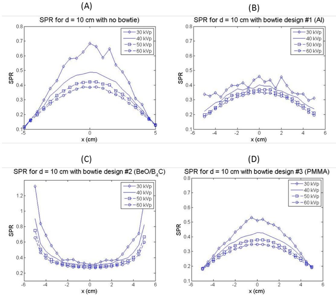
Figure 5.6: SPR calculations from simulated images for various tube voltages using (A) no-bowtie filter, (B) bowtie design #1 (Al), (C) bowtie design #2 (BeO/B<sub>4</sub>C), and (D) bowtie design #3 (PMMA).
