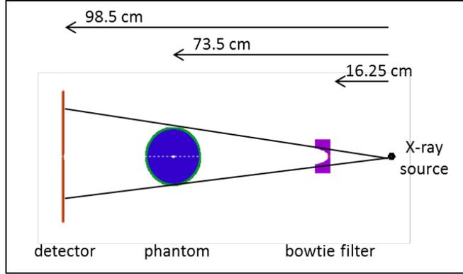
Figure 4.1: Breast CT simulation set-up.
