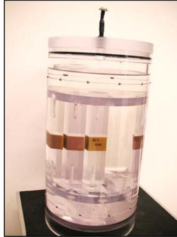
Figure 6.2: Cylindrical 14-cm diameter phantom with CNR insert.<sup>82</sup> The phantom contains three 100% glandular equivalent blocks from the center to the periphery to calculate the CNR homogeneity.
