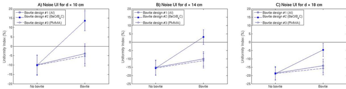
Figure 3.15: Noise uniformity index for all bowtie filter designs and no bowtie filter cases for three breast diameters. The bowtie and no bowtie case for all three bowtie filters is shown in each plot for breast diameters of (A) 10 cm, (B) 14 cm, and (C) 18 cm.
