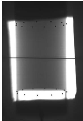
Figure 5.4: Experimental projection image using the lead strip beam block method.
