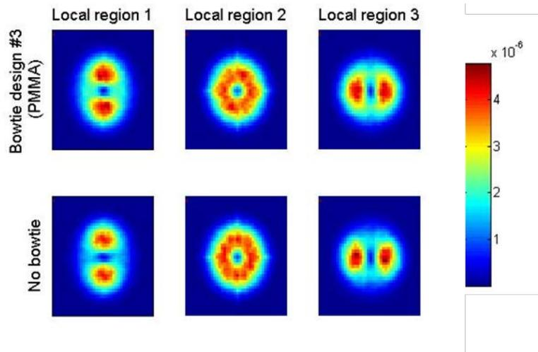
Figure 8.6: Location-dependent 2D NPS with and without bowtie design #3 (PMMA). The bowtie/no-bowtie filter cases are each plotted on the same scale.
