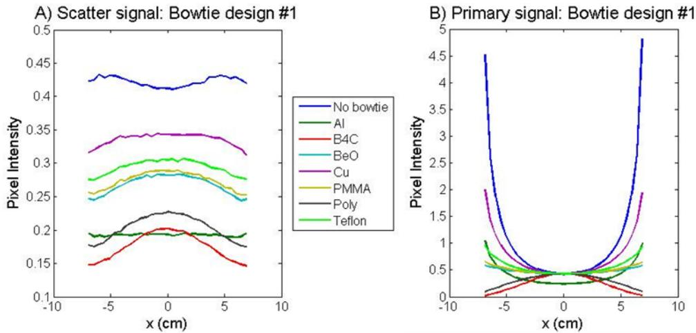
Figure 4.10: Scatter and primary signal from simulated projection images using various materials for bowtie design #1. (A) The averaged scatter signal over all projection images as a function of horizontal distance across the phantom for different materials. (B) The averaged primary signal over all projection images as a function of horizontal distance across the phantom for different materials.
