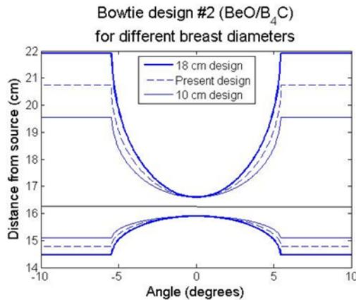
Figure 5.13: Comparison of bowtie designs for the 10-cm diameter and 18-cm diameter phantoms with the design used in the present study (14-cm diameter phantom). The shape of the two-material bowtie filter designed specifically for the 10-cm phantom is shown as the thin solid line while the specific design for the 18-cm phantom is shown as the thick solid line. The 14-cm phantom design used in the present study is shown as a dotted line.
