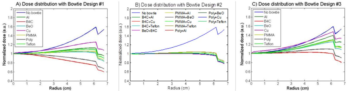
Figure 4.7: Dose distributions as a function of radial distance from the center of the phantom for (A) bowtie design #1, (B) bowtie design #2, and (C) bowtie design #3, using various materials. The y-axis is the dose normalized by the dose value at the center of the phantom.
