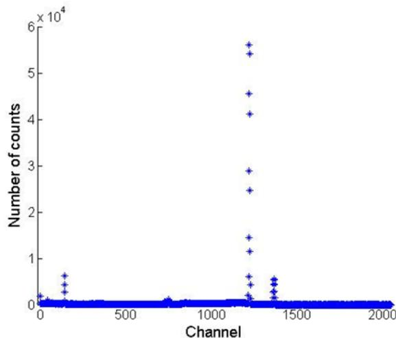
Figure 2.4: Calibration spectrum from Co-57 source used to determine the gain and offset for calibration of channels to energy.
