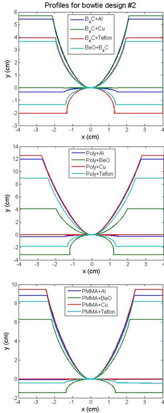
Figure 4.3: Cross section profile of bowtie design #2. The profiles of the 12 possible combinations from the seven materials being investigated were plotted in three different plots for easier viewing. Each bowtie filter combination is listed as a legend entry. The first material in the legend entry is plotted as a colored line above  $y = 0$ . The second material in the legend entry is plotted as the same colored line below  $y = 0$ .
