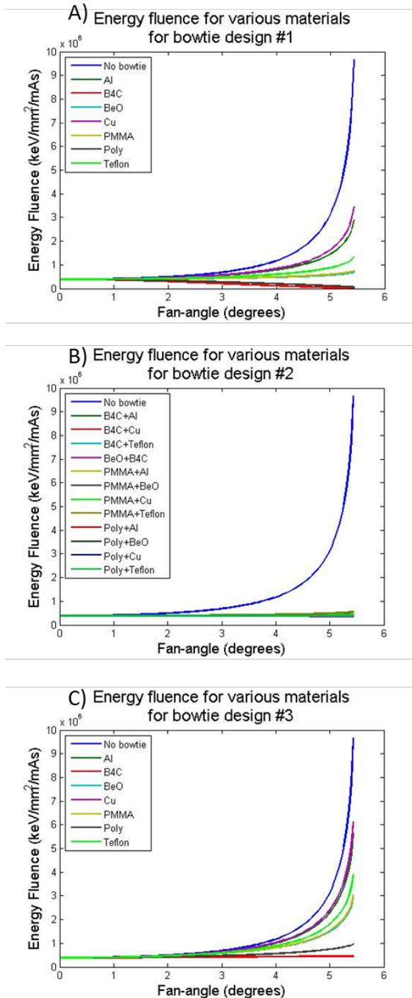
Figure 4.5: Energy fluence as a function of fan-angle plotted for three different bowtie filters using different materials to examine the dynamic range requirement. These plots show the energy fluence after the photons have traveled through the bowtie filter and the phantom. (A) Bowtie design #1 energy fluence for all materials. (B) Bowtie design #2 energy fluence for all different possible material combinations. (C) Bowtie design #3 energy fluence for all materials.
