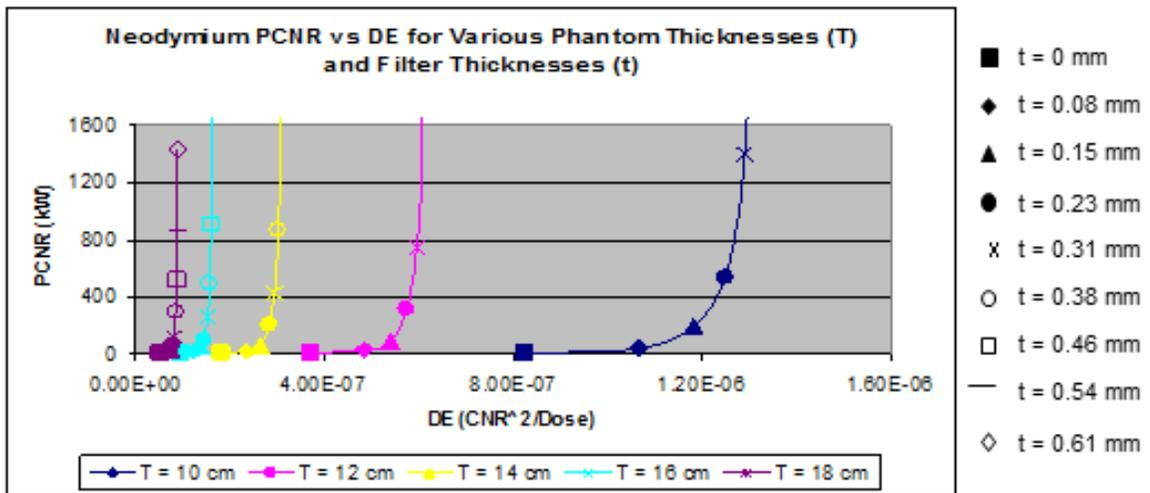
Figure 7.5: Power required to obtain the CNR of a 50 kVp beam as a function of dose efficiency. Each point of each curve represents a different filter thickness.
