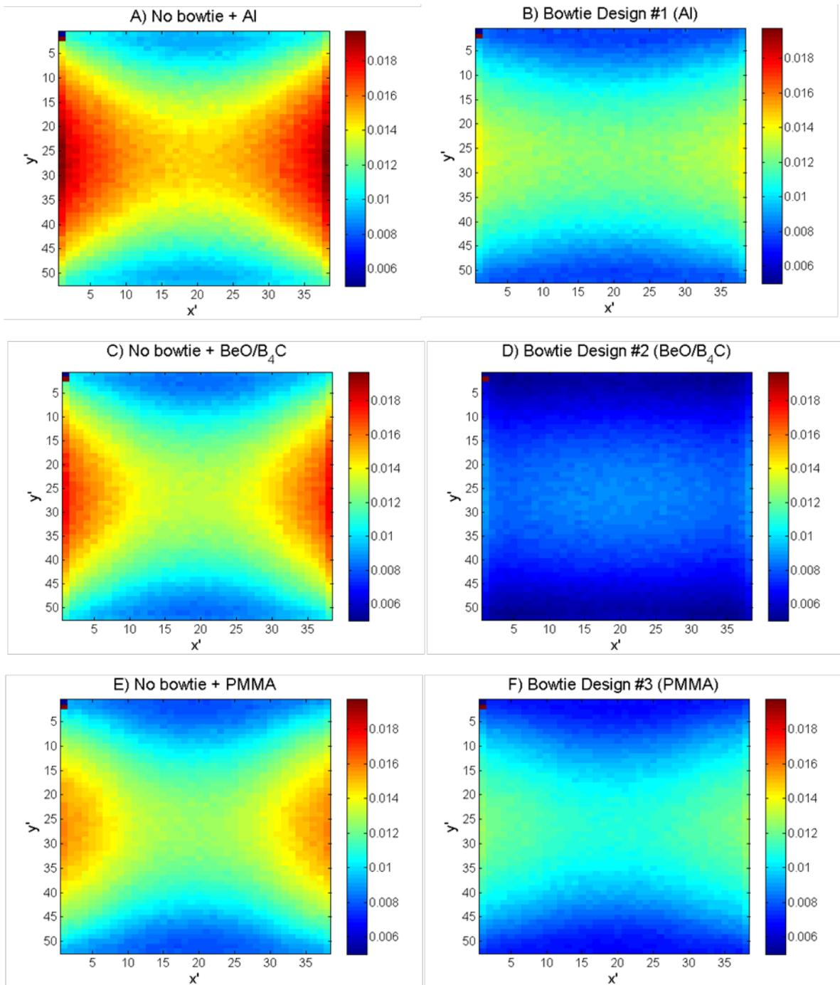
Figure 5.12: Scatter distribution using the SOCR metric for the three bowtie filter types using a 18 cm diameter breast phantom and a tube voltage of 50 kVp. A, C, E show the scatter distributions with no-bowtie filter, but include the constant thickness base from the bowtie filter so that a valid comparison between the two cases can be made. The variables  $x'$  and  $y'$  represent the bin number of the re-binned scatter image used to compute the SOCR.
