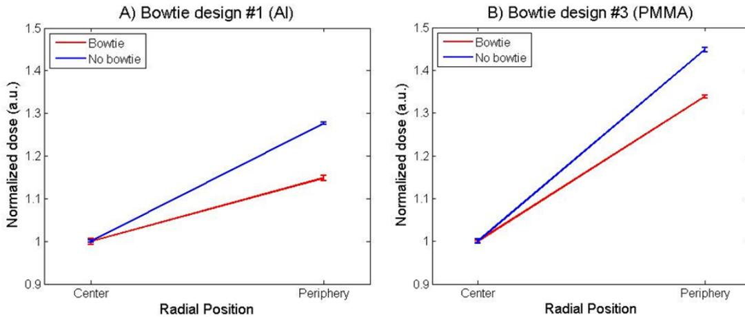
Figure 6.13: Experimentally measured dose distribution for the bowtie and no-bowtie filter case using (A) bowtie design #1 (Al) or 3.5 mm added Al filtration, and (B) bowtie design #3 (PMMA) or 3.5 mm added PMMA filtration.
