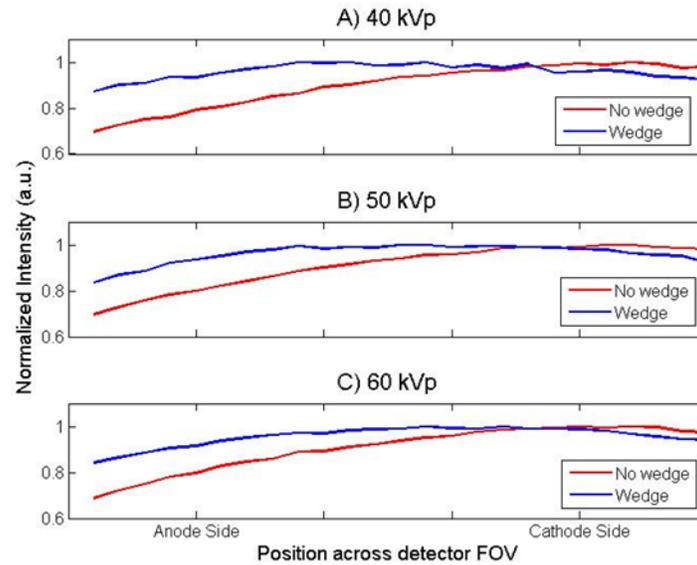
Figure 6.6: Air kerma measurements with and without a Teflon wedge filter to account for the heel effect. The values are normalized to the maximum intensity value. Measurements were acquired at (A) 40 kVp, (B) 50 kVp, and (C) 60 kVp.
