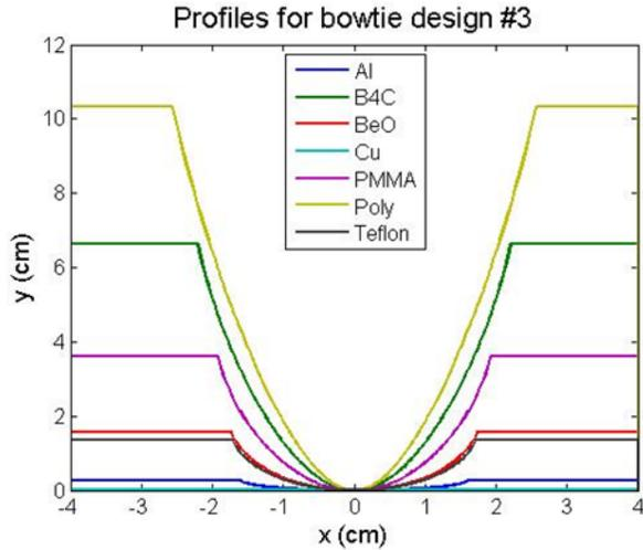
Figure 4.4: Cross section profile for bowtie design #3 using seven different investigated materials.
