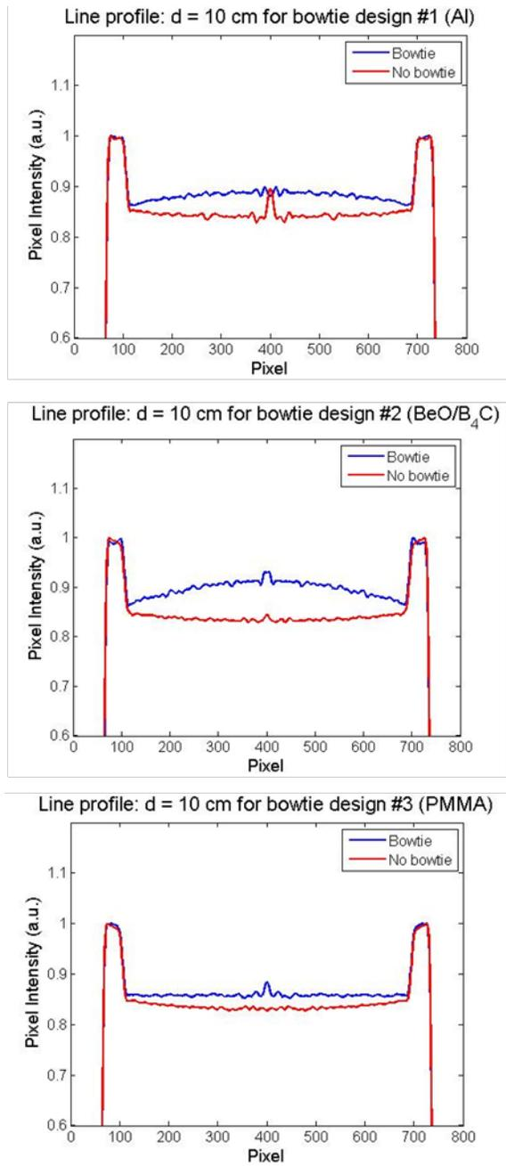
Figure 3.11: Line profiles through the center of the 10-cm phantom, plotted for bowtie design #1 (Al) (top), bowtie design #2 (BeO/B<sub>4</sub>C) (center), and bowtie design #3 (PMMA) (bottom).
