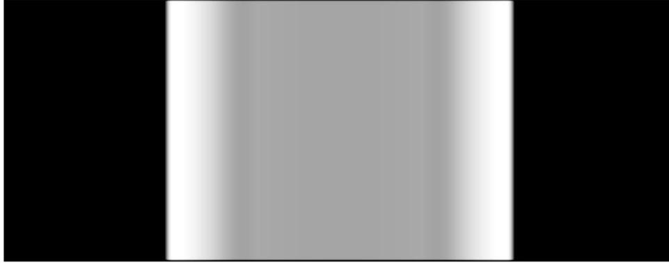
Figure 6.5: Interpolated estimation of the scatter image using the radial basis function in Matlab. This scatter estimate was for a 10 cm diameter phantom with bowtie design #1 (A1).
