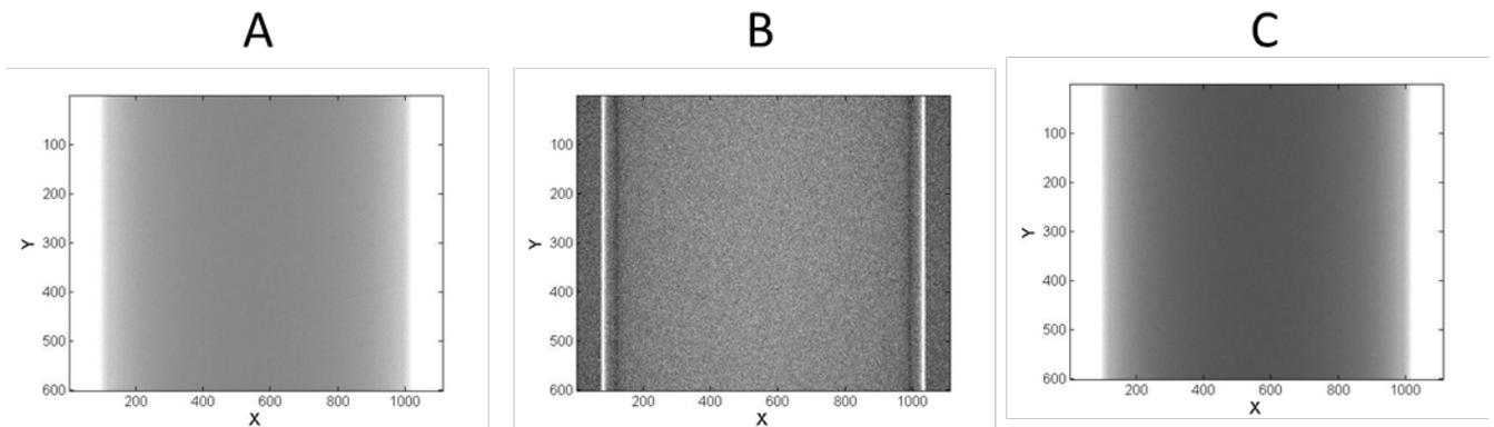
Figure 3.17: Projection views of the 14-cm phantom with (A) bowtie design #1, (B) bowtie design #2, and (C) bowtie design #3. Due to the extension of the bowtie filter at the maximum thickness, the signal intensity in the projection view beyond the phantom for bowtie design #2 is the same as the intensity within the phantom. This is another validation of the bowtie filter design.
