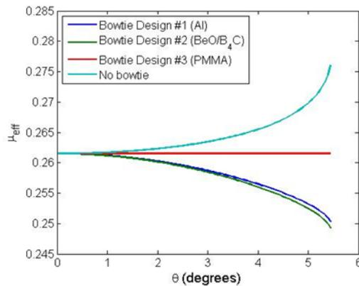
Figure 3.5: Calculated effective attenuation coefficient for all bowtie filters and the no-bowtie filter case.
