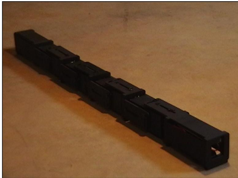
**Figure 3.31:** R2G2: Prototype of the Snake-Inspired Robot Design
