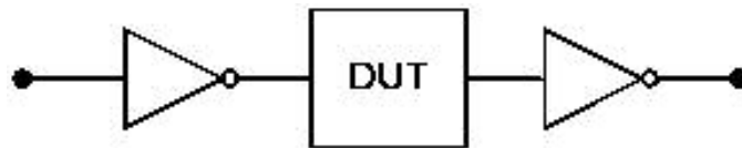
Figure 10A block diagram of a device under test with input and output inverter buffer stages.
