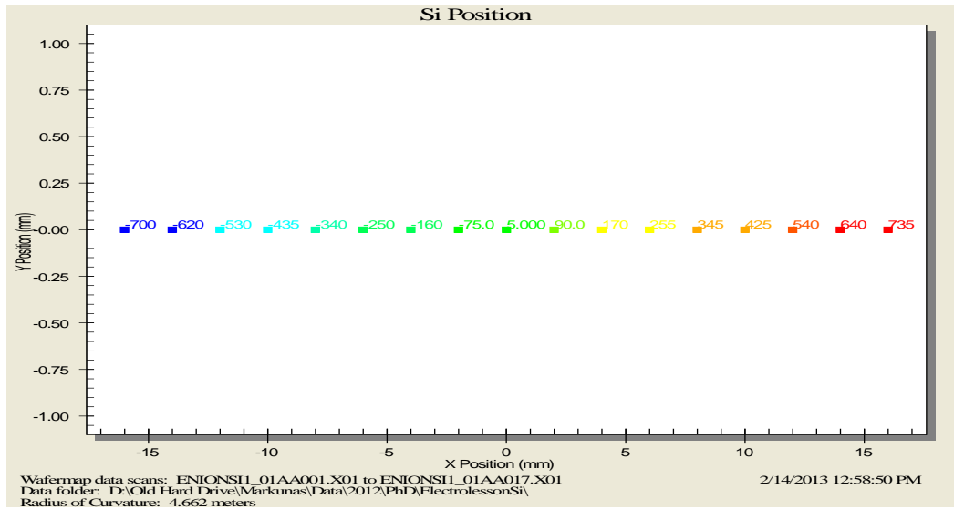
Figure 5.15: Si (400) peak location map used to generate a value for R.
