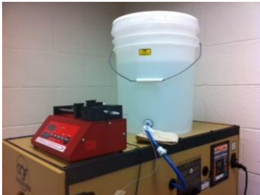
Figure 5.2 Speed adjustable syringe pump system. The pump was connected to a polyethylene tubing infusion line and fitted to a 0.5-mL syringe. A 27-gauge blunted needle was inserted into the chorio-allantoic compartment, secured to the egg shell with glue and connected to the polyethylene infusion line.
