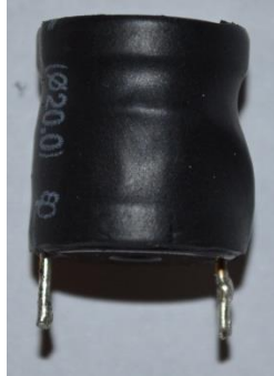
Figure 2: External View of Inductor
