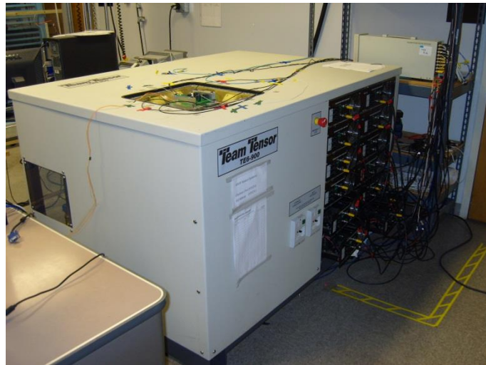
Figure 14: TEAM TENSOR TE6-900 Shaker Table
