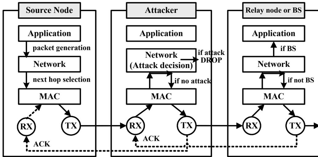
Figure 3.4: Implementation of packet drop attacks models in the OPNET Modeler. When an attacker receives a data packet from a node, the attacker sends an ACK message back to the sender, and then decides whether it drops the data packet based on a pre-defined attack rate.
