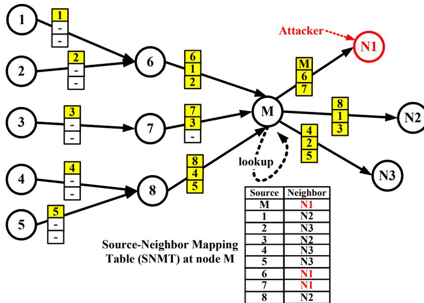
Figure 5.5: Our prevention routing algorithm against a selective forwarding-based DoS attacker (node N1) when the beta trust model is used with  $\theta_T = 0.7$ .
