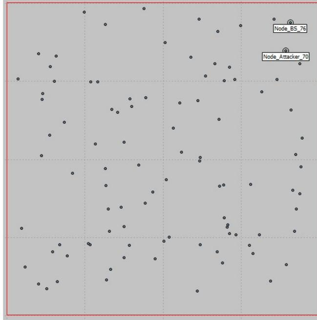
Figure 5.7: A WSN topology in our simulations. One hundred sensors are deployed in a 2km×2km area randomly
