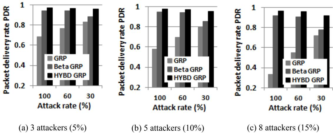
Figure 3.16: Packet delivery rate  $PDR$  (Multiple attackers). Our Hybrid GRP has the highest  $PDR$  among three routing algorithms (GRP, Beta GRP, and Hybrid GRP).
