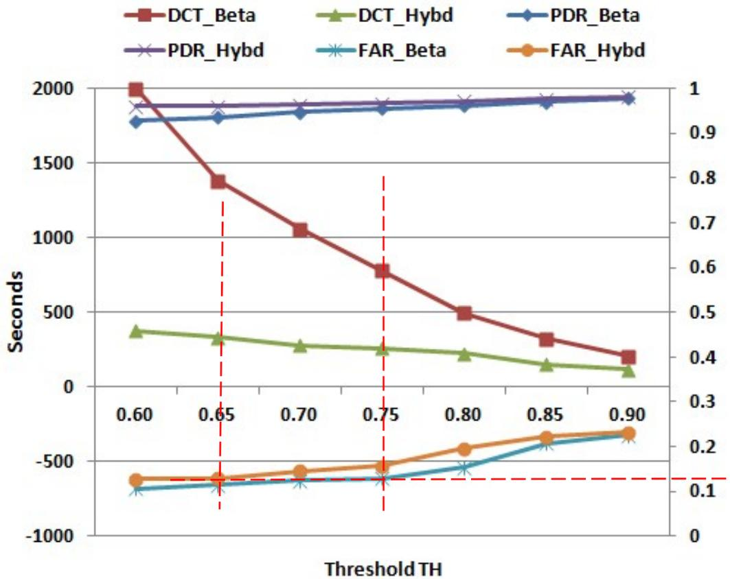
Figure A.1: *DCT* (left Y-axis), *PDR* and *FAR* (right Y-axis) for Hybrid GRP and Beta GRP with different trust threshold values (X-axis) when attacking rate is 60%.
