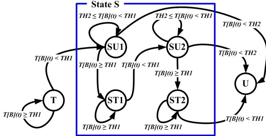
Figure 4.7: The multi-state trust mechanism with two recovery chances (recovery chance  $r=2$ ).
