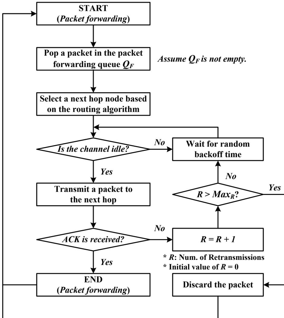
Figure 2.1: Simplified packet forwarding procedure in a WSN.
