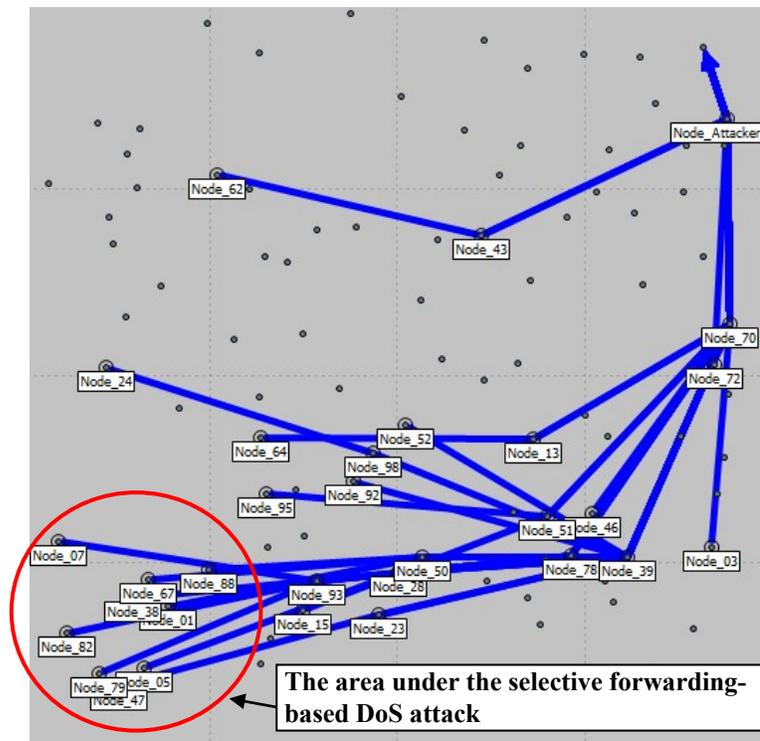
Figure 5.8: 30 potential victim source nodes and their routing paths to the BS when Beta GRP is used. The circle is the physical area under the selective forwarding-based DoS attack.
