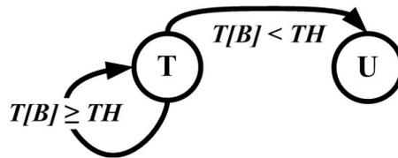
Figure 4.2: The 2-state finite state machine representation of current trust models. In this 2-state finite state machine, a U-node cannot change to a T-node.
