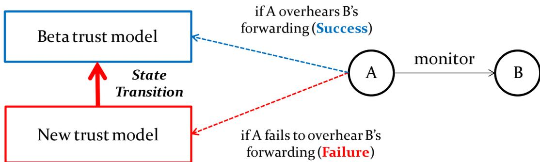
Figure 3.2: Hybrid trust model in node A. For each observation on node B's behavior, when A observes that B forwards A's packet successfully, A increases B's trust value by using the beta trust model. Otherwise, A decreases B's trust value by using the new trust model based on the number of consecutive drops.
