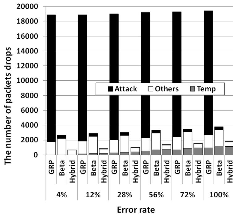
Figure 3.18: The number of packet drops at various error rates when the error period is set to be 1,200 seconds. Our hybrid trust model significantly reduces the packet drop rate of a routing even in a WSN with various error rates and error periods
