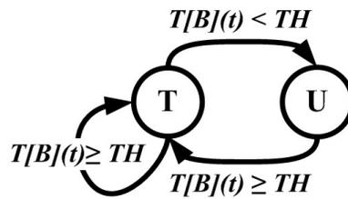
Figure 4.4: 2-state trust mechanism with a recovery transition. A U-node can change to a T-node unlimitedly when the recovery condition is satisfied.
