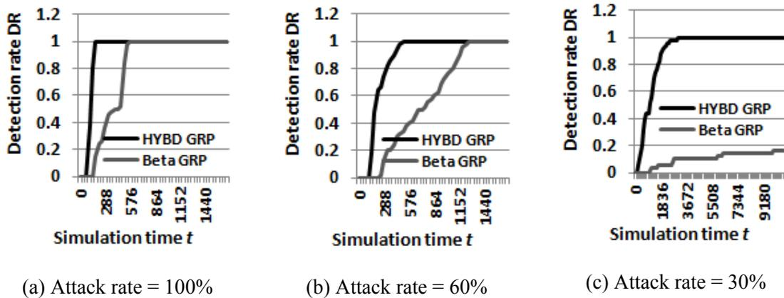
Figure 3.8: Detection rate *DR* when  $TH = 0.7$  (Single attacker). The difference of *DRs* shows the difference of attack detection accuracy of two trust models (Beta and hybrid trust models).
