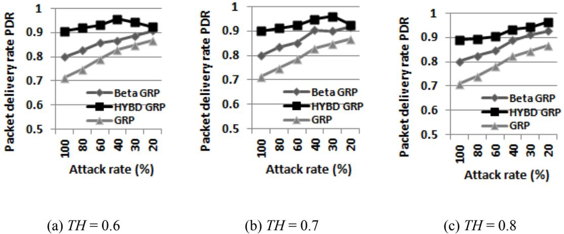
Figure 3.9: Packet delivery rate  $PDR$  (Single attacker). Our Hybrid GRP has the highest  $PDR$  among three routing algorithms (GRP, Beta GRP, and Hybrid GRP) and can deliver at least more than 89% of packets to the BS in all simulation setups.
