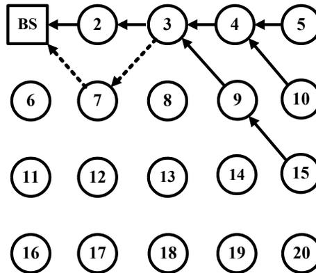
Figure 4.1: GPSR (Solid lines) and trust-based GPSR (Dotted lines). When node 2 drops many packets from node 3, a trust-based routing protocol will find a new routing path (Dotted lines) to avoid node 2.
