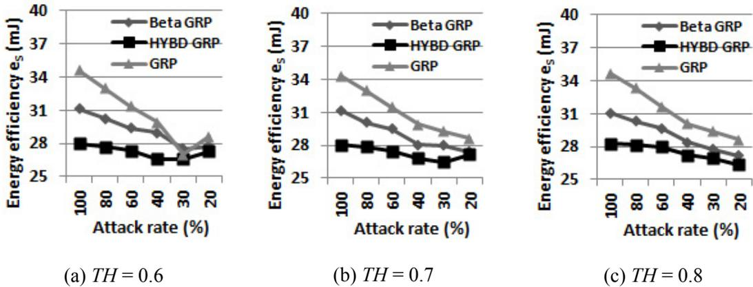
Figure 3.11: Energy efficiency  $e_S$ . (Single attacker). Our Hybrid GRP consumes the least energy to deliver a packet to the BS among three routing algorithms (GRP, Beta GRP, and Hybrid GRP).
