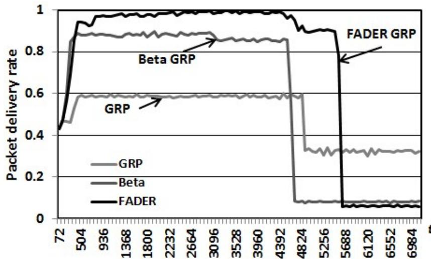
Figure 4.10: Packet delivery rate under two blackhole attackers when  $p = 8\%$ . From bottom to top around time  $t = 1,800$ s: GRP, Beta GRP, and FADER.
