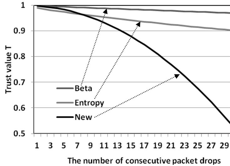
Figure 3.3: New trust model in the presence of consecutive packet drops. After 30 consecutive packet drops, the trust value in the new trust model is very low (i.e.,  $T_{New} \approx 0.534$ ) while the trust values in the beta trust model and entropy trust model are still very high (i.e.,  $T_{Beta} \approx 0.969$  and  $T_{Entr}^* \approx 0.902$ ).
