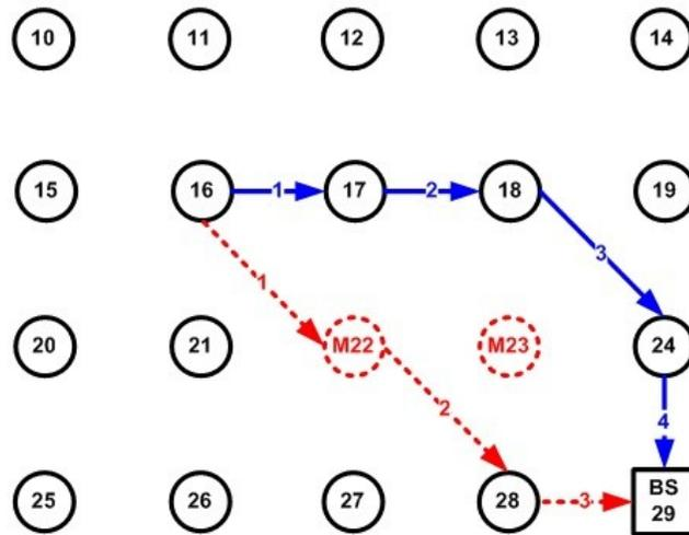
Figure 2.5: GPSR (Dotted lines) and Trust-based GPSR (Solid lines). In the presence of inside packet drop attackers (nodes M22 and M23), the trust-based GPSR finds a trustful routing path ( $16 \rightarrow 17 \rightarrow 18 \rightarrow 24 \rightarrow BS29$ ) to the BS by avoiding malicious nodes.
