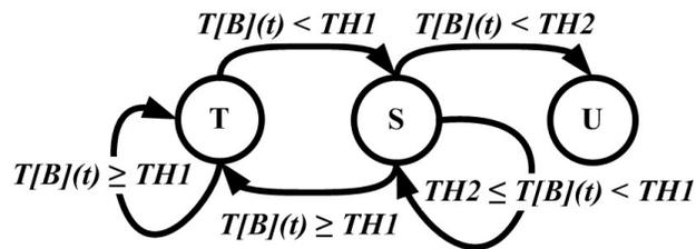
Figure 4.5: 3-state trust mechanism with a recovery transition. An S-node can change to a T-node, but a U-node cannot change to a T-node or a S-node.
