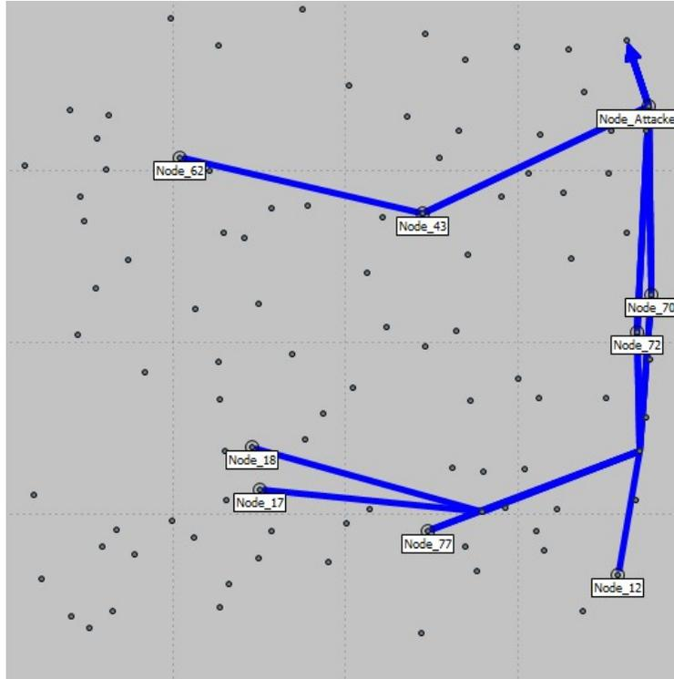
Figure 5.9: 8 potential victim source nodes and their routing paths to the BS when our prevention routing algorithm (Beta GRP-P) is used.
