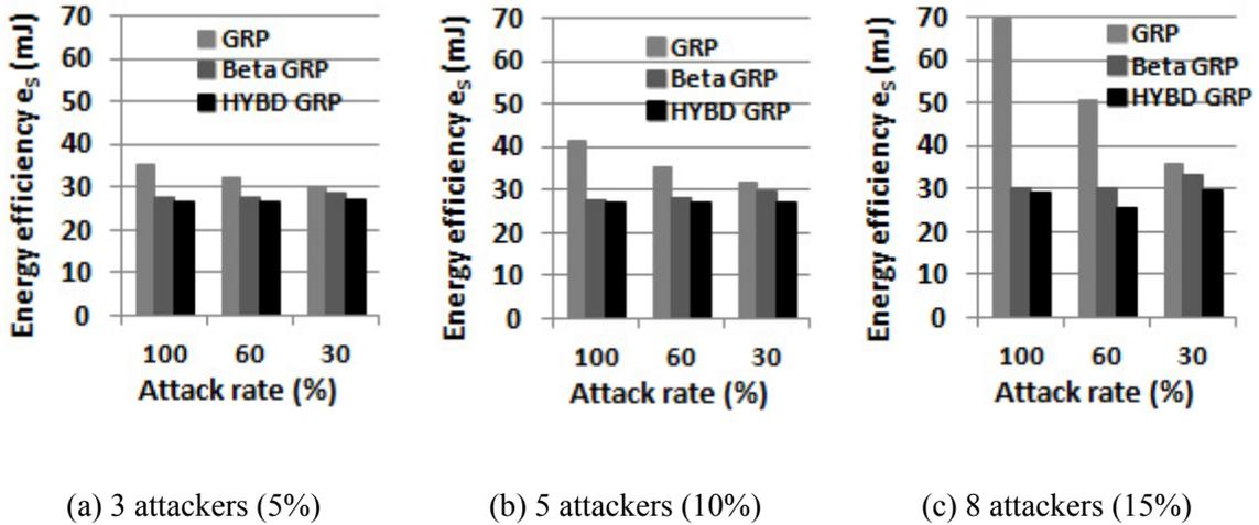
Figure 3.17: Energy efficiency  $e_S$  (Multiple attackers). Our Hybrid GRP has the least  $e_S$  among three routing algorithms (GRP, Beta GRP, and Hybrid GRP).
