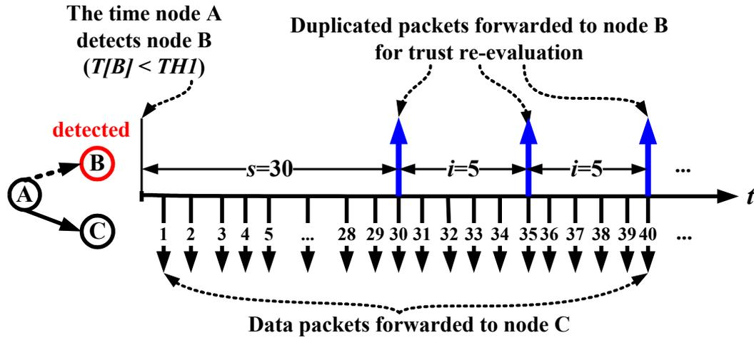
Figure 4.6: Our trust re-evaluation method based on a random sequence with  $s = 30$  and  $i = 5$ . Node A will duplicate its 30th packet for the first time after node A detects node B as an untrustworthy node and send that packet to B for trust re-evaluation. After that, A will duplicate every fifth packet (35th, 40th, 45th, ...) and send it to B until the trust re-evaluation is terminated.
