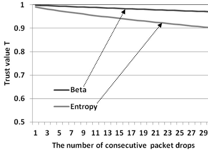
Figure 3.1: Beta and entropy trust models in the presence of consecutive packet drops. Even after 30 consecutive packet drops, the trust values in the beta trust model and the entropy trust model are still very high (i.e.,  $T_{Beta} \approx 0.969$  and  $T_{Entr}^* \approx 0.902$ ).
