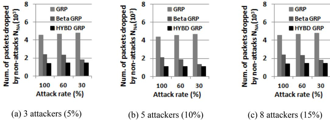
Figure 3.15: The number of packet drops due to non-attacks  $N_{NA}$  (Multiple attackers). Our Hybrid GRP has the least  $N_{NA}$  among three routing algorithms (GRP, Beta GRP, and Hybrid GRP).
