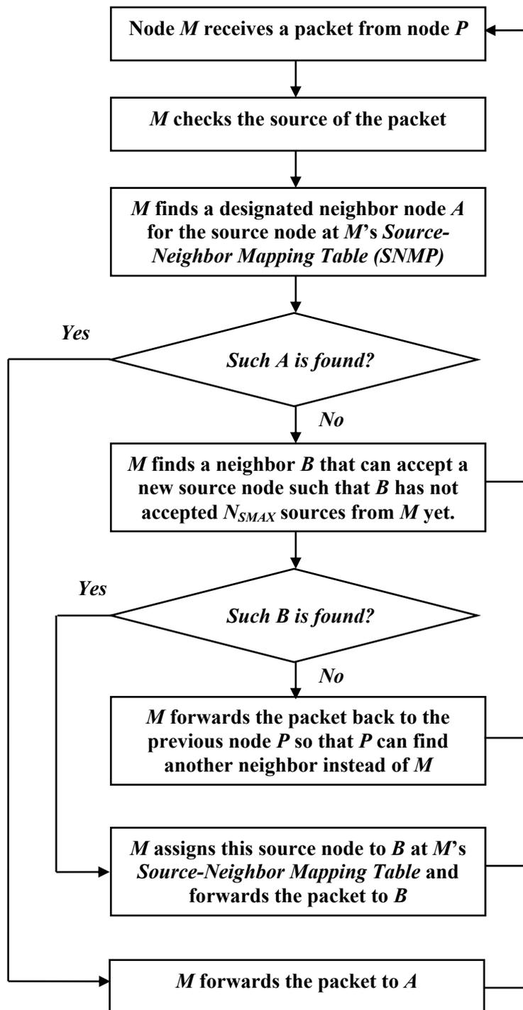
Figure 5.6: The flow chart of a trust-based routing algorithm with our prevention method to prevent the selective forwarding-based DoS attack.
