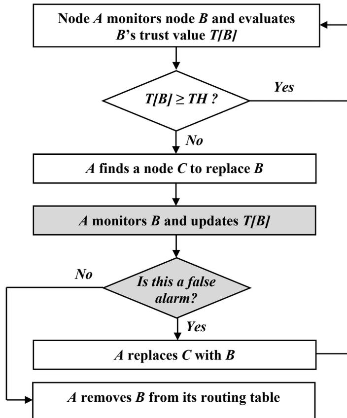
Figure 4.3: Outline of FADER: False Alarm DEtection and Recovery.
