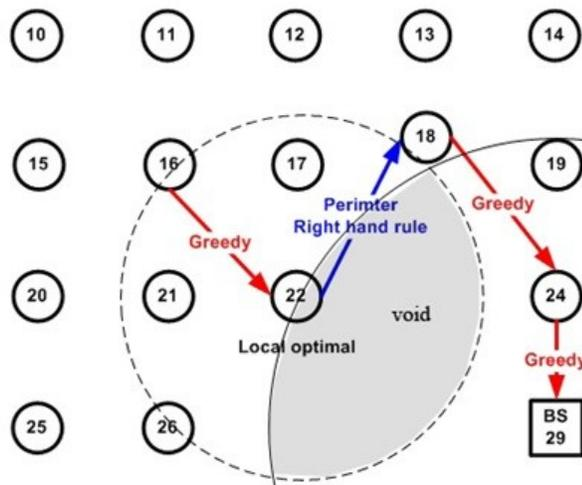
Figure 2.4: Greedy forwarding and perimeter forwarding in the GPSR. Greedy forwarding finds a neighbor closest to the BS. When greedy forwarding fails in finding such a neighbor (e.g., when node 22 meets a *void* or a *hole* in the figure), perimeter forwarding is used to find a path to the BS.
