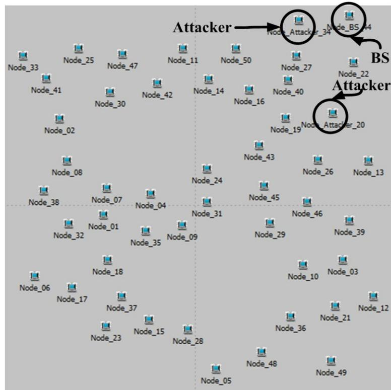
Figure 4.9: The ad hoc WSN with two inside packet drop attackers used in our simulations.
