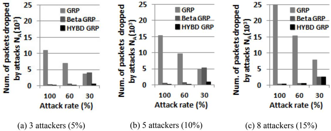
Figure 3.14: The number of packet drops due to attacks  $N_A$  (Multiple attackers). Our Hybrid GRP has the least  $N_A$  among three routing algorithms (GRP, Beta GRP, and Hybrid GRP).
