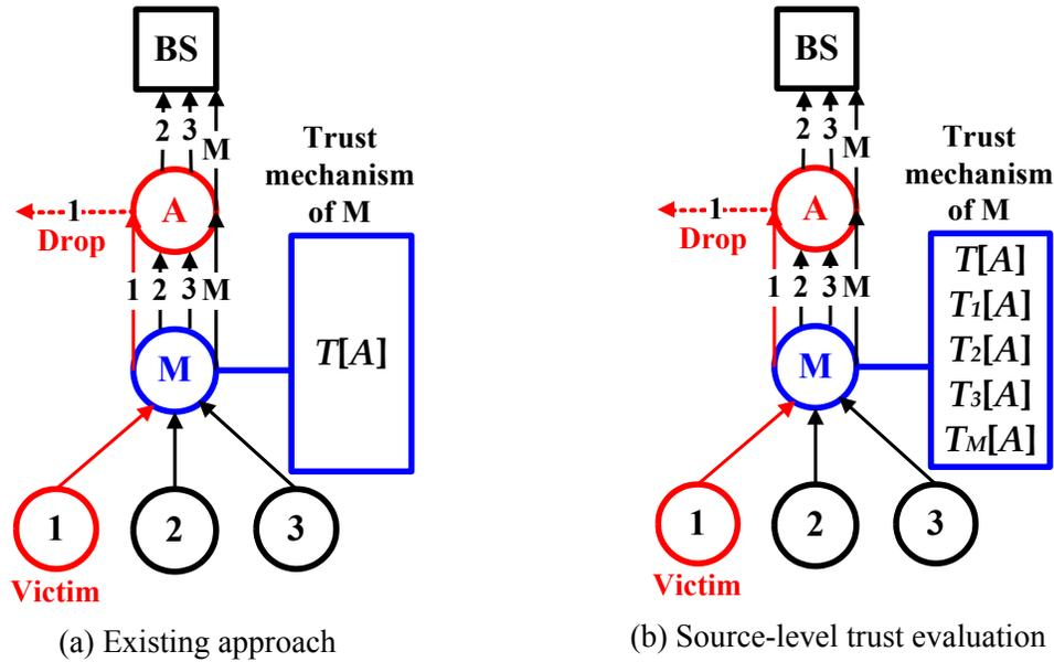
Figure 5.2: Existing trust evaluation approach and proposed approach. In our approach (source-level trust evaluation), M evaluates not only A's overall trust value  $T[A]$  but also A's source-level trust values  $T_i[A]$  to see how much M can trust A in forwarding packets from node  $i$ .
