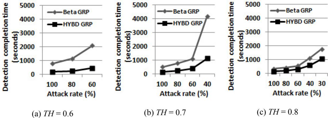
Figure 3.6: Detection completion time *DCT* (Single attacker). Our Hybrid GRP detects an inside packet drop attacker always faster than the Beta GRP in the presence of various attack models.
