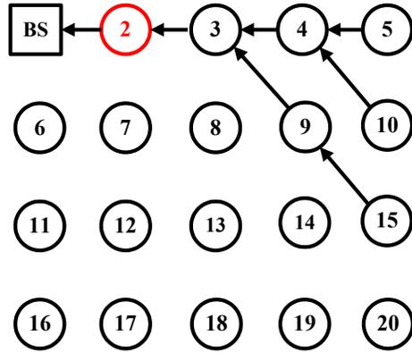
Figure 5.1: Trust-based GPSR in the presence of a selective forwarding-based DoS attacker (node 2).
