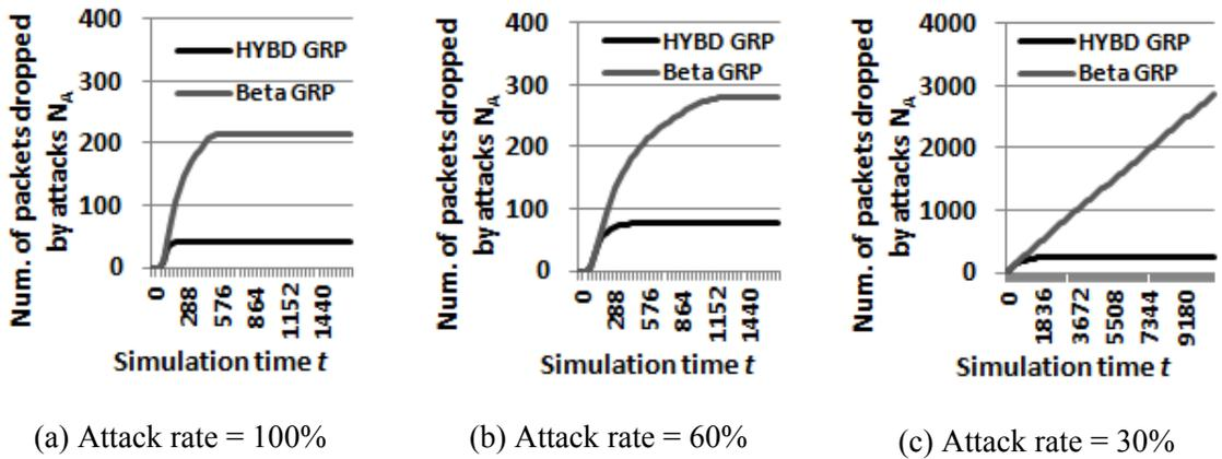
Figure 3.7: The total number of packets dropped due to attacks  $N_A$  when  $TH = 0.7$  (Single attacker). The early detection capability of our hybrid trust model based on consecutive drops significantly reduces the damage to the network due to attacks compared to that of the beta trust model.
