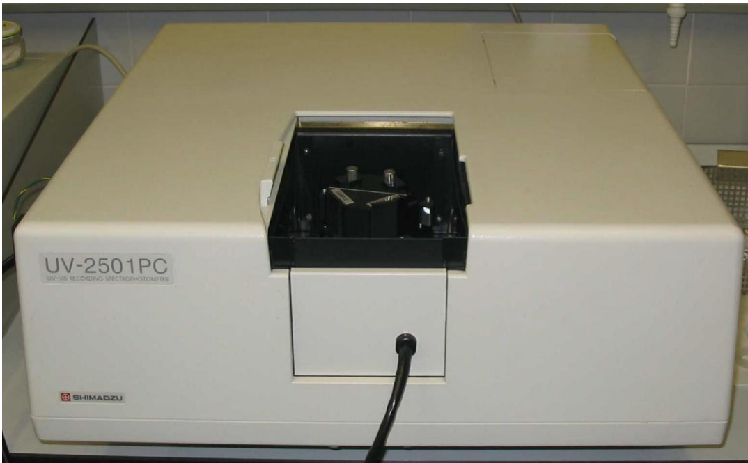
Fig 1.15. Shimadzu UV2501PC UV-vis Spectrophotometer. The working wavelength for this machine is from 200nm to 900nm.
