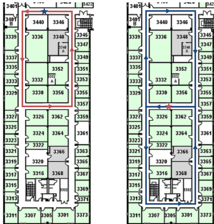
Figure 15- A.V. Williams Wing (3rd Floor) Floor Plan with Robot Path Overlaid (Left: Double Loop, Right: Infinity Loop) [13]
