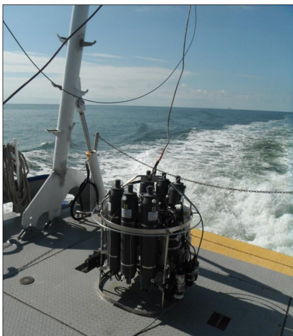
Photo 10. Vertical Profiling Rosette and visible surface oil slick above location of submerged, leading barge.
