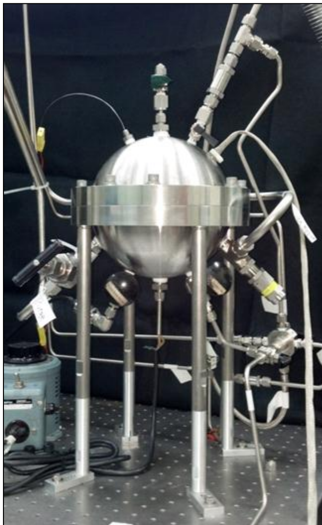
Figure 2: 2 L constant volume combustion chamber used to collect experimental data.
