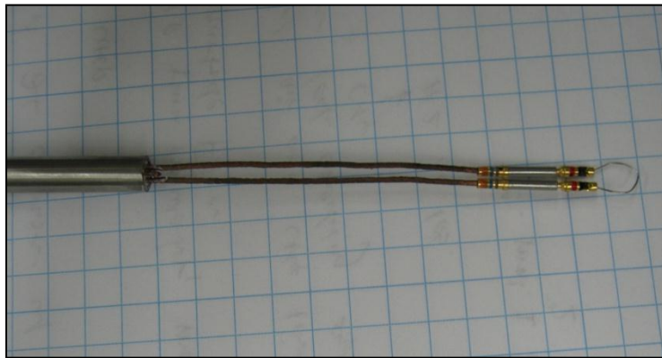
Figure 3: 2L chamber igniter feedthrough with a platinum wire crimped connected.
