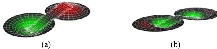
Figure 4-14: Mode shapes obtained by laser Doppler vibrometer measurement for the miniature directional microphone inspired by the fly ear. (a) Rocking mode (9.8 kHz). (b) Bending mode (22.0 kHz).
