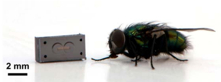
Figure 4-11: A fabricated MEMS directional microphone placed next to a house fly
