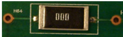
Figure 4.1: FR4 Test board with 2512 Resistors
