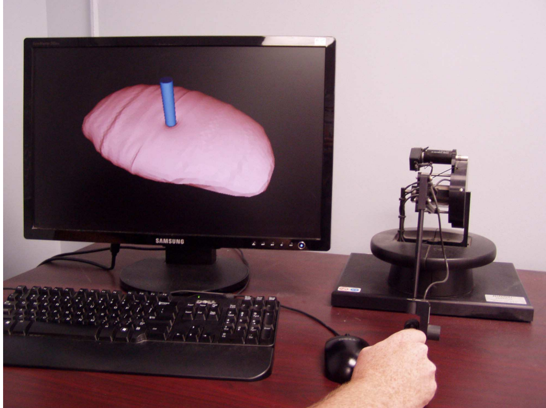
Figure 4.9: Preprocessor based real-time, probing simulator with realistic display and haptic feedback. ©2009 IEEE.
