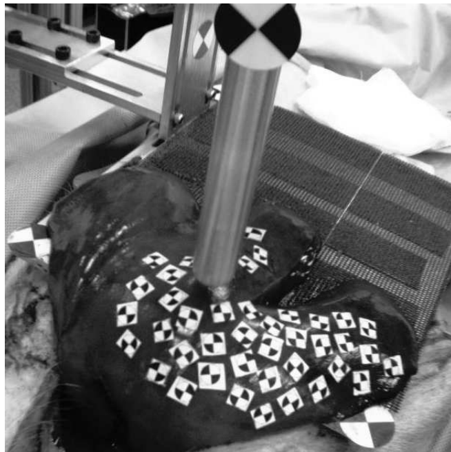
Figure 2.22: Location of markers during one test location in the first pig lab.
