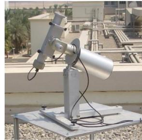
Figure 4: Pyranometer and Pyrhelimeter
