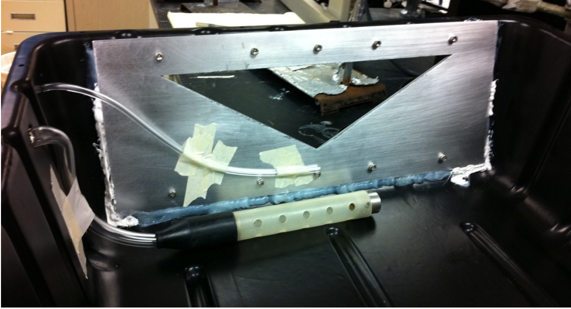
Figure 75. Side of prototype filter tub where effluent exited the tub.
