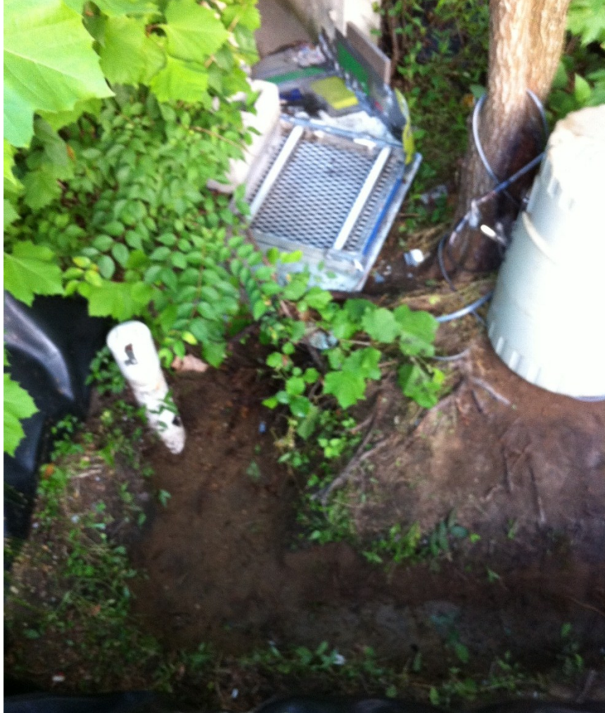
Figure 77. View over the area inside of a bioretention cell where the prototype filter tub and ISCO sampler were placed.
