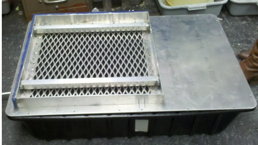
Figure 74. Prototype filter and tub used in-field to collect stormwater effluent.
