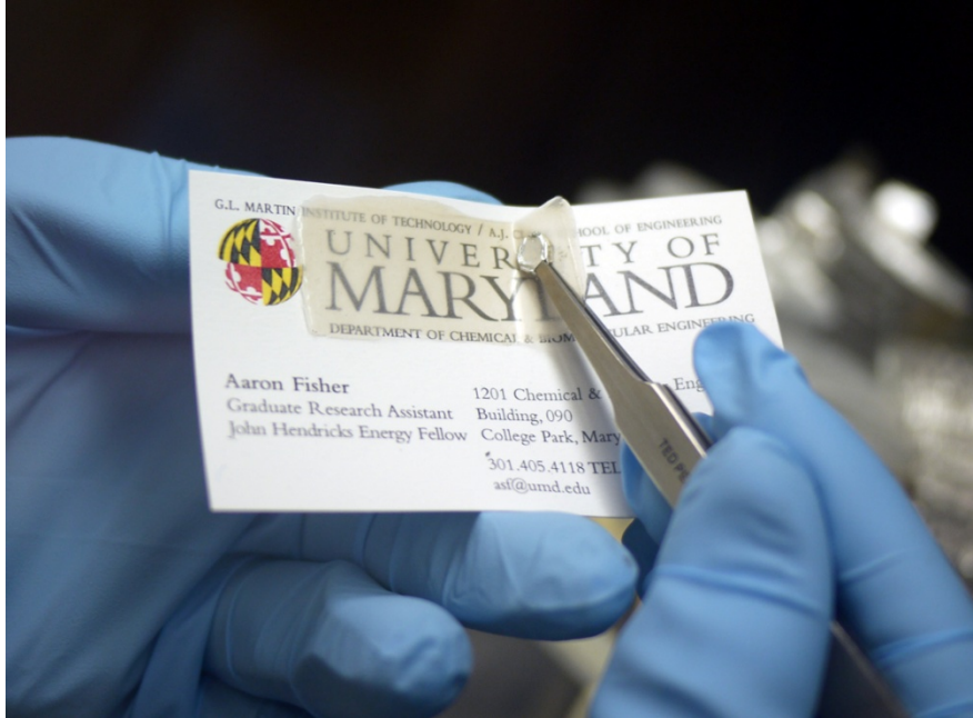
Figure VI-2 Visual image of the solid block copolymer showing the flexible transparent nature of the as-cast film. The film ratio is 20 PEO of the BCP : 1 LiBOB : 0.1 S 2 BOB.
