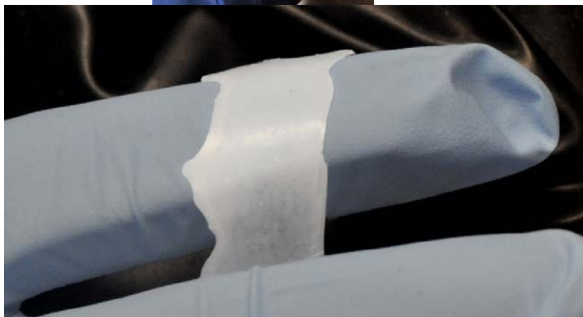
Figure IV-1 Pictures of thin film solid electrolyte in Ar atmosphere. Electrolyte is ~5 cm. x 2cm.
