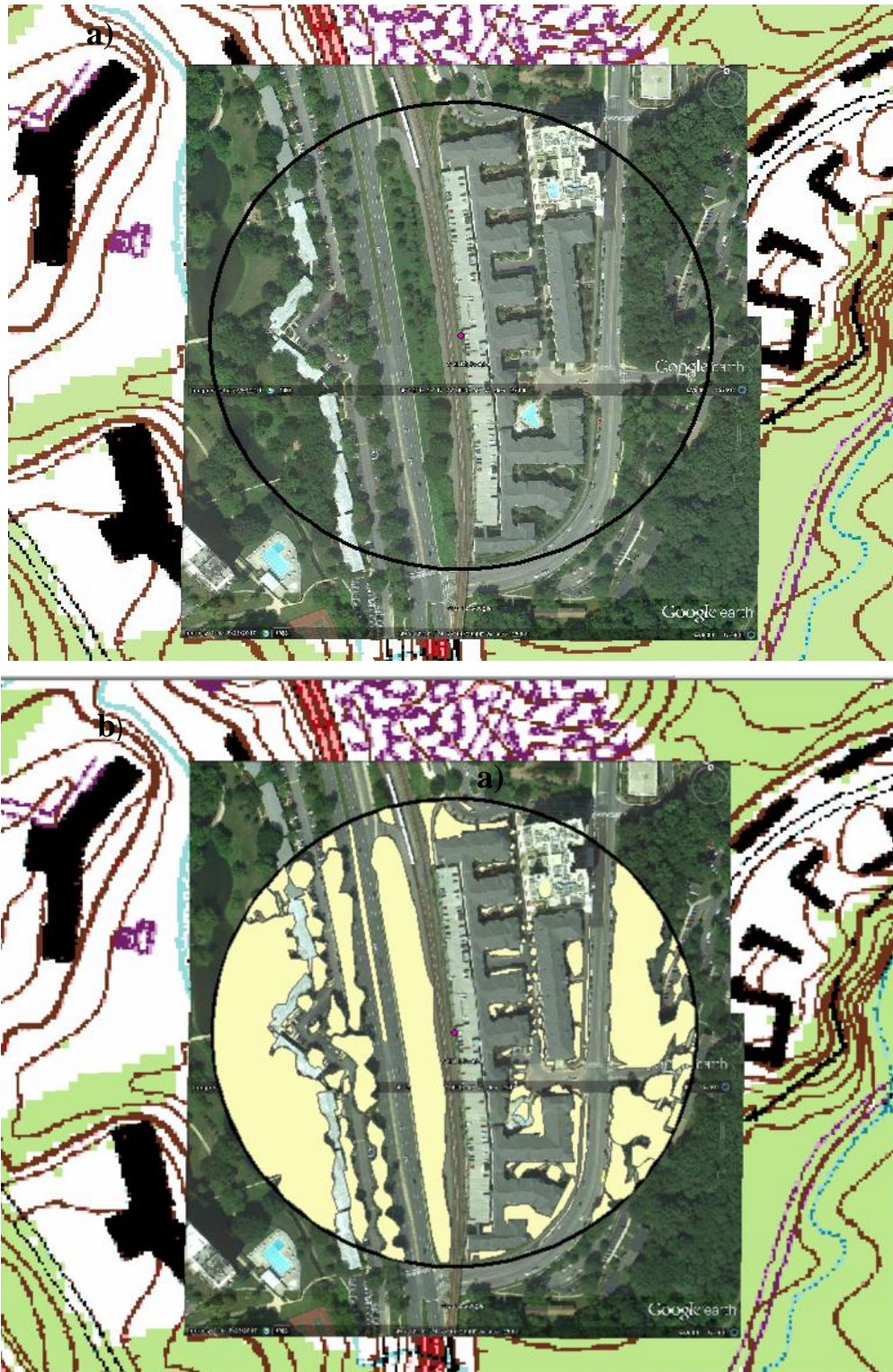
Figure 16. Aerial photograph of site 6 in Rockville, MD georeferenced in ArcMap a) indicates 200m buffer surrounding the site b) “unsealed” surfaces have been outlined and overlaid by yellow polygons using the Editor tool in ArcMap.
