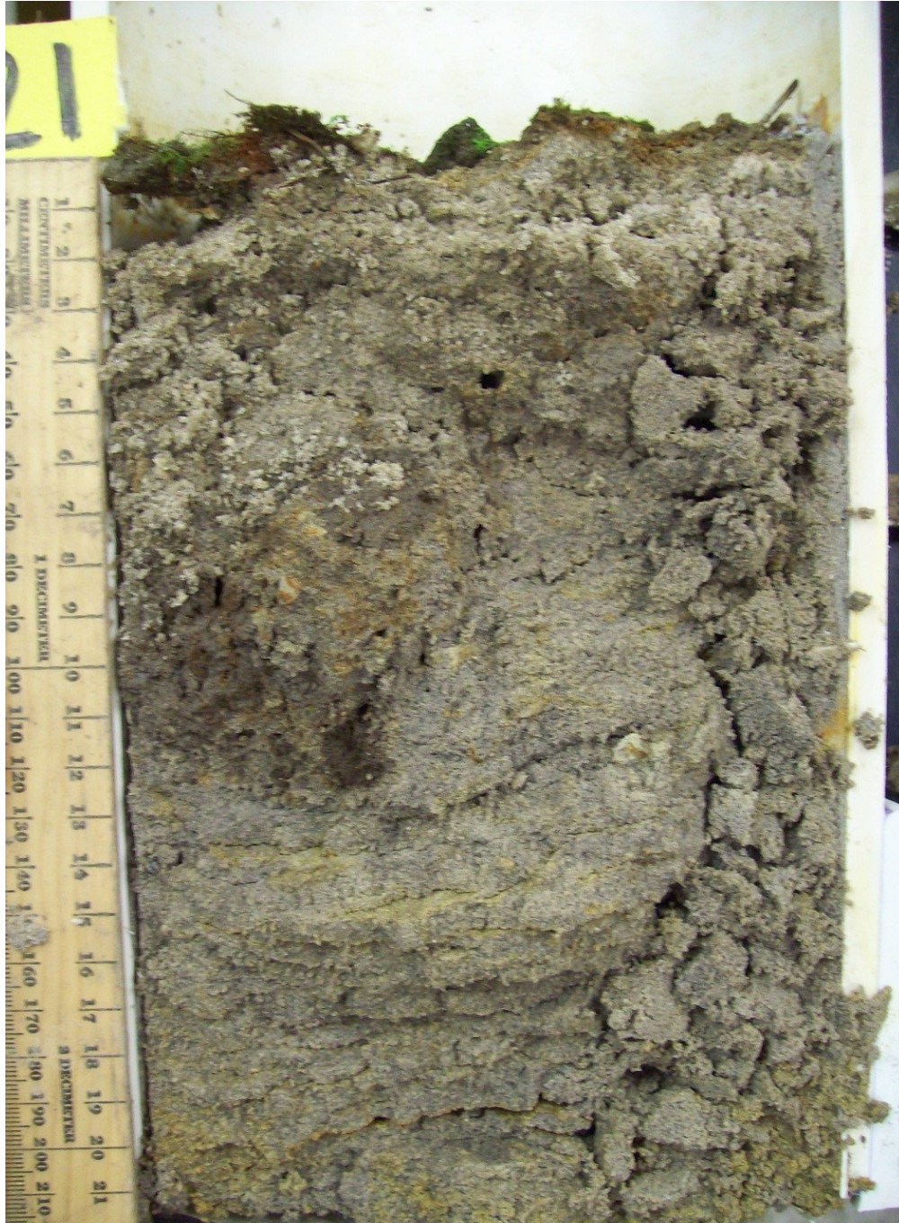
Illustration 3.7. Mesocosm taken 14 days after dredging of ditch and then subjected to experimental treatments. Note platy structure of materials left in place despite dredging. Note the lack of structure and inclusion of A material from colluvium/alluvium which collected at the surface between dredging and mesocosm harvest.
