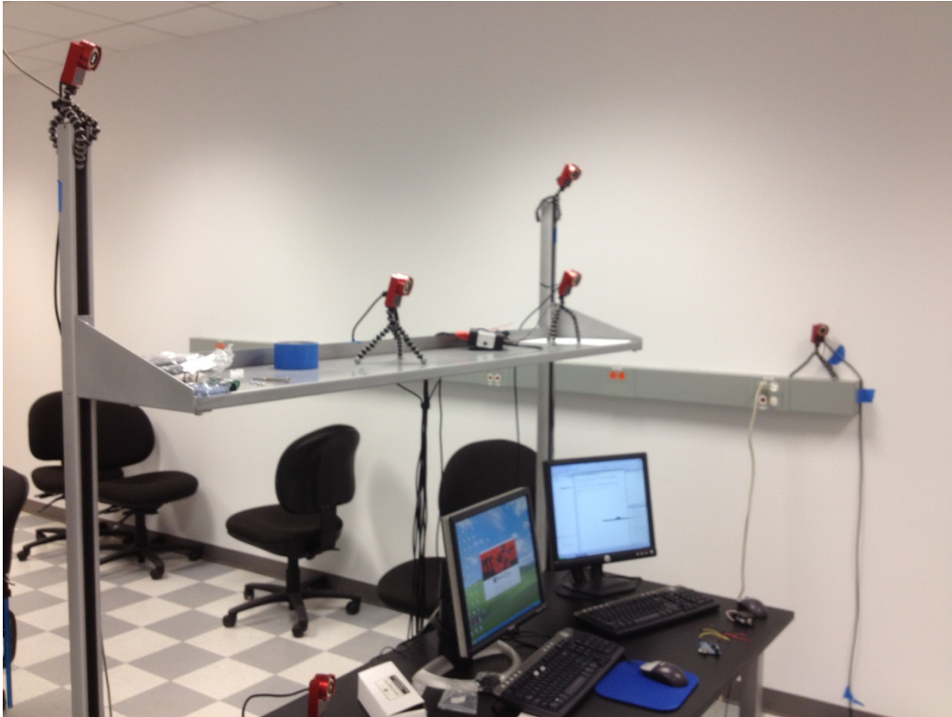
Figure 28 - Experimental array of NaturalPoint OptiTrack cameras
