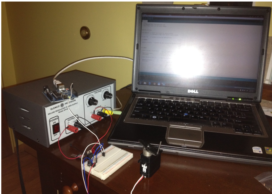
Figure 8 – Equipment setup for servo motor characterization
