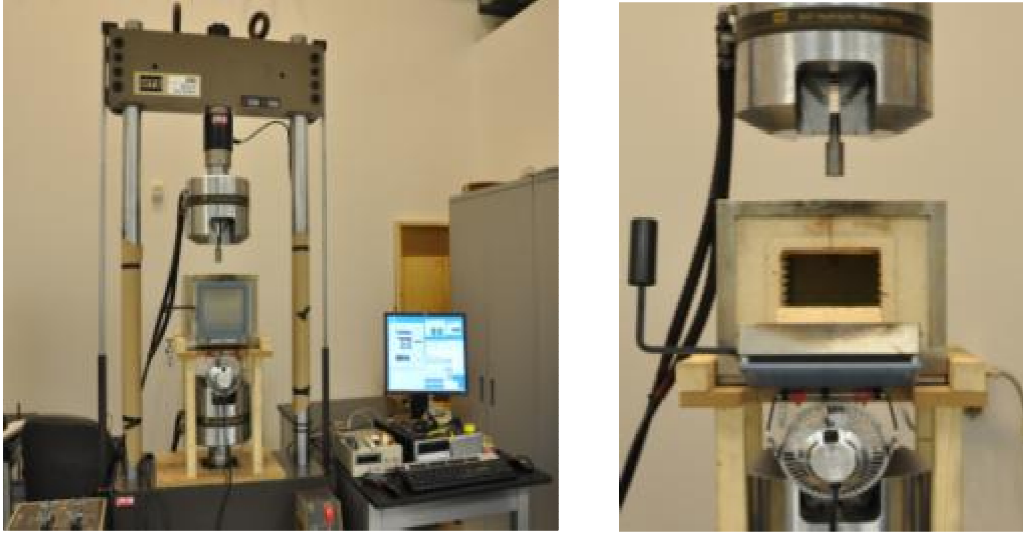
Figure 4.19: MTS-810 Material Test System equipped with creep furnace and data acquisition.
