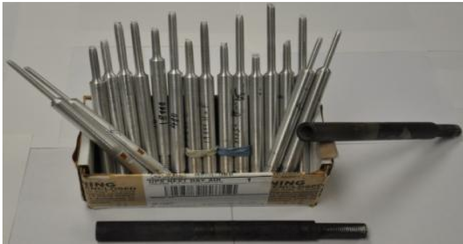
Figure 4.20: Al-7075-T6 used in creep experiments with hardened grip holders
