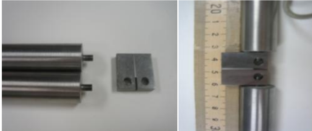
Figure 4.6: X70 carbon steel with top and bottom threaded grips
