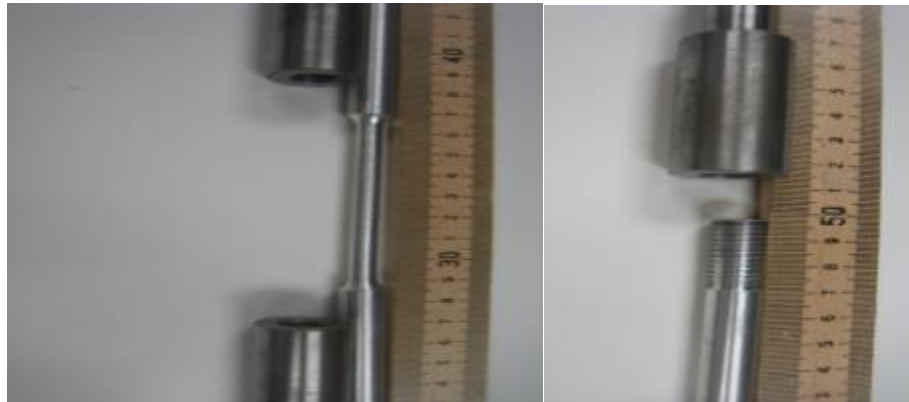
Figure 4.5: Al-sample with two threaded holders (left), in top or bottom view (right)
