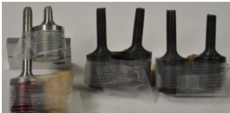
Figure 4.28: Broken sample at room temperature with cup and cone ductile breakage (left) and two X70 carbon steel samples after creep experiment with brittle fracture types (right)
