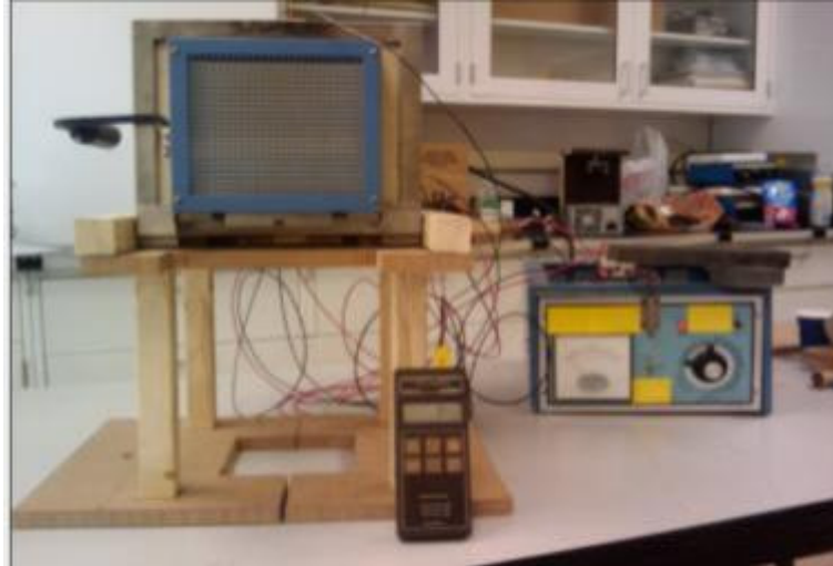
Figure 4.3: The heating chamber for creep experiment during the temperature test before installing in the MTS machine.
