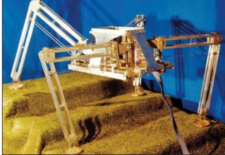
Figure 4 PV-II Climbing Stairs [25]
