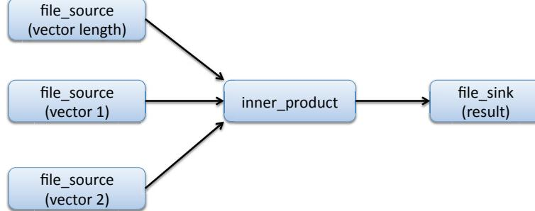
Figure 1: Dataflow graph for the inner product computation example.
