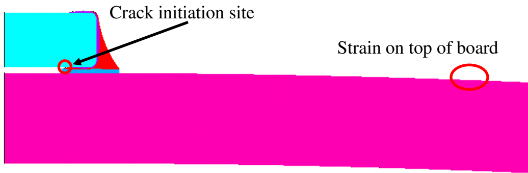
Figure 18. The crack initiation site for flex cracking
