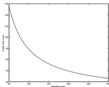
**Fig. 7.** Stereo error analysis
