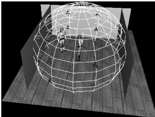
**Fig. 6.** The adjustable mountings allow the cameras to be positioned on a virtual sphere, if so desired.
