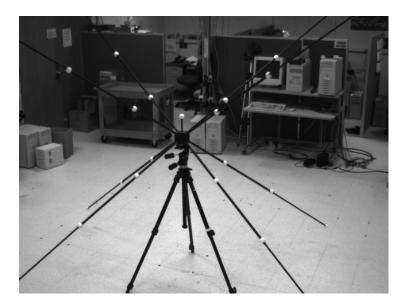
Fig. 9. Peak Performance calibration frame
