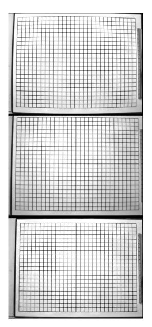
Fig. 8. Lens distortion analysis. Top: Cosmicar 6 mm, Middle: Canon 7.5 mm, Bottom: Schneider 8 mm.
