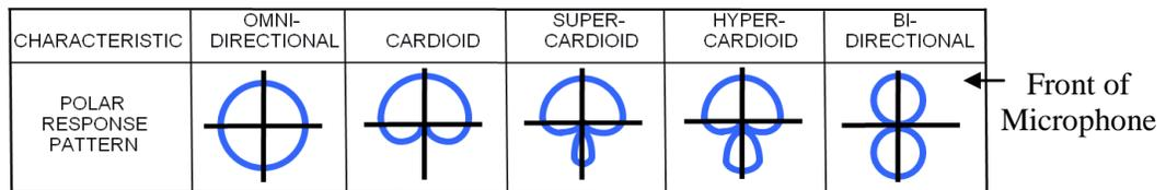
Illustration G-1. Two-dimensional graphical representation of five common polar pattern responses at 1 kHz. The top of each illustration represents the front of the microphone. Simplified from an illustration from Shure Brothers, Inc., used with permission.
