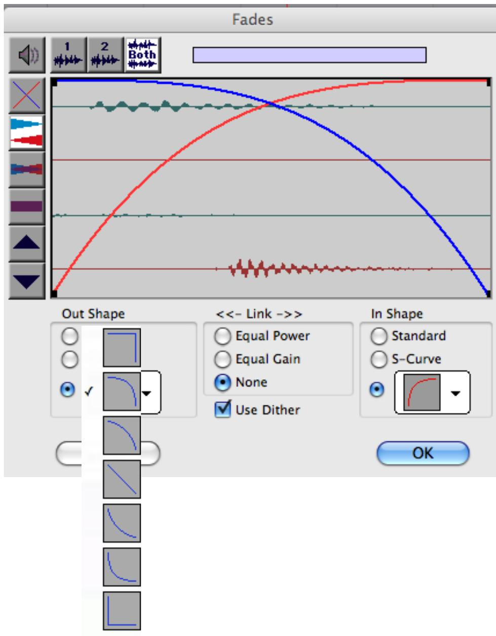
Illustration 5-5. Cross fade screen with pull-down menu and possible curve choices. In shape and out shape have the same possibilities, which one can mix-and-match.
