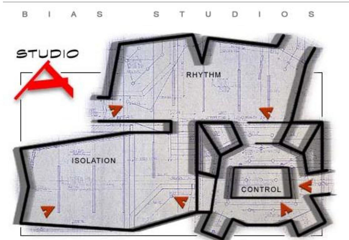
Illustration 4-1. Floor plan of Studio A at Bias Studios. Note in Illustration 4-8 that the floor of the isolation portion of the studio is lower than the rhythm section floor. Floor plan copied from [www.biasrecording.com](http://www.biasrecording.com) and used with permission. Red arrows are hyperlinks active on the website.
