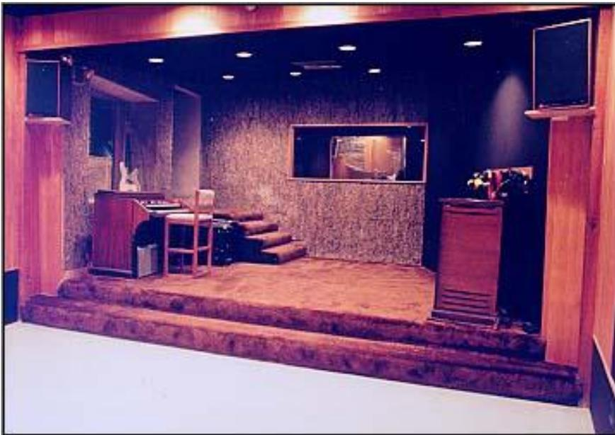
Illustration 4-8. View from the isolation room toward the control room in the back. Note the stairs going up to the upper isolation room for rhythm section. There is a window between the upper and lower isolation rooms.
