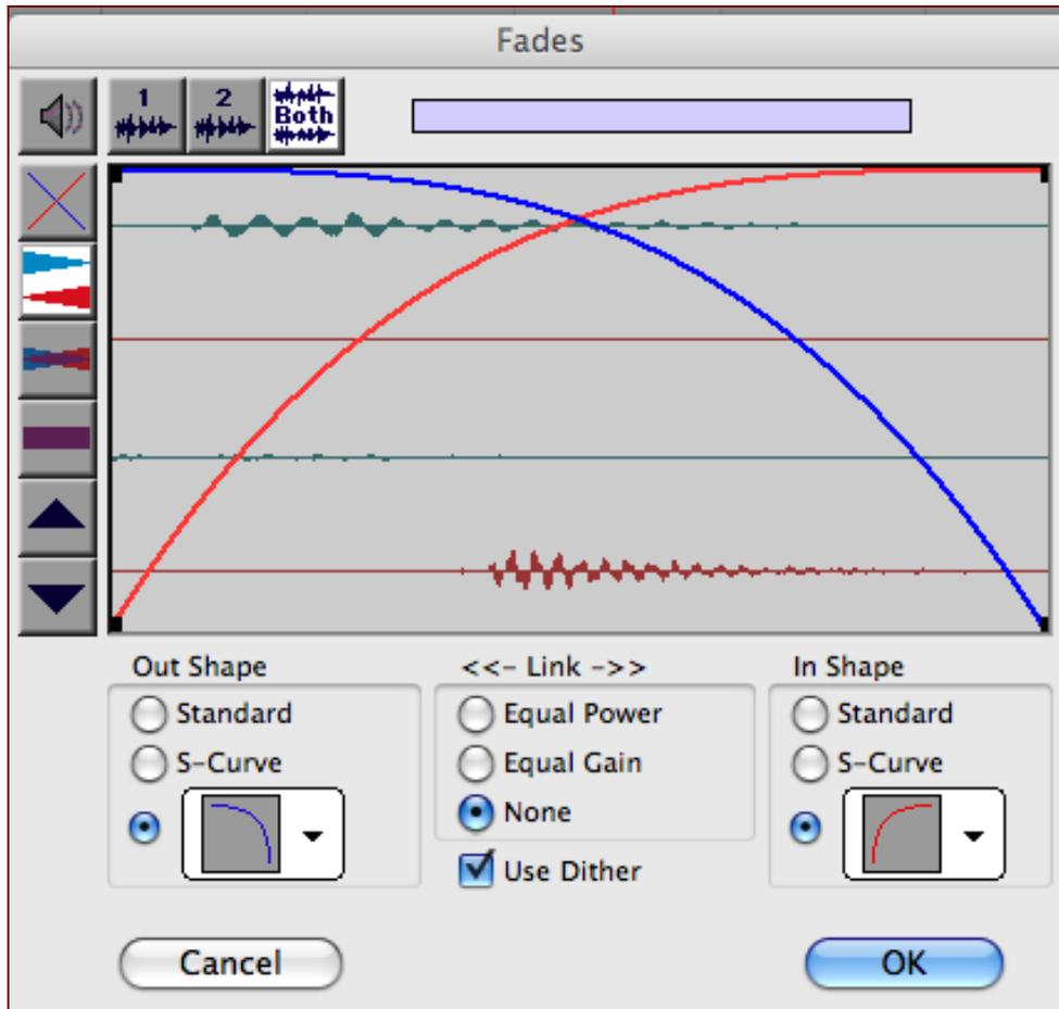
Illustration 5-4. Cross fade curves used for bass, tenor, trombone, and piano. When the link button is used, equal power is for non-phase coherent material, while equal gain is for audio loops and other phase coherent material.<sup>125</sup> See “Dither” in the Glossary.
