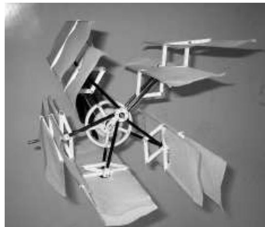
(b) Cyclorotor using the pantograph mechanism.
