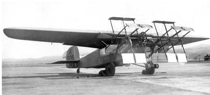
Figure 5.1: **Schroeder cyclogyro built in 1930s [29].**
