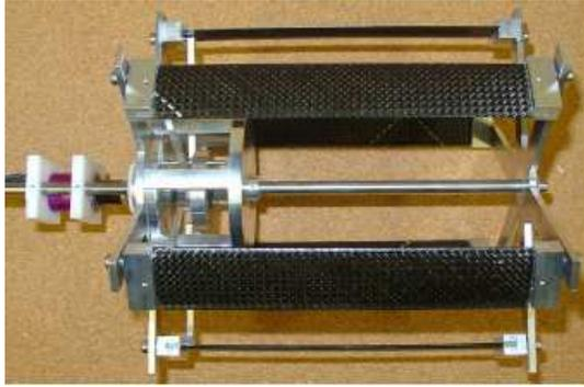
(a) Cyclorotor used for testing.
