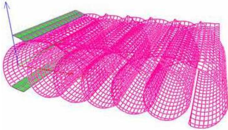
Figure 1.30: **Results from the unsteady vortex lattice analysis on the cyclorotor (National University of Singapore) [60].**
