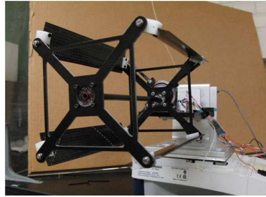
(b) Rotor used on the quad-cyclocopter.
