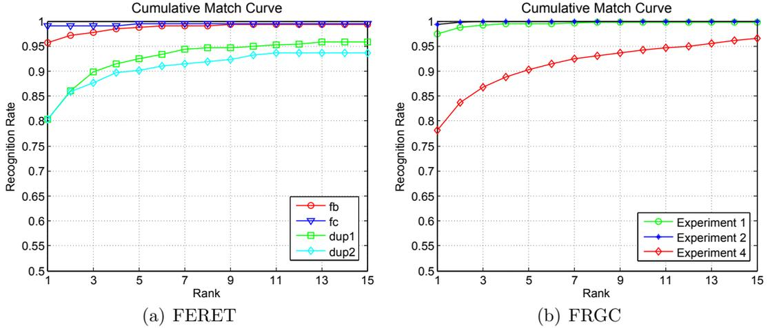
Figure 6.4: The cumulative match curve for the top 15 matches obtained by the one-against-all approach based on PLS regression for FERET and FRGC datasets.
