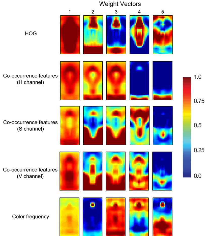
Figure 2.4: Weight vectors for different features within the detection window. Red indicates high importance, blue low (the plots are in the same scale and normalized to interval  $[0, 1]$ ).
