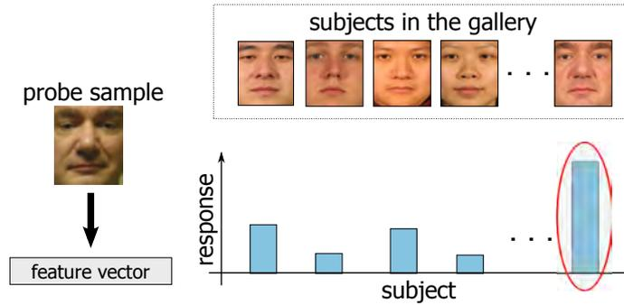
Figure 6.2: One-against-all face identification approach. Matching of a probe sample against the subjects in the gallery. The best match for a given probe sample is the one associated with the PLS model presenting the highest regression response.
