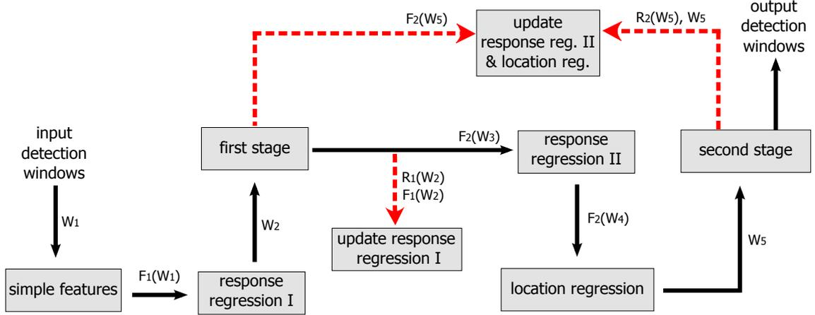
Figure 4.1: Integration of the regression models into the PLS detector. Regression models to estimate the detector’s response, *the response regression I* and *the response regression II*, are added before each stage and a regression to estimate the object location, *the location regression*, is incorporated right before the second stage.
