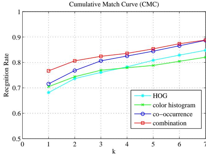
Figure 5.8: Recognition rates obtained by using individual features and combination of all three feature channels for sequence #3.
