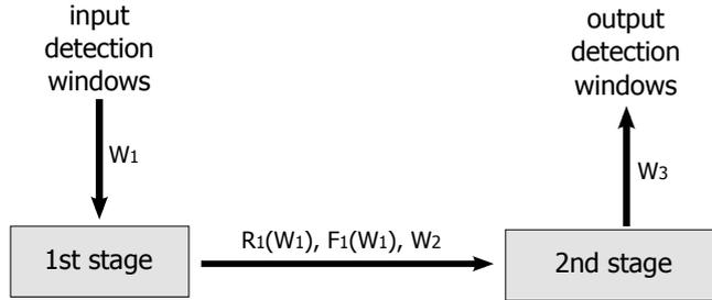
Figure 4.2: Steps of the PLS detector. Given an input set of detection windows,  $\mathbf{W}_1$ , the first stage outputs the windows selected to be considered by the second stage,  $\mathbf{W}_2 \subset \mathbf{W}_1$ , the response and the features for all input detection windows,  $R_1(\mathbf{W}_1)$ ,  $F_1(\mathbf{W}_1)$ , respectively.
