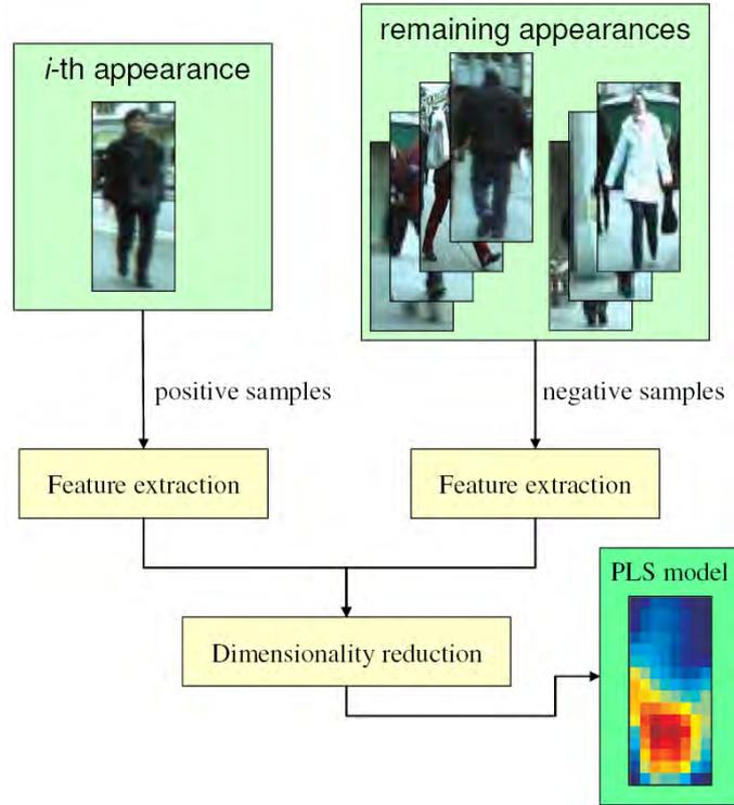
Figure 5.2: Proposed method. For each appearance represented by an image window, features are extracted and PLS is applied to reduce dimensionality using a one-against-all scheme. Afterwards, a simple classifier is used to match new samples to models learned.
