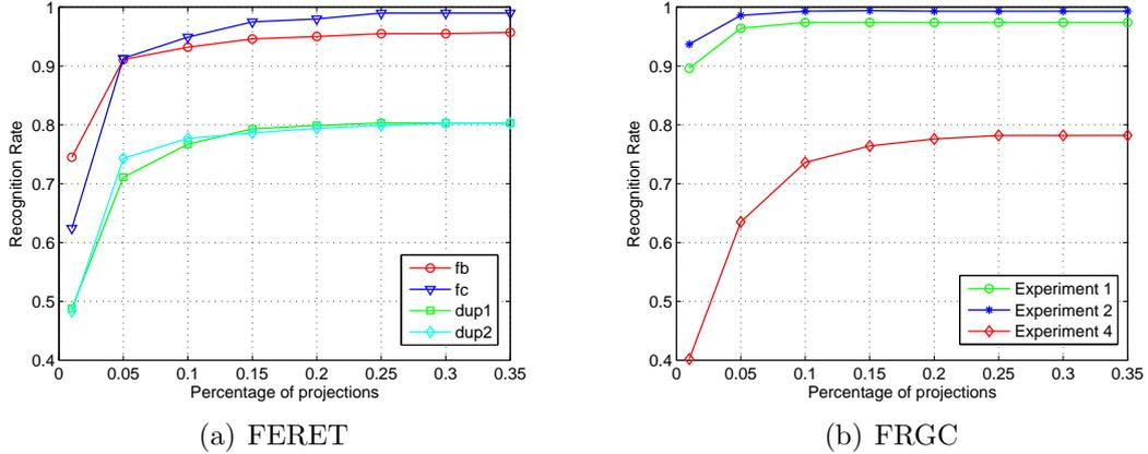
Figure 6.6: Recognition rates as a function of the percentage of projections performed by the tree-based approach when compared to the one-against-all approach.
