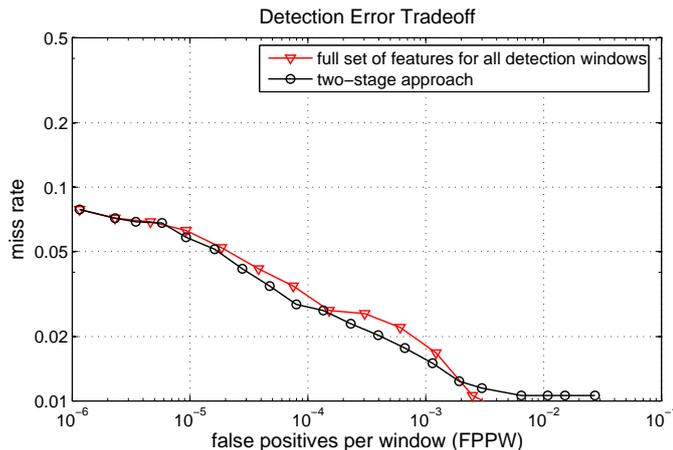
Figure 2.6: Results after adding two stages compared to results obtained without speed optimization.
