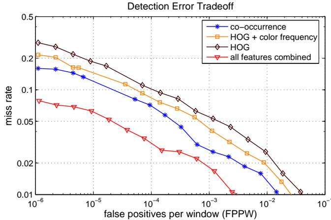
Figure 2.3: Results obtained by using different features and combination of all three feature channels used by this work.
