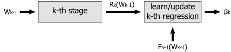
Figure 4.3: Learning a regression model to estimate the generic detector’s responses for the  $k$ ’st stage. Using features extracted from the previous stage,  $k-1$ , and responses obtained by the generic detector at the  $k$ ’th stage, a regression model is learned using  $F_{k-1}(\mathbf{W}_{k-1})$  and  $R_k(\mathbf{W}_{k-1})$  as independent and dependent variables, respectively.
