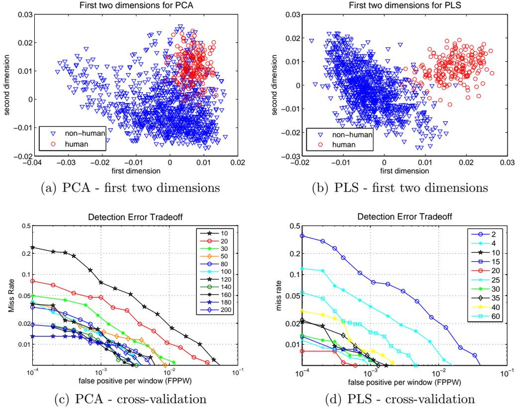
Figure 2.2: Comparison of PCA and PLS for dimensionality reduction. (a-b) projection of the first two dimensions of the training samples for one of the models learned in the cross-validation. (c-d) DET curves according to the number of dimensions used to train the classifier.
