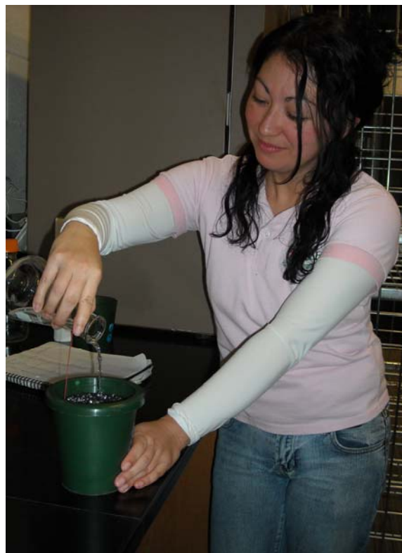
Fig. 2.3. Addition of 250 ml of RO water to Oyama pot containing the treatment of 30% CR and 70% glass beads.
