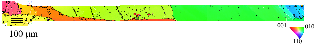
Figure 6-11: OIM Images of as-fabricated TMM joint showing 5 Sn grains across the length of the joint
